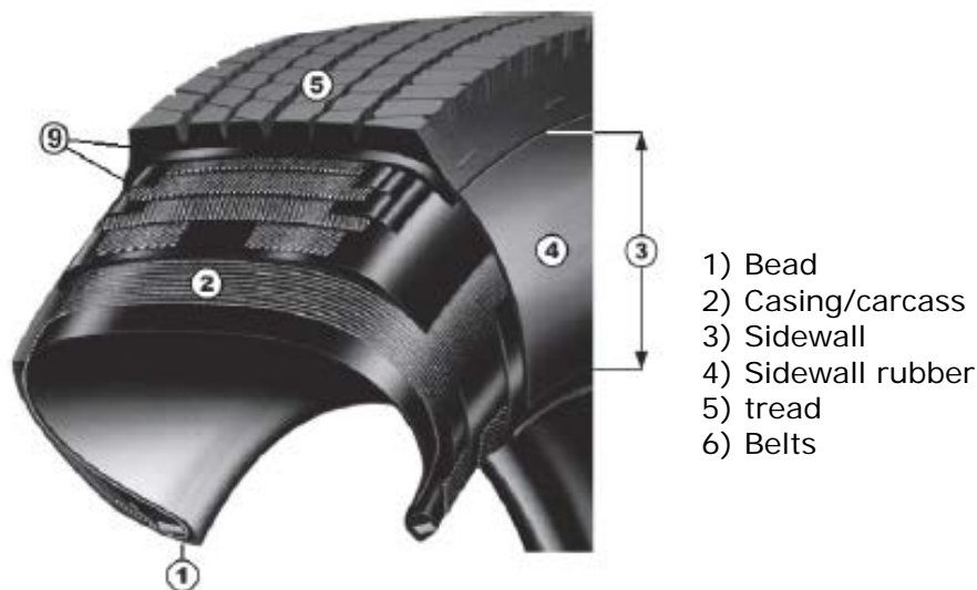
Figure 23: Basic tyre components (figure from ETRMA and ETRTO)
