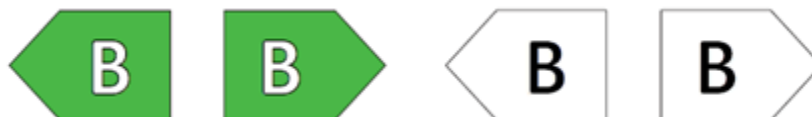
Figure 1: Coloured/monochrome left/right arrow for the part of the packaging facing the prospective customer
