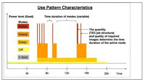
Figure 3: Schematic description of use pattern factors
