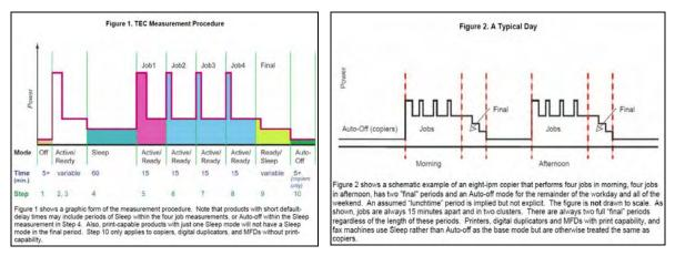
Figure 4: Energy Star TEC Measurement Procedure
