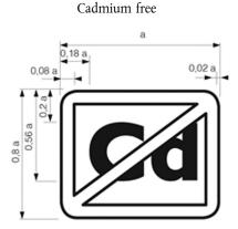
The dimension of 'a' shall be greater than 9 mm and the typeface to be used is 'Gill Sans'.
