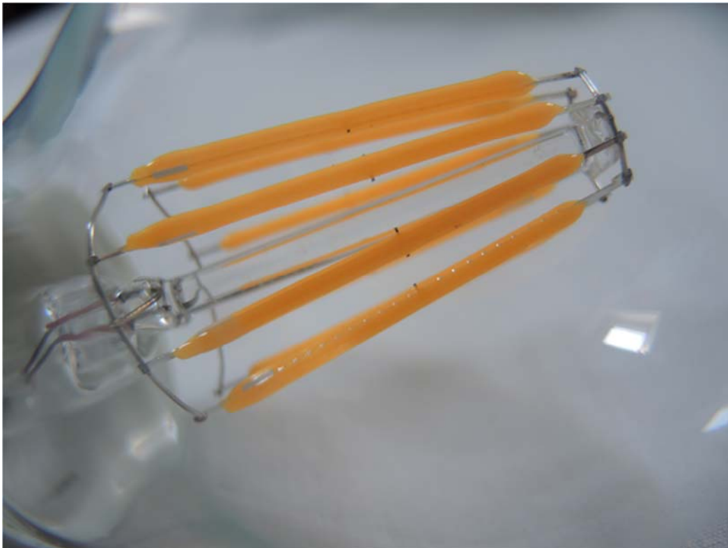
Figure 2-4. Close-up photograph of LED filaments from LED Connection (#5) 8W lamp
