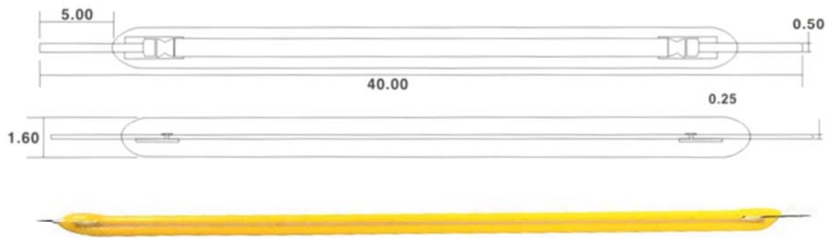
Figure 2-6. Dimensioned (mm) diagram of LED filament and close-up photograph
