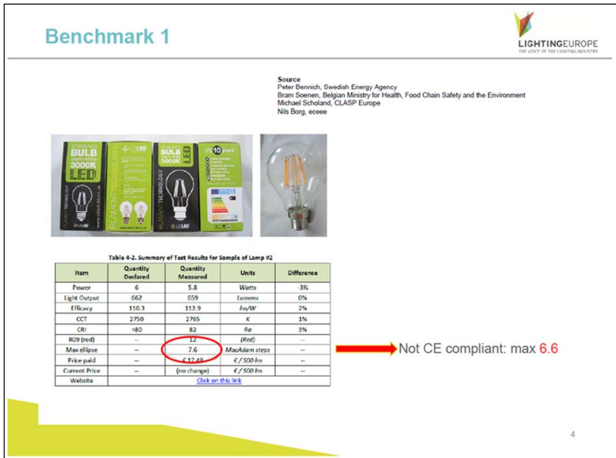
Figure C-1. Lamp #2 exceeds the maximum allowance of MacAdam Steps
