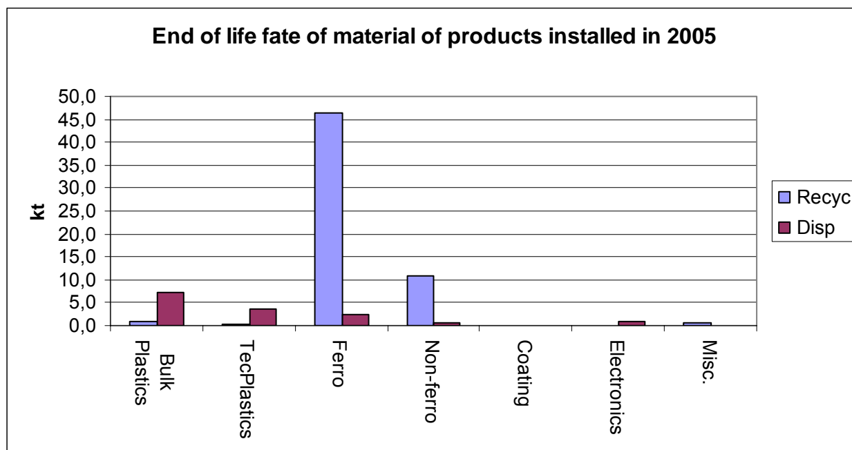
Figure 5-5: End of life fate of material of all residential ventilation products in 2005
