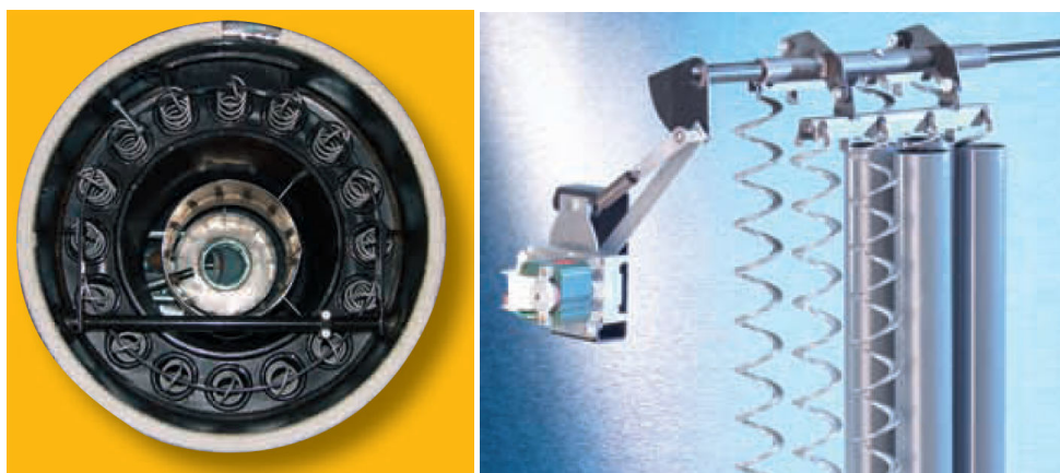
Figure 6-25: Automatic heat exchanger cleaning 34
