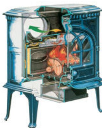
Figure 6-15: A stove with tertiary air supply 20
