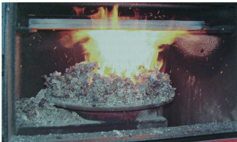
**Figure 3-9: Slagging of retort hearth**
