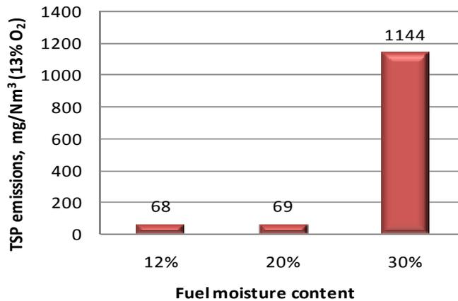
**Figure 3-7: Effect of moisture content in wood (33 cm beech logs) on total dust emissions from a 30 kW chimney stove<sup>34</sup>**
