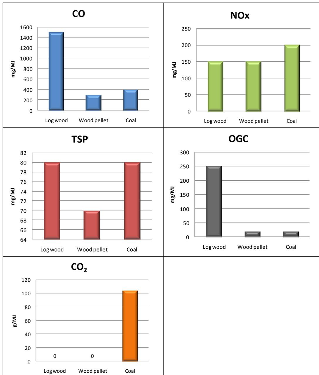
Figure 3-6: Examples of emissions from the combustion of different fuels<sup>12, 30</sup>
