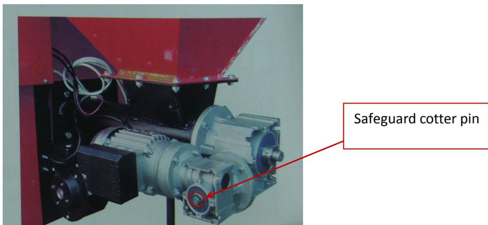
**Figure 3-5: Safeguard cotter pin on the screw conveyor feeding the fuel**
