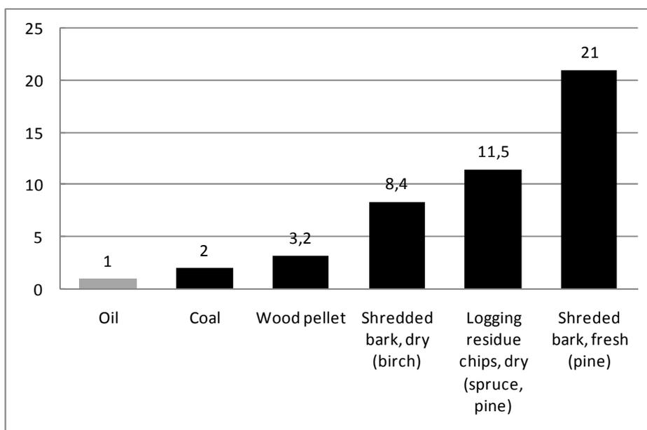
**Figure 3-21: Relative fuel storage space requirement per unit of heat <sup>16</sup>**
