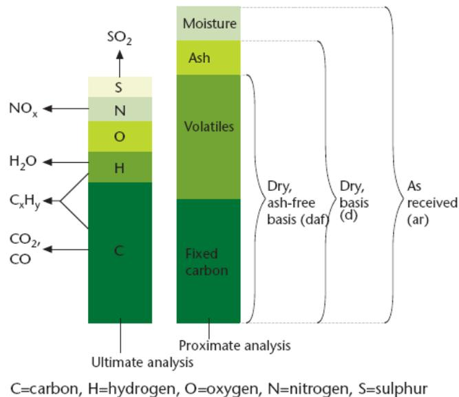
**Figure 3-4: Illustration of how the different levels of fuel analysis and states of fuel (ar, d, daf)<sup>16</sup> relate to each other**
