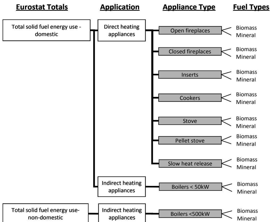
**Figure 3-16: Tree diagram showing the top-down approach used for calculating the solid fuel energy use for each appliance<sup>61</sup> (and eventually for each fuel type)**
