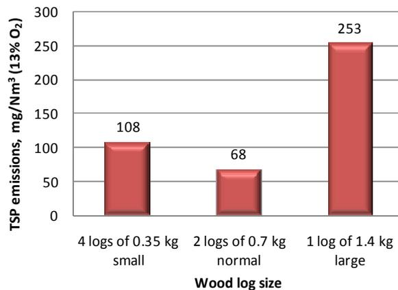
**Figure 3-8: Effect of wood (beech) log size on total dust emissions from a 7 kW chimney stove<sup>36</sup>**
