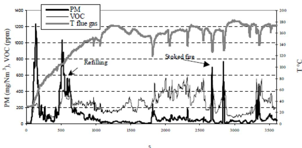
**Figure 3-14: Variations of emissions over time after loading a closed fire place with beech wood<sup>50</sup>**
