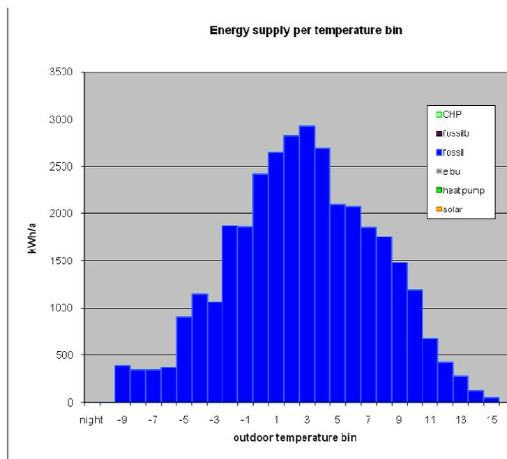
**Figure 3-17: Example calculation for estimating energy consumption in Lot 1 boilers**
