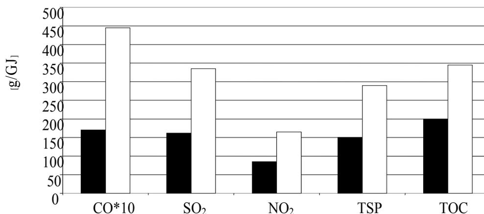
**Figure 3-12: Emissions from a manually fuelled fixed bed coal boiler of 30 kW<sup>44</sup> under natural draught (in white) and under forced draught (in black)<sup>45</sup>**
