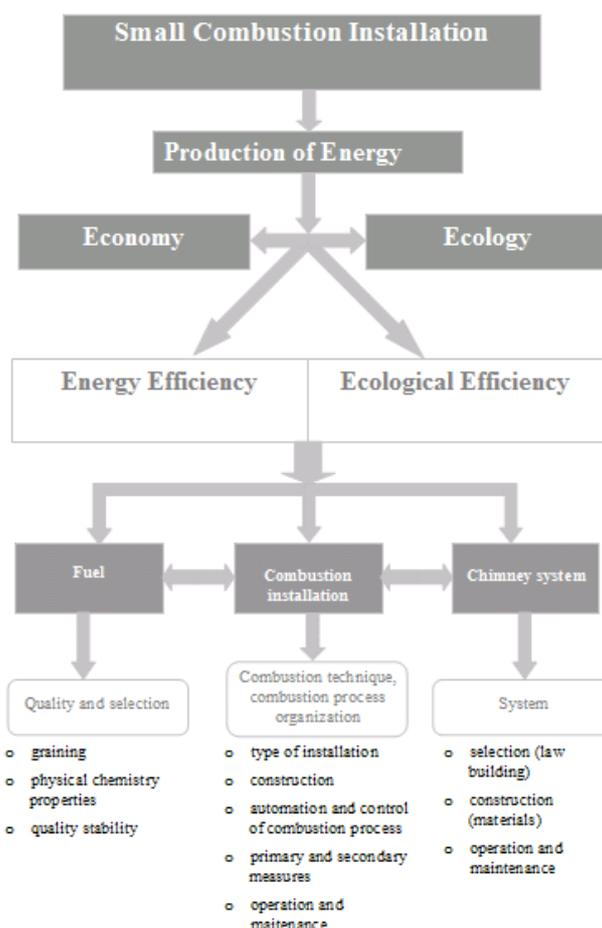
**Figure 3-3: Parameters affecting the environmental impact of solid fuel SCIs<sup>12</sup>**
