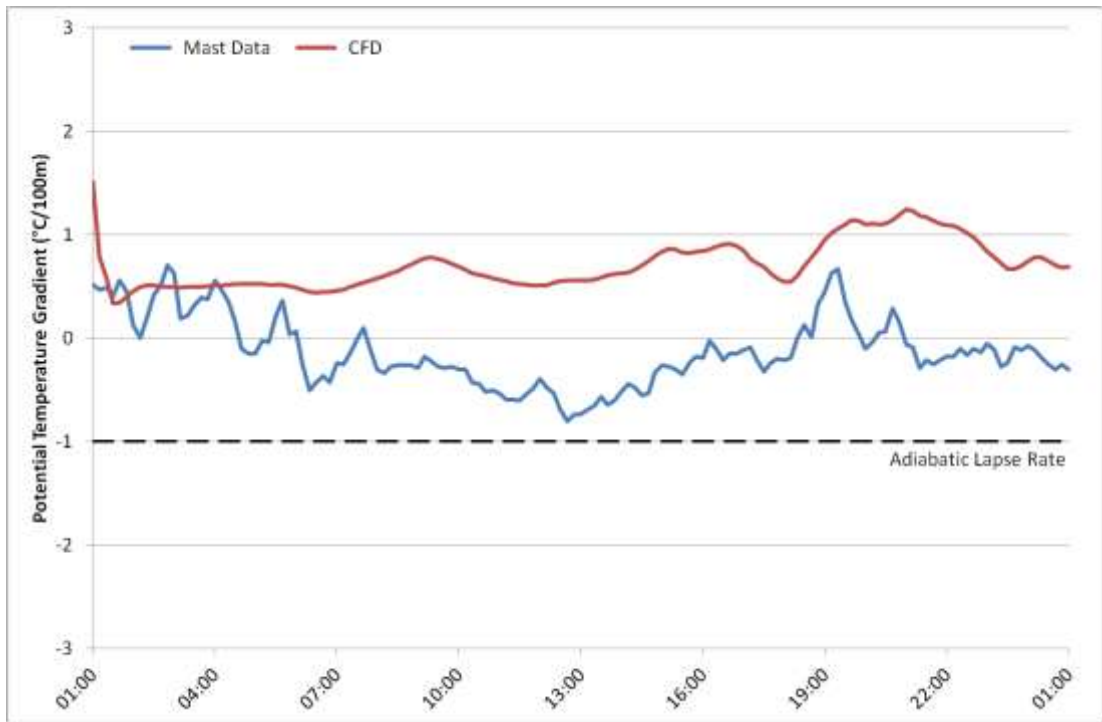
Figure 7N.3: Potential temperature gradient time-series for 16 th January 2011 at M6261, taken between 90m and 10m AGL. Comparison between measured data and CFD.
