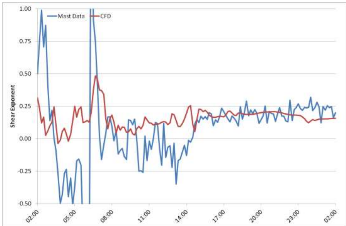
Figure 7T.10: Shear exponent time-series for 27 th May 2011 at M6282, taken between 73m and 50m AGL. Comparison between measured data and CFD.
