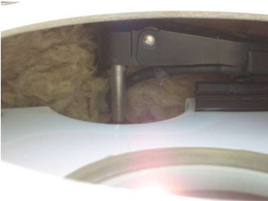
Figure 7.3.4: Insulation in the LiDAR device.
