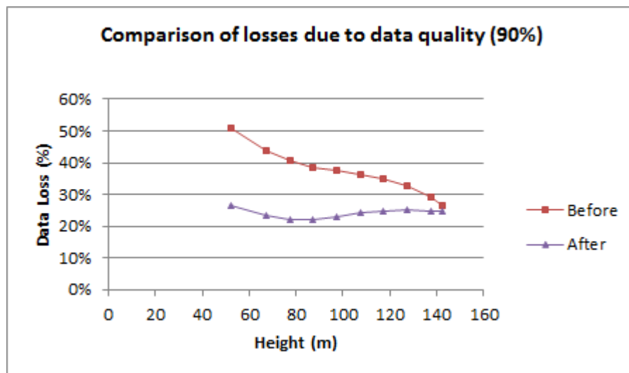
Figure 7.2.2: Comparison of losses due to data quality before and after wiper replacement
