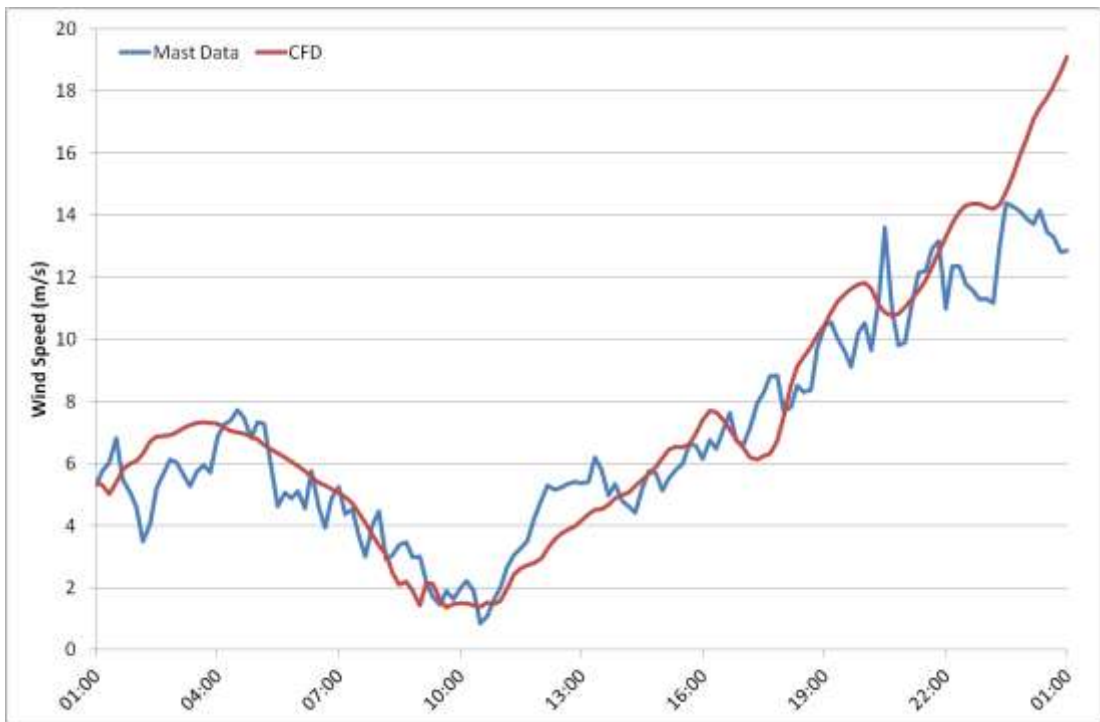
Figure 7L.1: Wind speed time-series for 27 th November 2012 at M6261, 87m AGL. Comparison between measured data and CFD.
