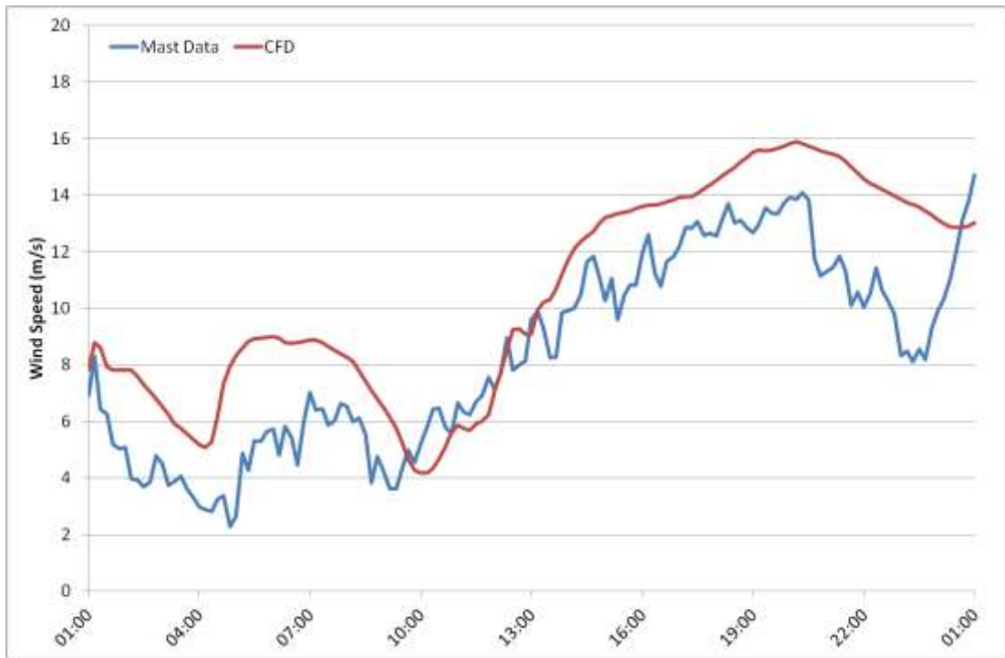
Figure 7P.1: Wind speed time-series for 20 th February 2012 at M6261, 87m AGL. Comparison between measured data and CFD.
