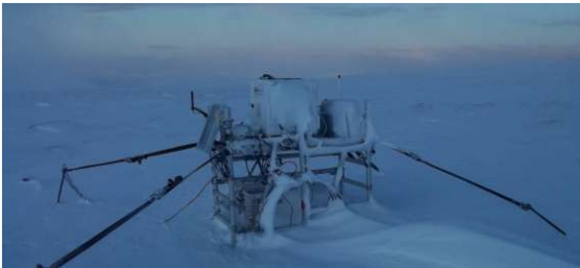
Figure 7.3.2: Leosphere WINDCUBE V2 on a scaffold snow platform in Scotland.
