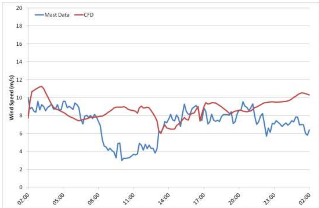
Figure 7Q.6: Wind speed time-series for 6 th April 2012 at M6282, 87m AGL. Comparison between measured data and CFD.
