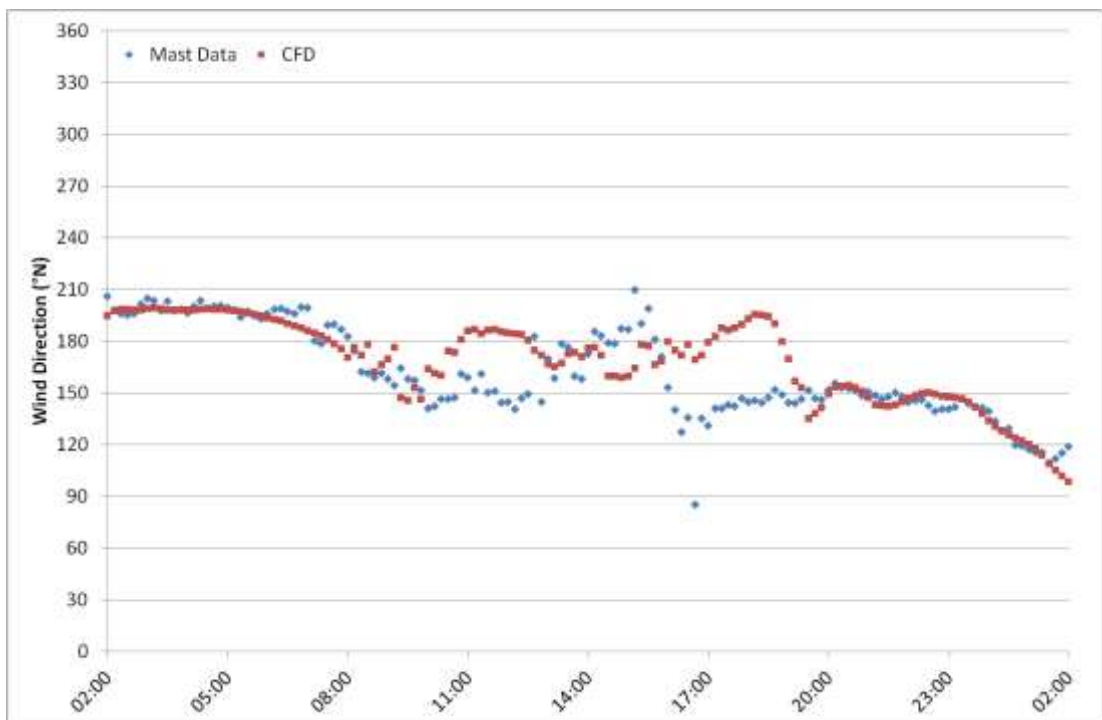
Figure 7S.2: Wind direction time-series for 16 th May 2012 at M6261, 85m AGL. Comparison between measured data and CFD.
