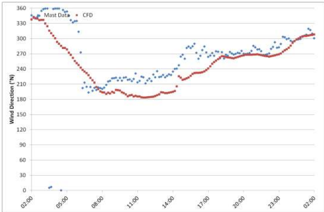
Figure 7T.7: Wind direction time-series for 27 th May 2012 at M6282, 85m AGL. Comparison between measured data and CFD.
