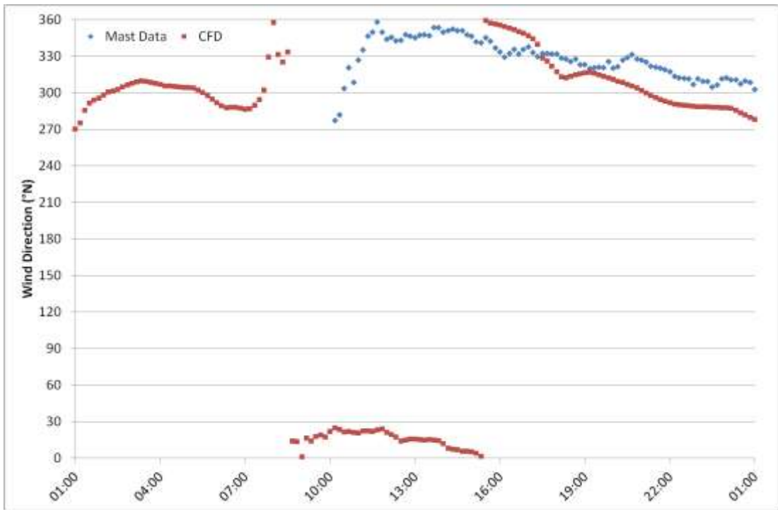
Figure 7L.7: Wind direction time-series for 27 th November 2012 at M6282, 85m AGL. Comparison between measured data and CFD.
