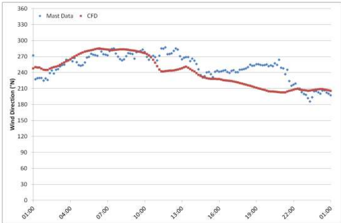
Figure 70.7: Wind direction time-series for 17 th February 2012 at M6282, 85m AGL. Comparison between measured data and CFD.
