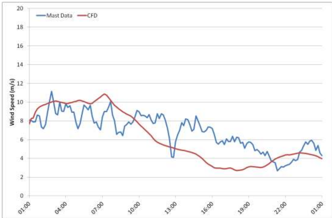
Figure 7N.1: Wind speed time-series for 16 th January 2012 at M6261, 87m AGL. Comparison between measured data and CFD.
