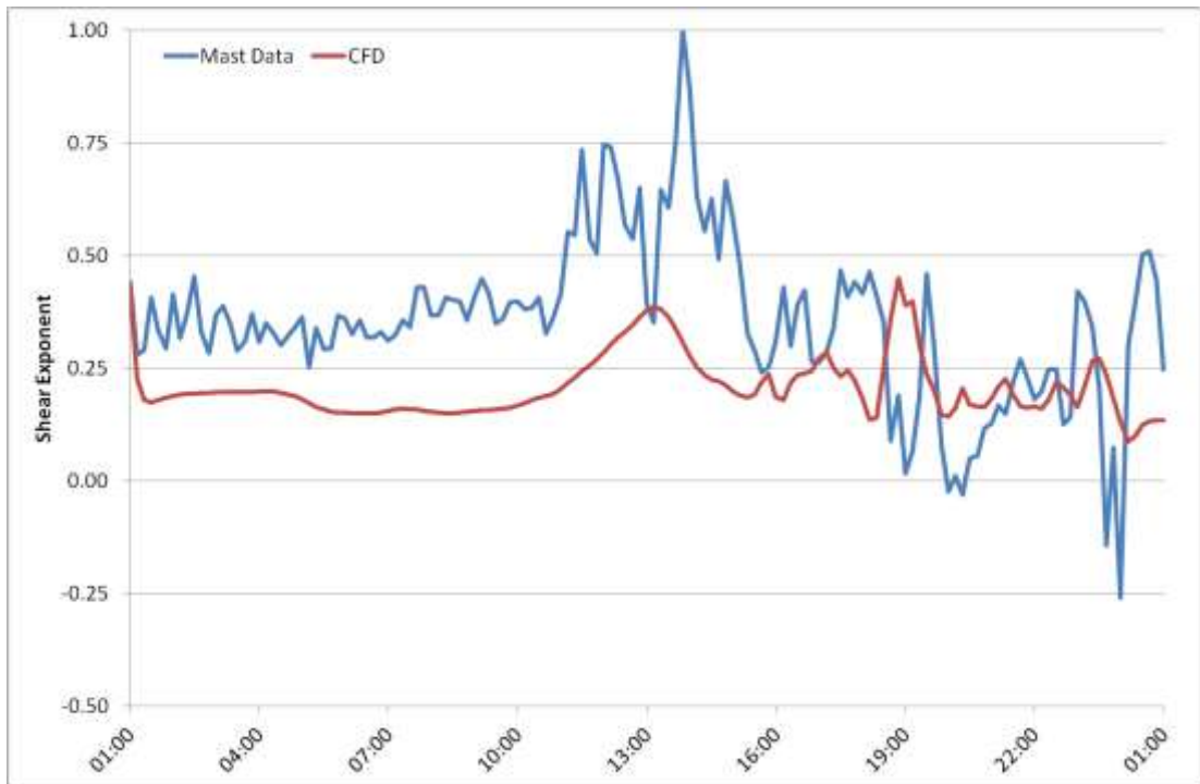
Figure 7M.10: Shear exponent time-series for 31 st December 2011 at M6282, taken between 73m and 50m AGL. Comparison between measured data and CFD.
