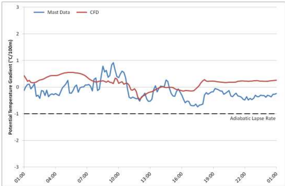
Figure 7L.3: Potential temperature gradient time-series for 27 th November 2011 at M6261, taken between 90m and 10m AGL. Comparison between measured data and CFD.
