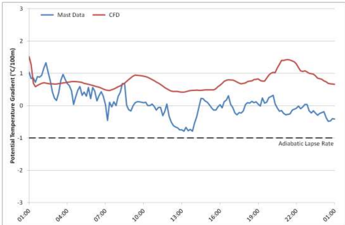
Figure 7N.8: Potential temperature gradient time-series for 16 th January 2011 at M6282, taken between 90m and 10m AGL. Comparison between measured data and CFD.
