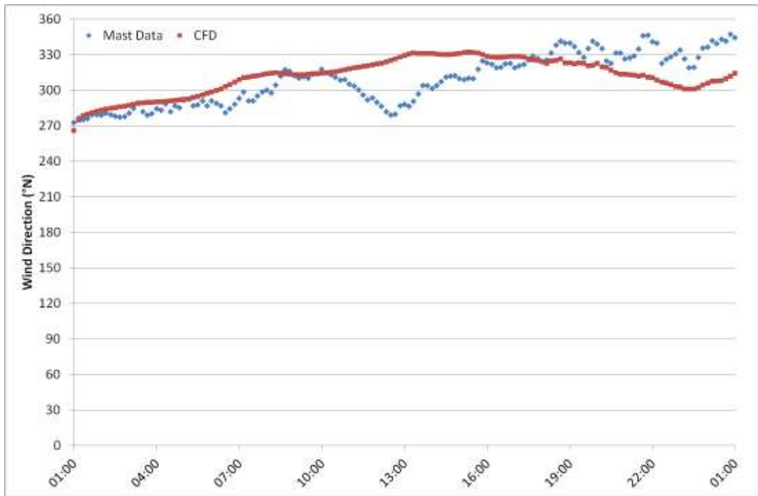
Figure 7N.7: Wind direction time-series for 16 th January 2012 at M6282, 85m AGL. Comparison between measured data and CFD.
