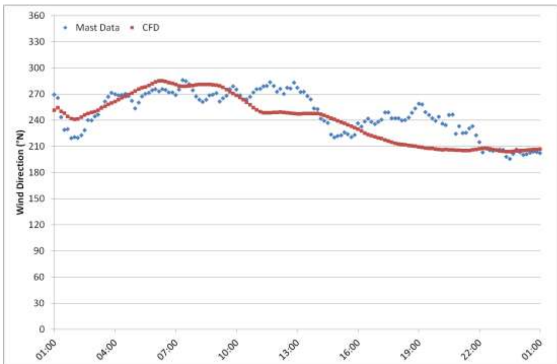
Figure 70.2: Wind direction time-series for 17 th February 2012 at M6261, 85m AGL. Comparison between measured data and CFD.
