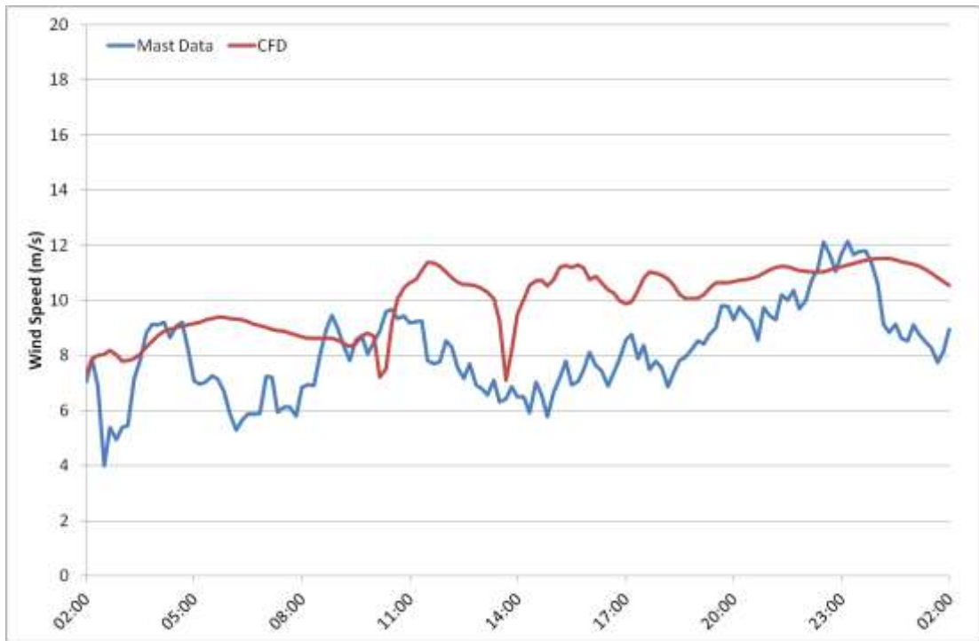
Figure 7R.1: Wind speed time-series for 19 th April 2012 at M6261, 87m AGL. Comparison between measured data and CFD.
