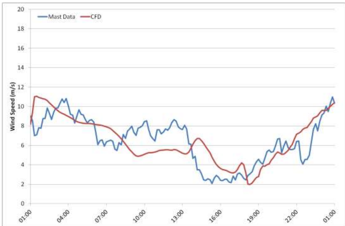
Figure 7M.1: Wind speed time-series for 31 st December 2012 at M6261, 87m AGL. Comparison between measured data and CFD.
