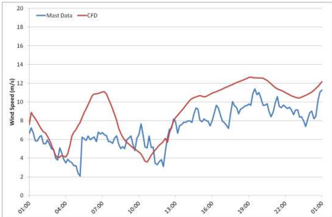
Figure 7P.6: Wind speed time-series for 20 th February 2012 at M6282, 87m AGL. Comparison between measured data and CFD.
