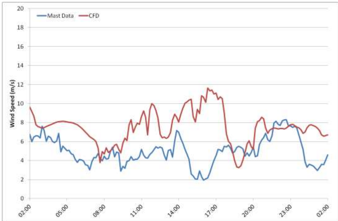
Figure 7S.1: Wind speed time-series for 16 th May 2012 at M6261, 87m AGL. Comparison between measured data and CFD.
