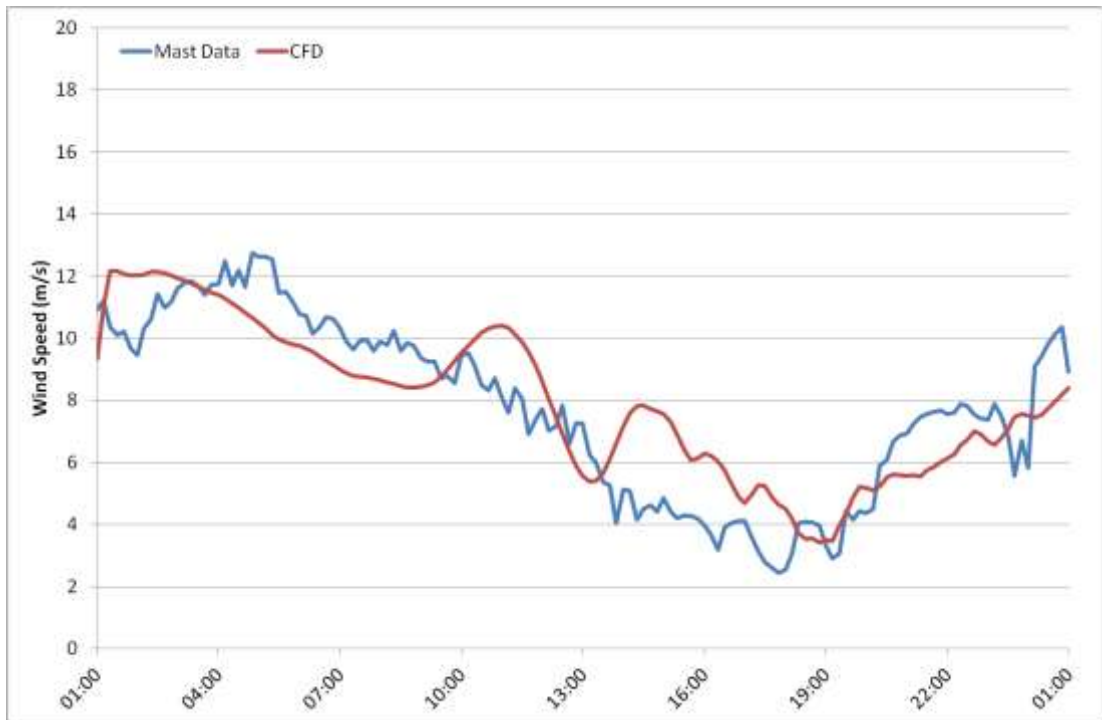
Figure 7M.6: Wind speed time-series for 31 st December 2012 at M6282, 87m AGL. Comparison between measured data and CFD.
