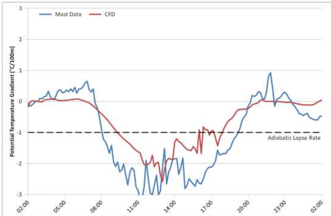
Figure 7.7.31: Temperature gradient time-series for 6 th April 2012 at M6261, taken between 90m and 10m AGL. Comparison between measured data and CFD.
