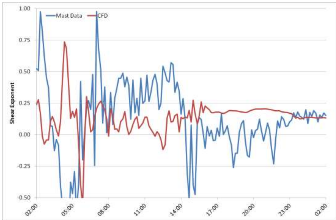
Figure 7T.5: Shear exponent time-series for 27 th May 2011 at M6261, taken between 73m and 50m AGL. Comparison between measured data and CFD.
