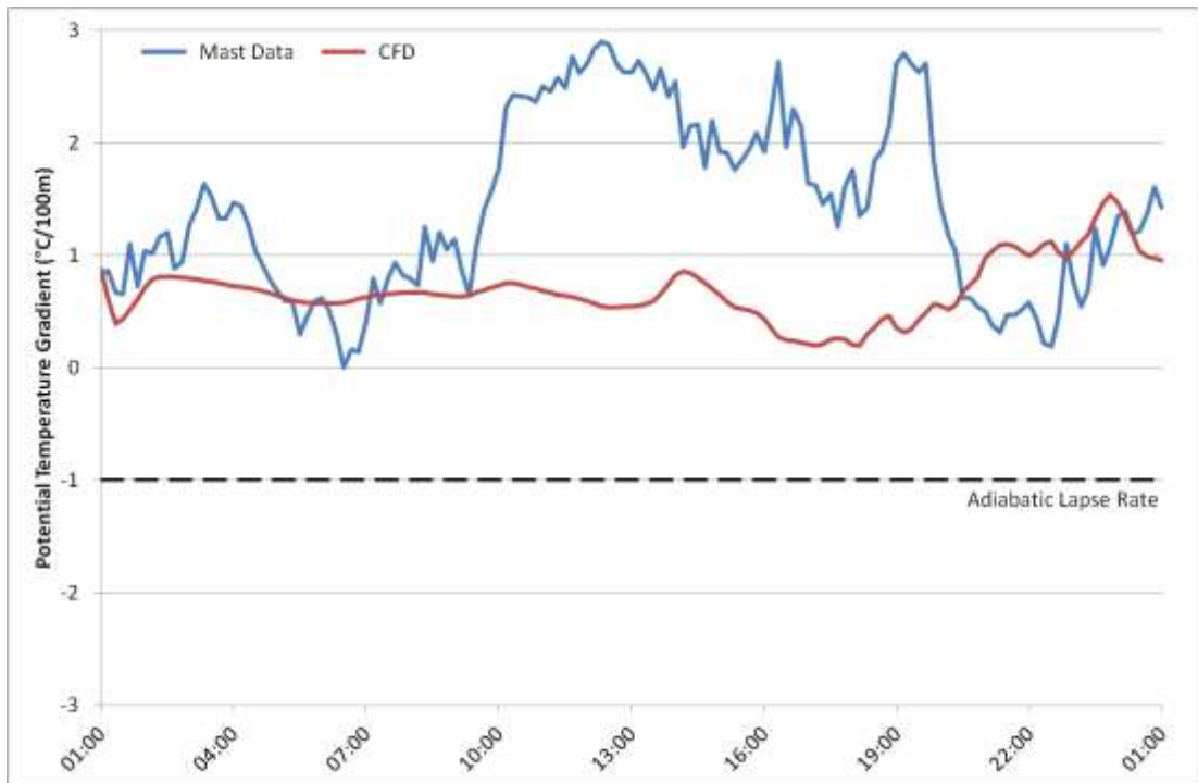
Figure 7M.3: Potential temperature gradient time-series for 31 st December 2011 at M6261, taken between 90m and 10m AGL. Comparison between measured data and CFD.
