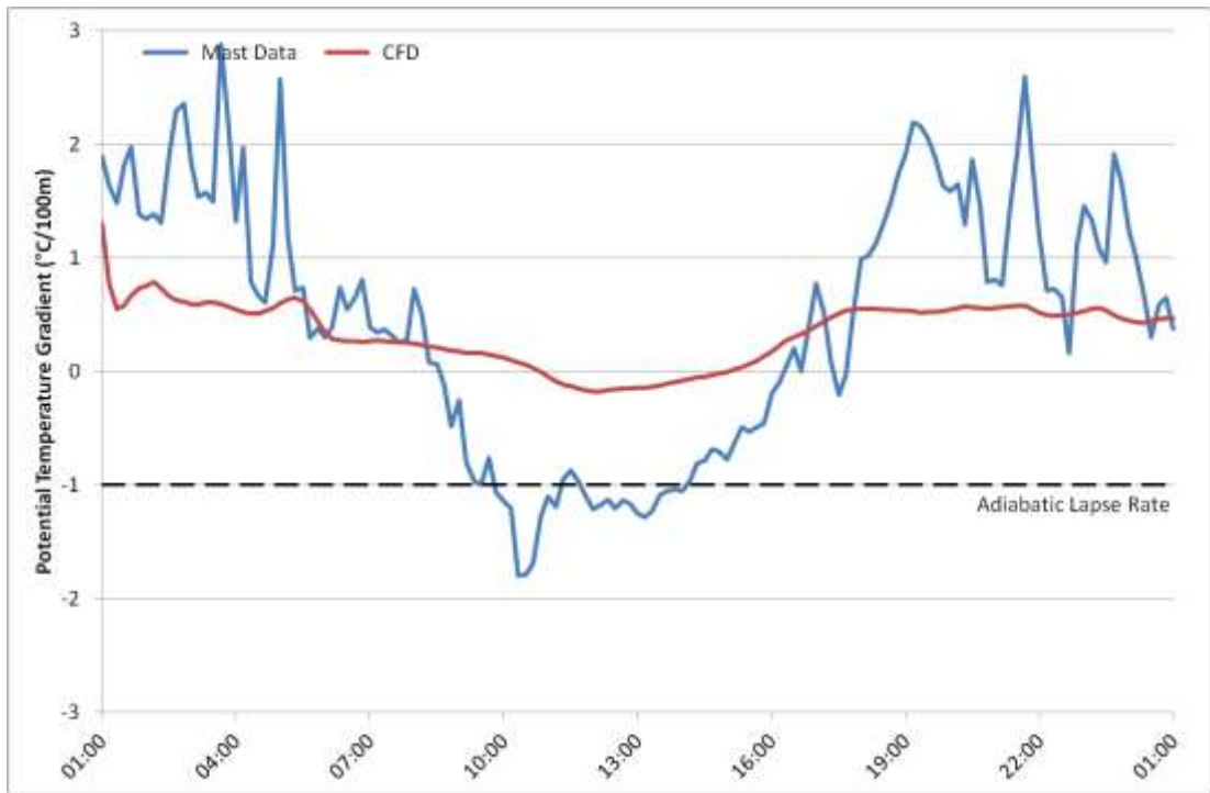
Figure 70.3: Potential temperature gradient time-series for 17 th February 2011 at M6261, taken between 90m and 10m AGL. Comparison between measured data and CFD.
