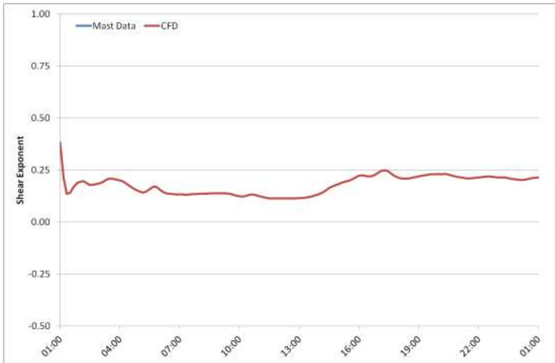
Figure 70.5: Shear exponent time-series for 17 th February 2011 at M6261, taken between 73m and 50m AGL. CFD only, no measured data available for comparison.
