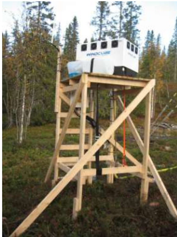
Figure 7.3.1: Leosphere WINDCUBE V1 on snow/hunting platform at Havsnäs
