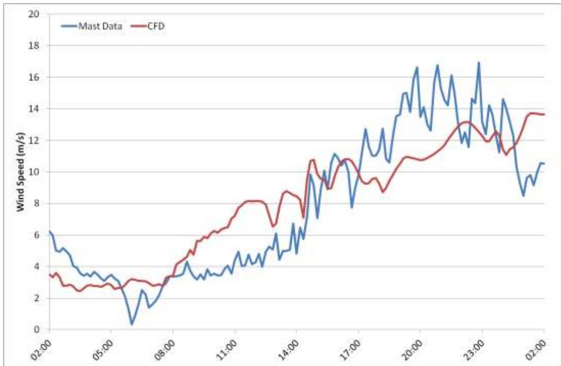
Figure 7T.6: Wind speed time-series for 27 th May 2012 at M6282, 87m AGL. Comparison between measured data and CFD.
