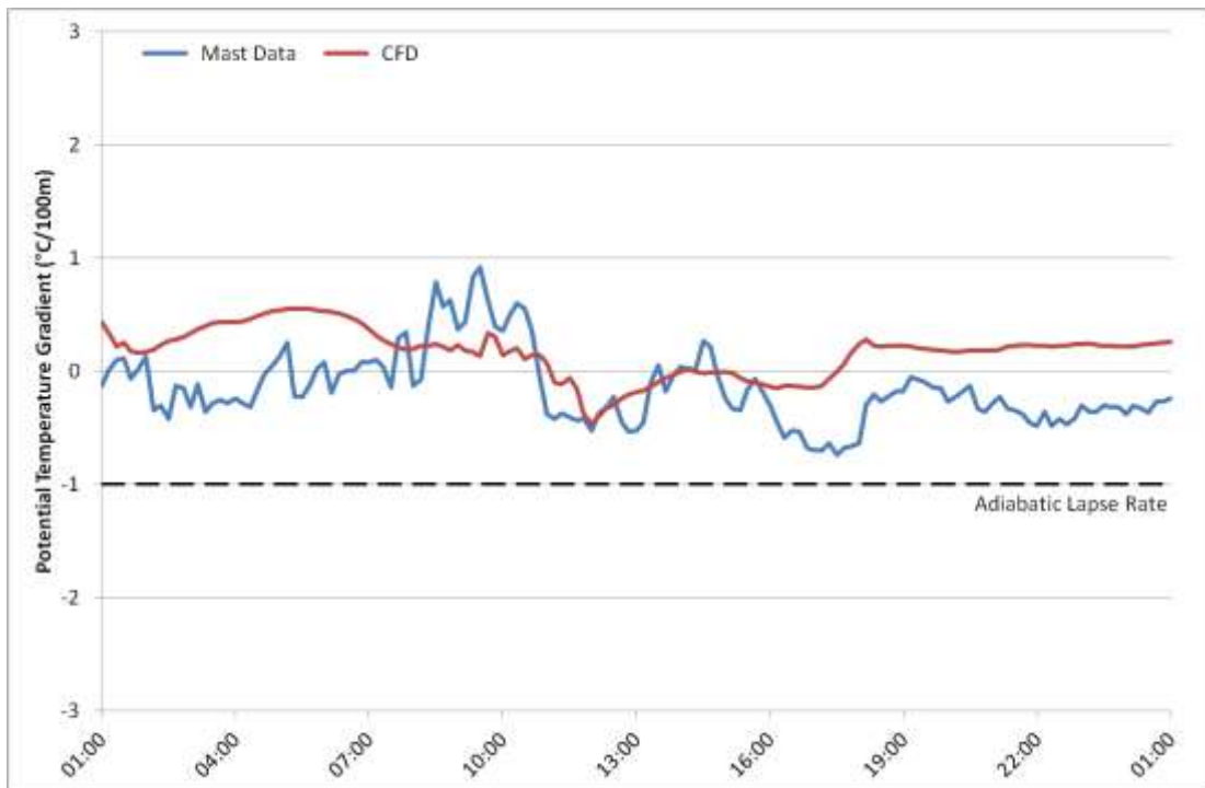
Figure 7.7.30: Temperature gradient time-series for 27 th November 2011 at M6261, taken between 90m and 10m AGL. Comparison between measured data and CFD.
