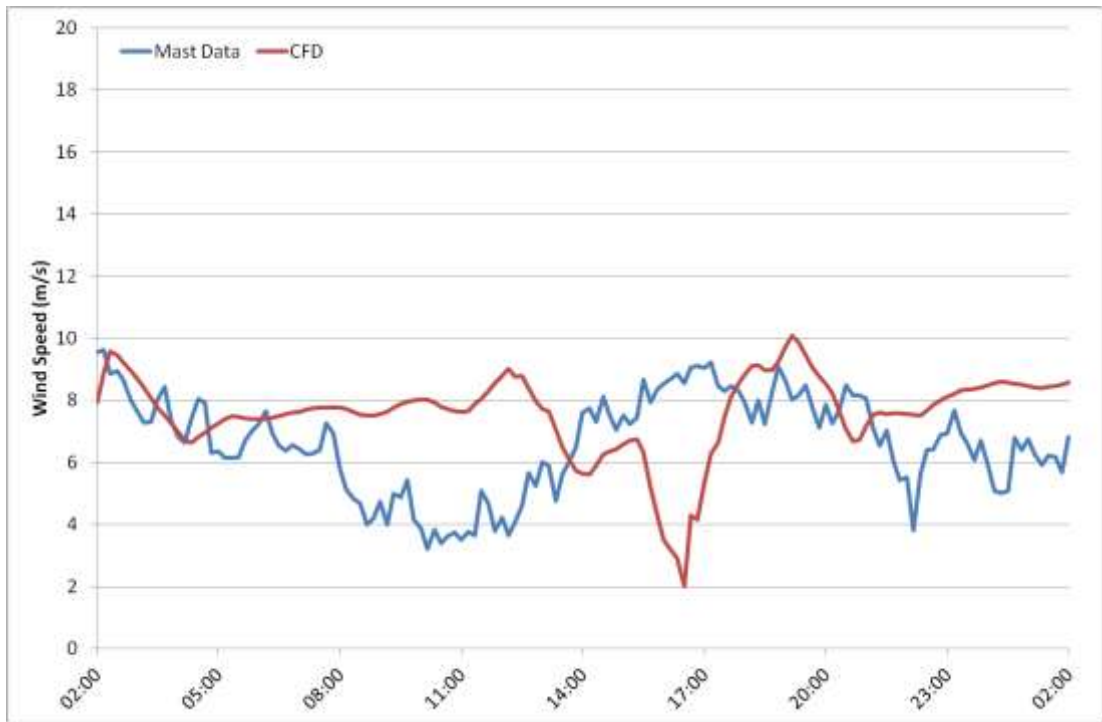
Figure 7Q.1: Wind speed time-series for 6 th April 2012 at M6261, 87m AGL. Comparison between measured data and CFD.
