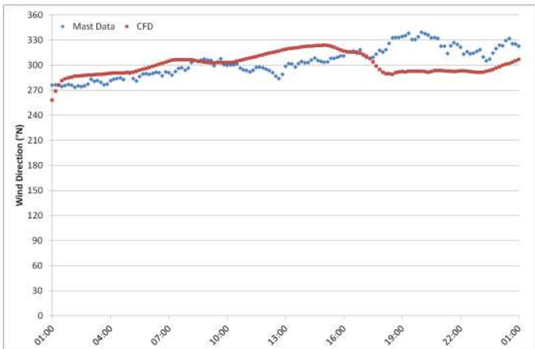
Figure 7N.2: Wind direction time-series for 16 th January 2012 at M6261, 85m AGL. Comparison between measured data and CFD.
