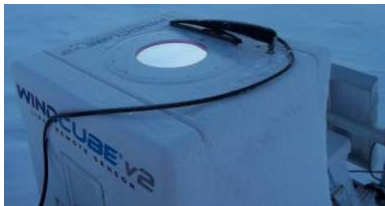
Figure 7.3.5: Clear window on Leosphere WINDCUBE V2.
