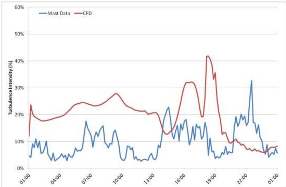
Figure 7M.4: Turbulence intensity time-series for 31 st December 2012 at M6261, 87m AGL. Comparison between measured data and CFD.
