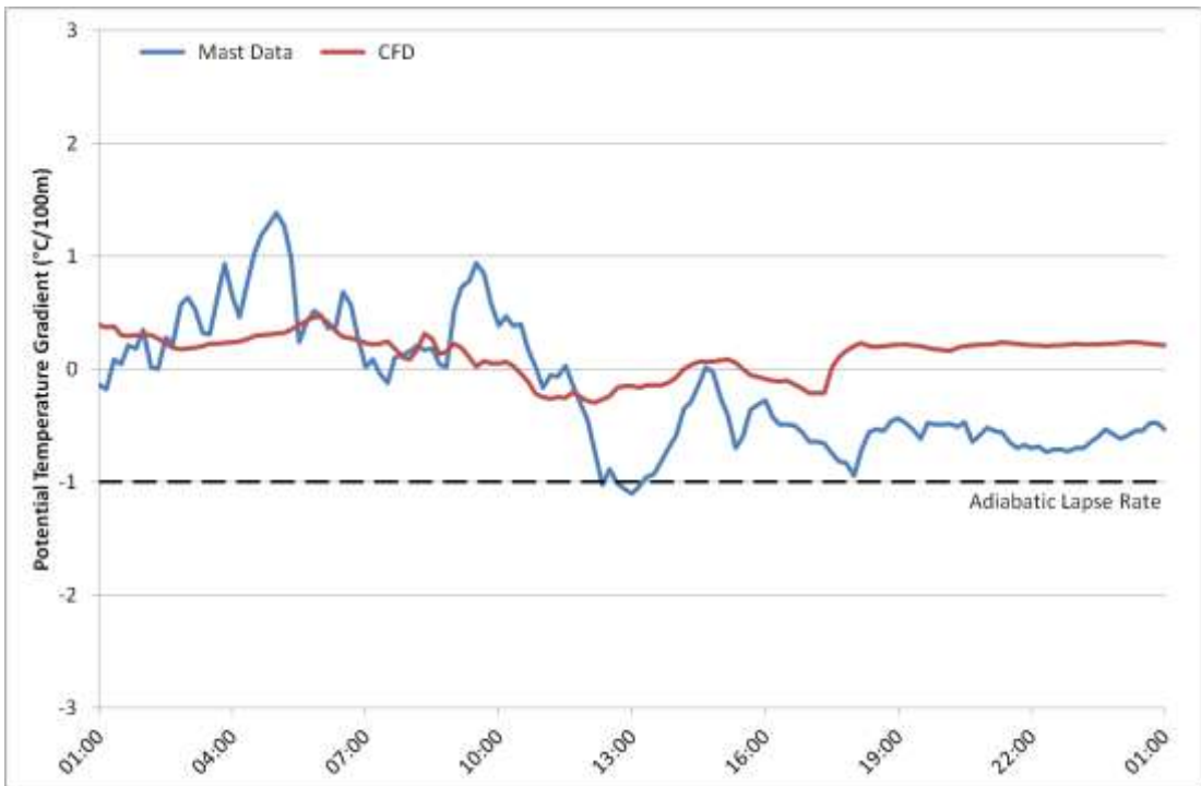
Figure 7L.8: Potential temperature gradient time-series for 27 th November 2011 at M6282, taken between 90m and 10m AGL. Comparison between measured data and CFD.
