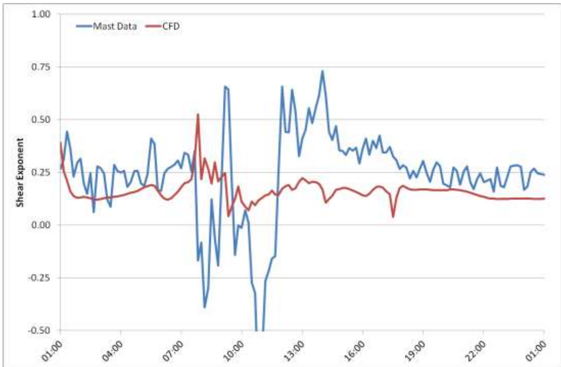
Figure 7L.10: Shear exponent time-series for 27 th November 2011 at M6282, taken between 73m and 50m AGL. Comparison between measured data and CFD.
