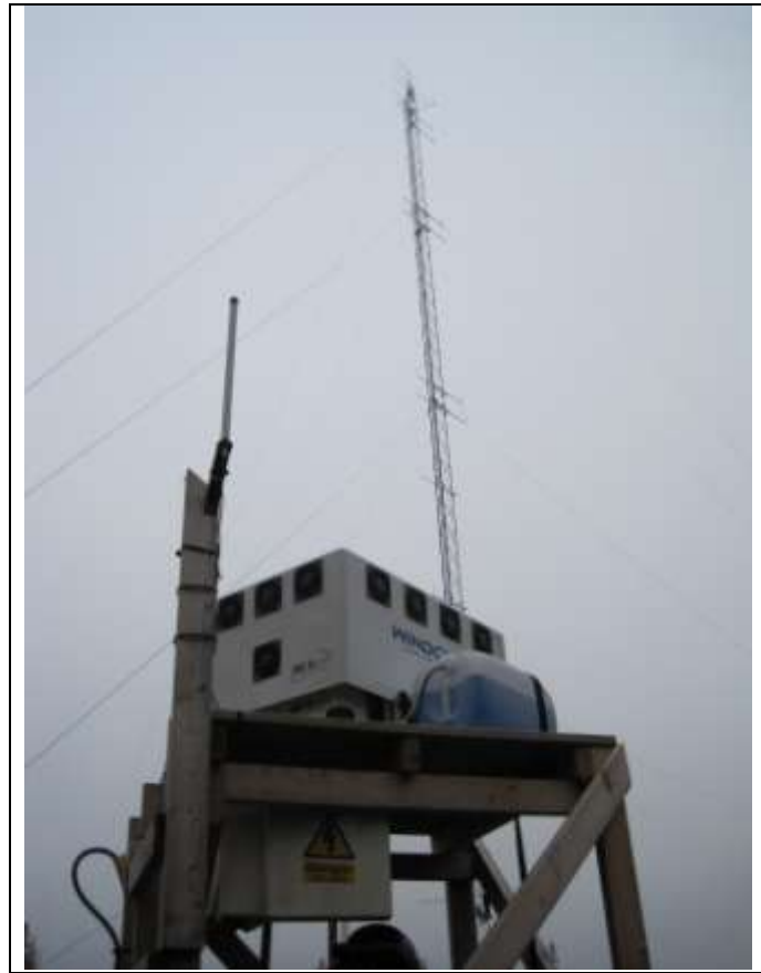
Figure 7.6.1: Windcube LiDAR and Reference Mast M626.
