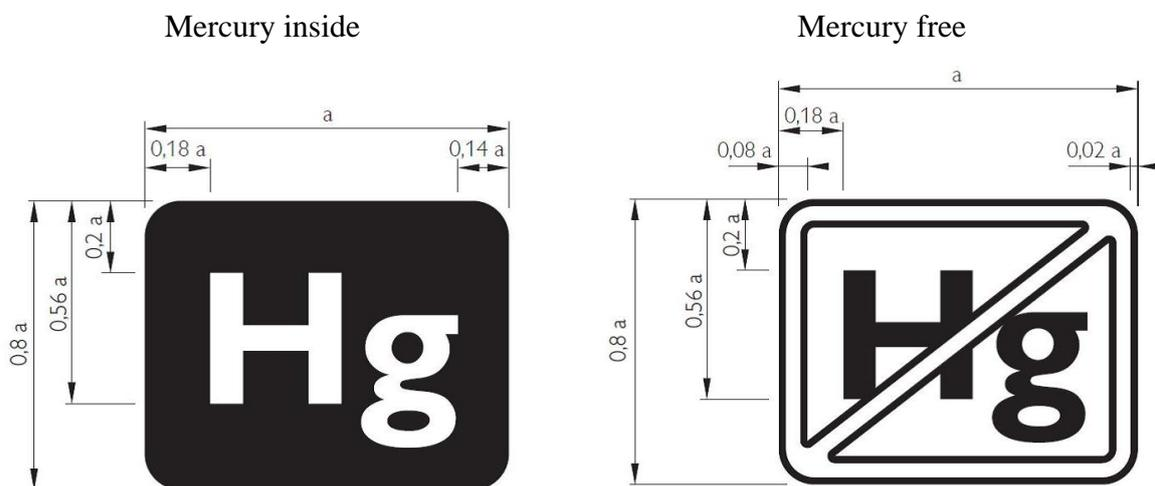
The “Mercury inside” logo shall be firmly attached also internally on the display panel in a position clearly visible by workers once the external cover bearing the external logo is removed.
