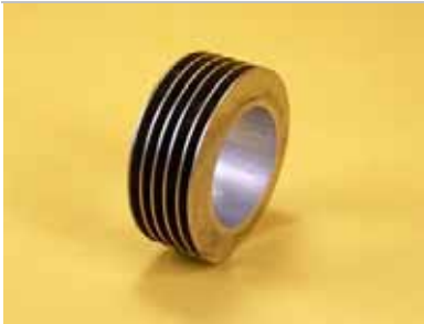
Figure 5-14. Solid fin, in the form of a metal strip: The fin is helically wound around the specified pipe/tube and continuously fillet welded to the tube using the M.I.G. weld process (source: Tex-Fin, USA).
