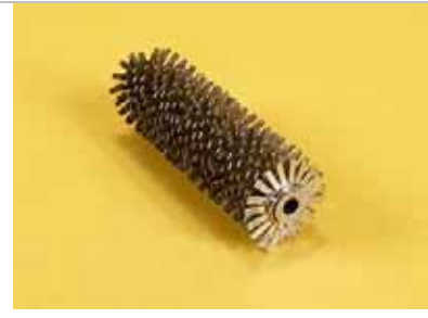
Figure 5-16. Serrated Fin: A metal strip that has been serrated or cut and then helically wound around the specified tube. The fin is welded to the tubular base using a high frequency weld process (source: Tex-Fin, USA).
