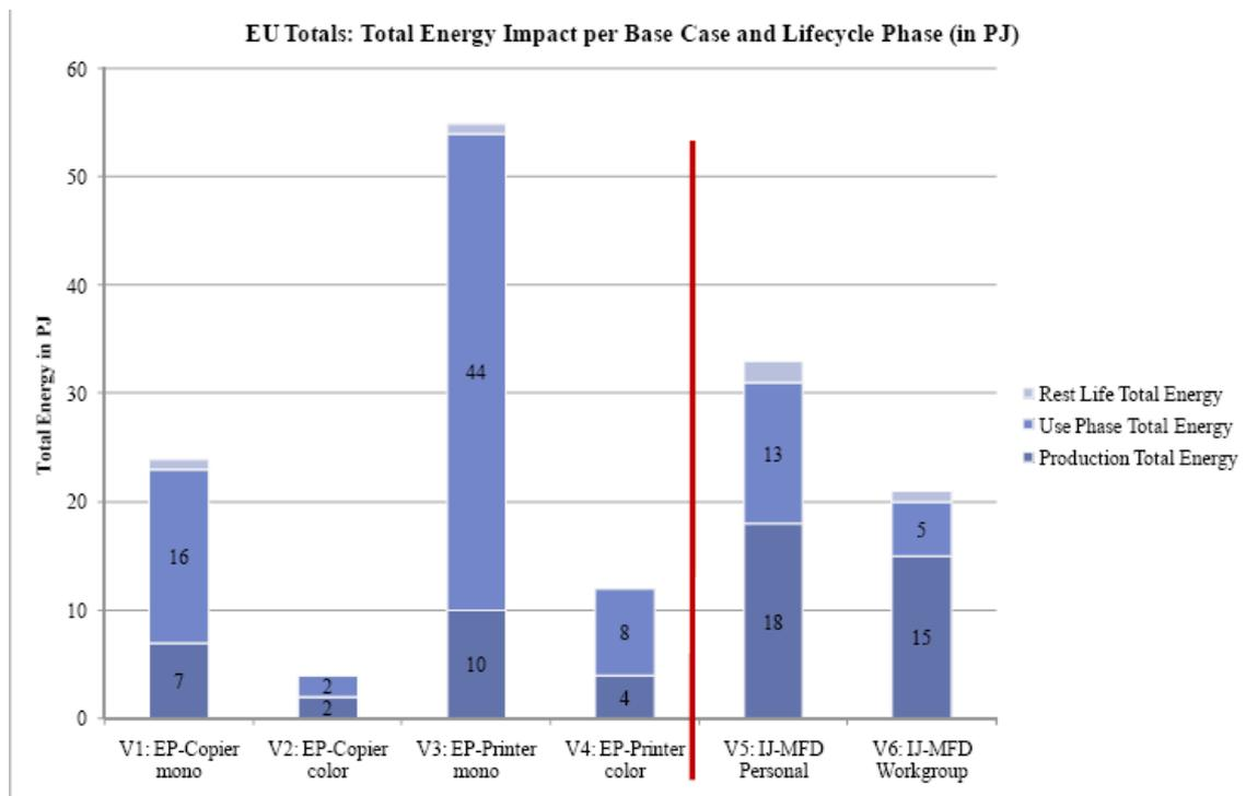
**Figure 2: Total energy impact of life cycle phases according to the base cases (excl. paper consumption)**
