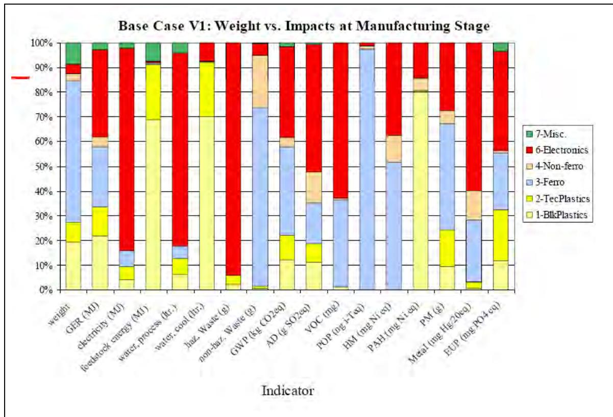
**Figure 3: Manufacturing phase impact assessment of EP-Copier monochrome (base case V1)**
