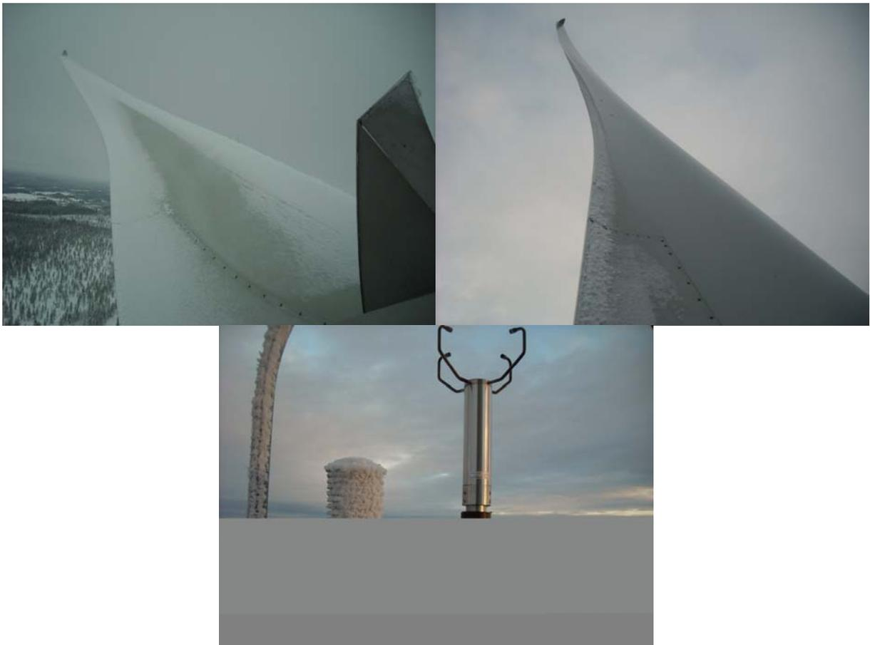
**Figure 5: test site Dragaliden on 2008-01-01; upper photos: with unheated blade at WEC 1 (left) and heated blade at WEC 2 (right), photo below: heated nacelle anemometer at WEC 2**
