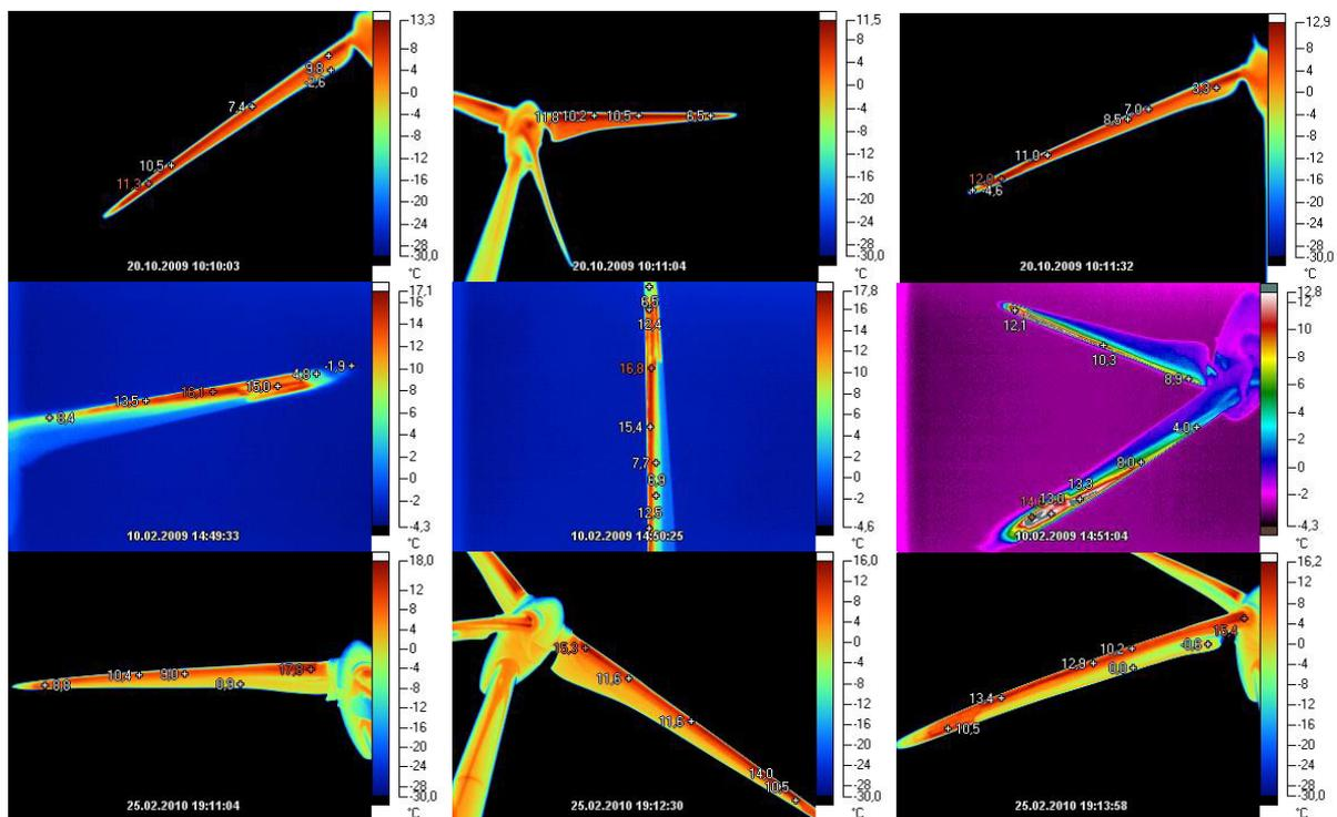
**Figure 4: infrared heat images of heated rotor blades;**
