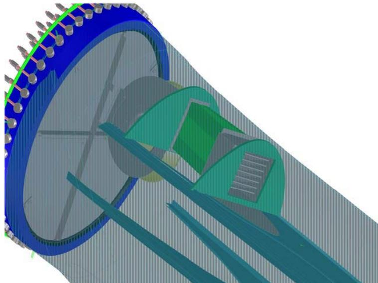
**Figure 2: Fan heater integrated into the rotor blade**
