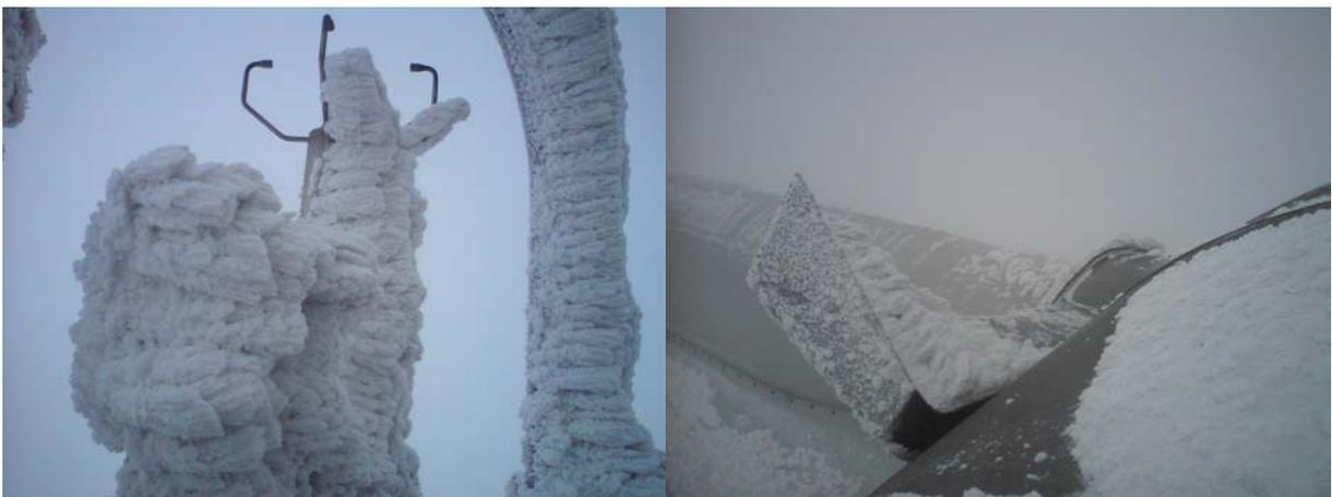
**Figure 6: example of extreme icing conditions at the wind farm Krystofovy-Hamry, left: nacelle anemometer and air temperature sensor of a test WEC on 2010-01-14 14:45, right: heated rotor blade of a test WEC at the wind farm Krystofovy-Hamry on 2010-01-15 12:26**
