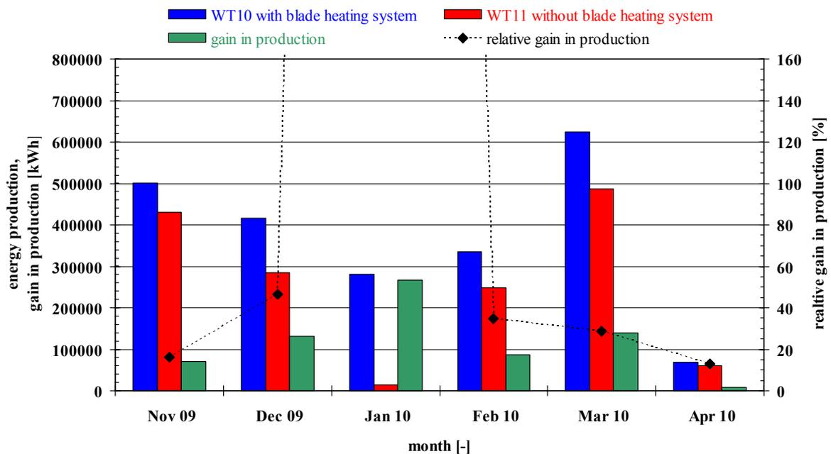
**Figure 8: Comparison of energy metering data of the WEC with and without the rotor blade de-icing system at the site Krystofovy-Hamry, Czech Republic**
