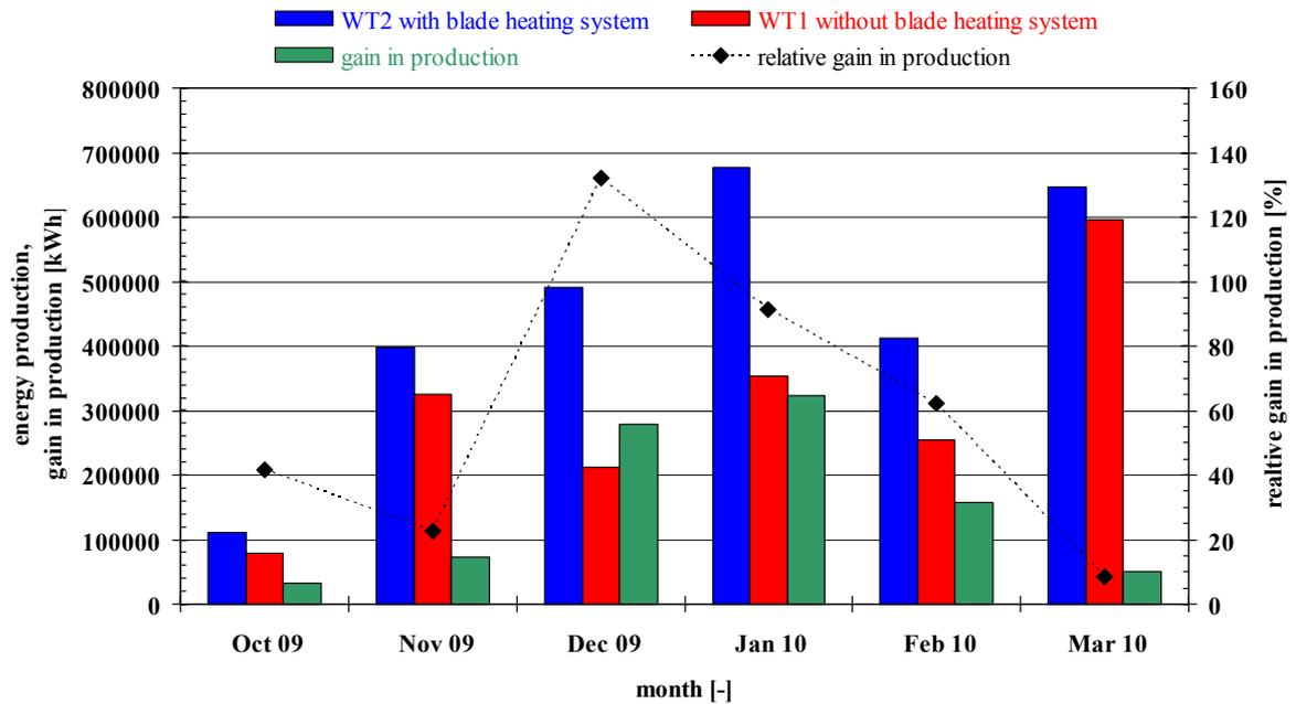
**Figure 7: Comparison of the energy metering data of the WECs with and without the rotor blade de-icing system in Dragaliden, Sweden. In the period 2009-11-09 to 2009-11-22 the energy production of WEC 2 has been replaced by the energy production of WEC 1 as in this period the blade de-icing system of WEC 2 was switched off and the blade de-icing system of WEC 1 was switched on.**
