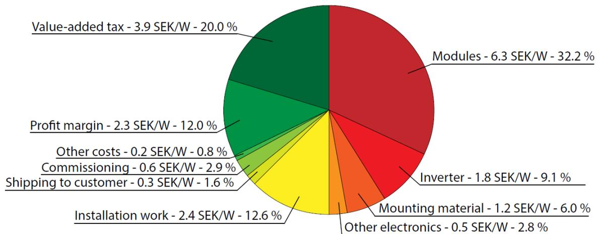
**Figure 10: Average of 15 Swedish installation companies cost structures for a typical turnkey grid-connected roof-mounted residential PV system (4–6 kW<sub>p</sub>) to the end customer in the end of 2015.**
