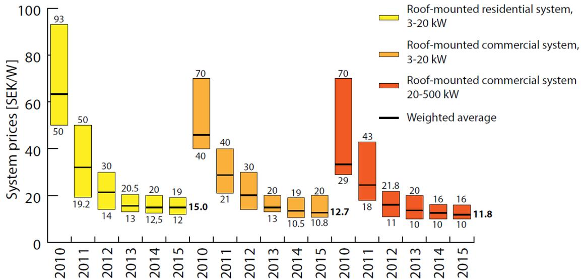
**Figure 9: The price difference for typical turnkey PV systems between different Swedish installation companies (excluding VAT). Note that this is the prices that the companies regard as typical for their company, and that the graph therefore does not show the absolute highest and lowest prices in Sweden.**
