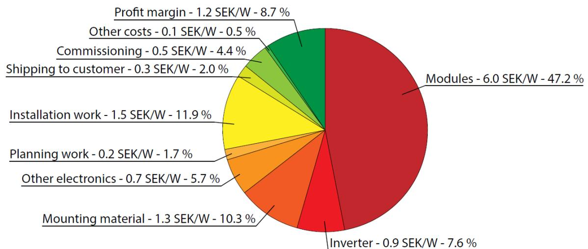
**Figure 11: Average of 5 Swedish installation companies cost structures for a typical turnkey grid-connected roof-mounted commercial PV system (40–60 kW<sub>p</sub>) to the end customer in the end of 2015.**
