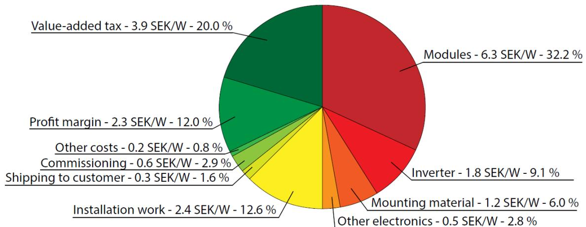
**Figure 10: Average of 15 Swedish installation companies cost structures for a typical turnkey grid-connected roof-mounted residential PV system (4–6 kW<sub>p</sub>) to the end customer in the end of 2015. The average price was 19.45 SEK/W<sub>p</sub>.**
