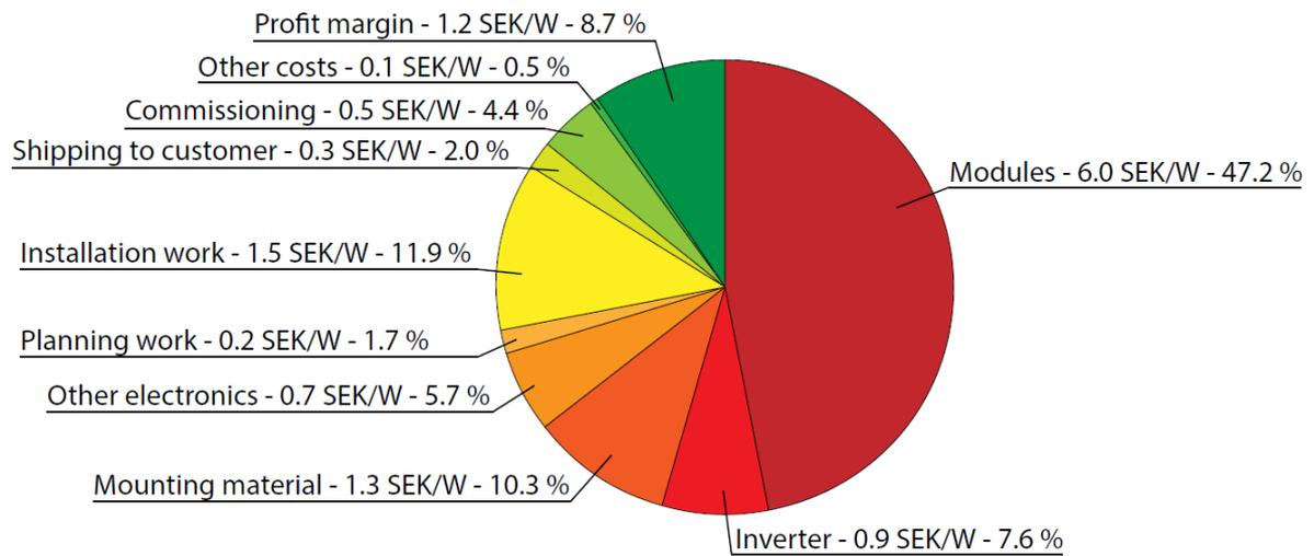
**Figure 11: Average of five Swedish installation companies cost structures for a typical turnkey grid-connected roof-mounted commercial PV system (40–60 kW<sub>p</sub>) to the end customer in the end of 2015. The average price was 12.7 SEK/W<sub>p</sub>.**
