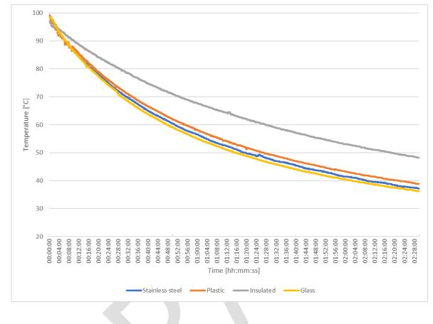
The tests presented in Figure 7-2 indicate that all single wall kettles had similar heat losses during the cool-down phase<sup>28</sup>, while the insulated container had a much better performance.<sup>29</sup> Based on these measurements, Table 7-4 shows the temperature drop after 15, 30 and 60 min for single wall kettles and for the insulated kettle.
