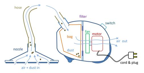
Figure 30: Key components in a mains-operated vacuum cleaner
