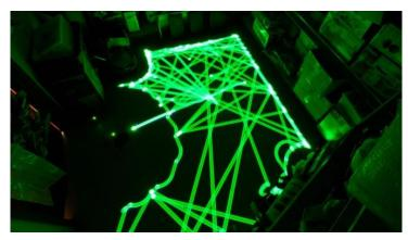
Figure 41: Robot cleaner using a random bounce pattern to cover the surface
