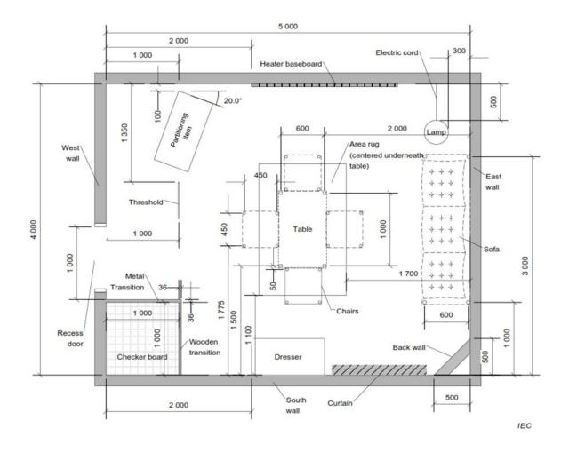
Figure 11: Floor plan for testing autonomous coverage
