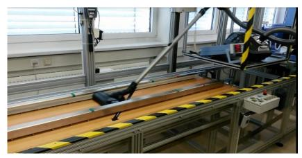
Figure 73: test rig for vacuum cleaner testing<sup>316</sup>
