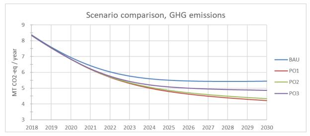
Figure 68: GHG emissions in PO1, PO2 and PO3 compared to BAU from 2018 to 2030
