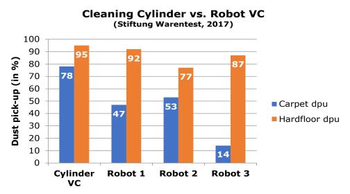
Figure 44: Dust pick-up for an average cylinder cleaner and the three best robot cleaners (source: Stiftung Warentest 2017).
