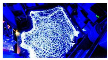
Figure 42: Robot cleaner using a random + spiralling pattern to cover the surface<sup>241</sup>
