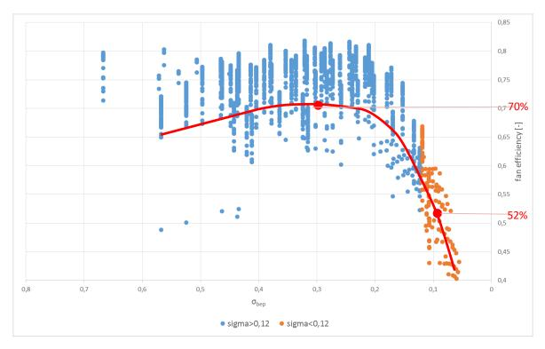
Figure 34: Fan efficiency as a function of specific speed for industrial centrifugal fans in the range up to 10 kW (source: Eurovent, EVIA. pers. comm.)
