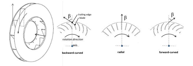
Figure 32: Backwards curved centrifugal fan (left) and fan definitions using the centrifugal
