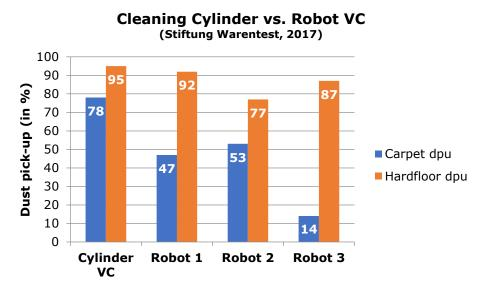
Figure iii: Dust pick-up for an average cylinder cleaner and the three best robot cleaners (source: Stiftung Warentest 2017).
