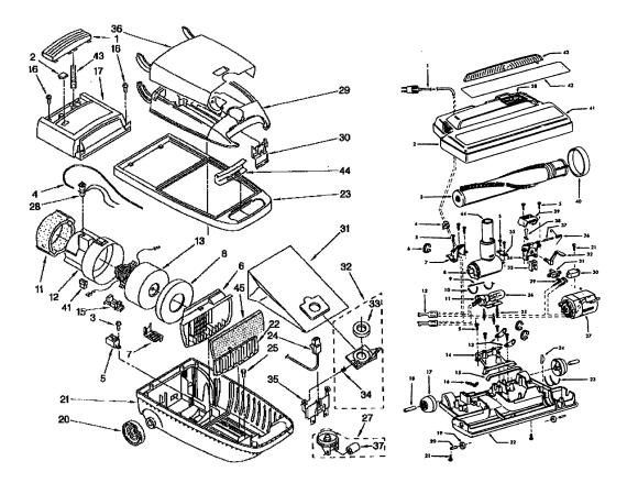
Figure 37: Example of an exploded drawing and spare parts listing for the canister (left) and the nozzle plate (right)
