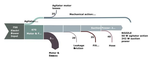
Figure 31: Sankey-diagram of energy flows in a mains-operated cylinder vacuum cleaner (source: VHK 2017 graph on the basis of AEA Ricardo 2009 data)
