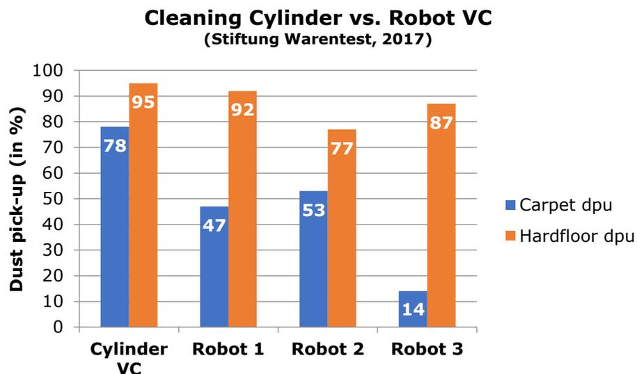
The high-end robot vacuum cleaners advertise 20 'Airwatts'<sup>39</sup> suction power, which is only 5-18% of that of an average cylinder vacuum cleaner. The relatively limited suction power is a key factor in the relatively low dust retention performance.
