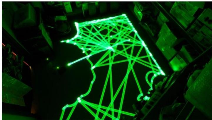
**Figure 55: Robot cleaner using a random + spiralling pattern to cover the surface<sup>308</sup>**
