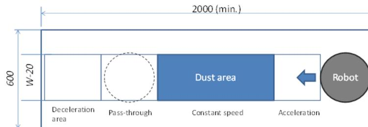
**Figure 23: Floor plan of straight-line cleaning test according to section 6**
