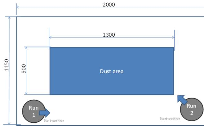
**Figure 22: Floor plan of test-box for cleaning, according to section 5**
