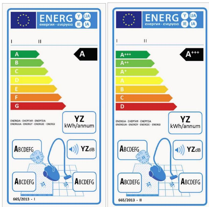
**Figure 21: The previous, annulled Energy Label 1 (left) and label 2 (right) for vacuum cleaners**
