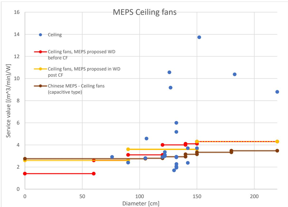
Figure 3: Data for ceiling fans collected in this study (including data from review study). Solid lines are MEPSs from working document presented at consultation forum, the revised MEPS from after consultation forum and Chinese MEPS according to standard GB/T 13380-2018.
