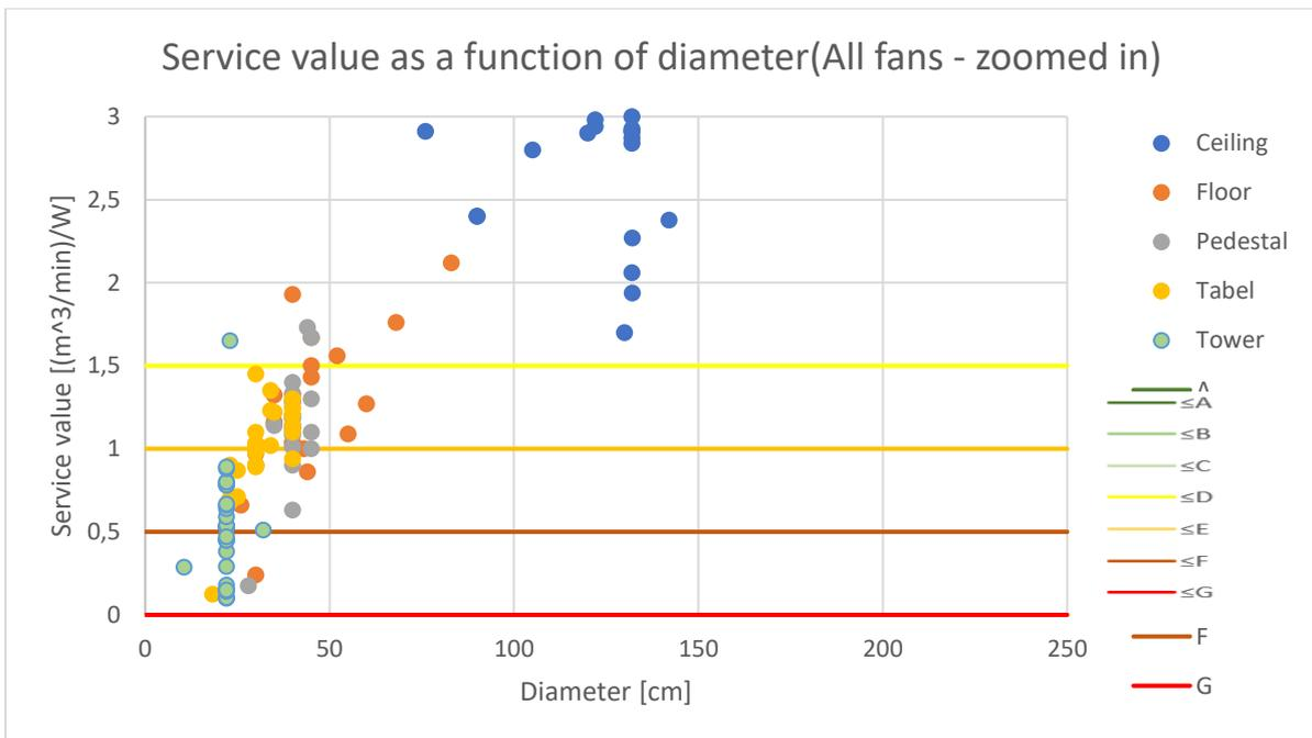
Figure 7: Suggestion for common energy label scale set independent of diameter and with uneven distribution of classes (zoomed in on 'other fans')
