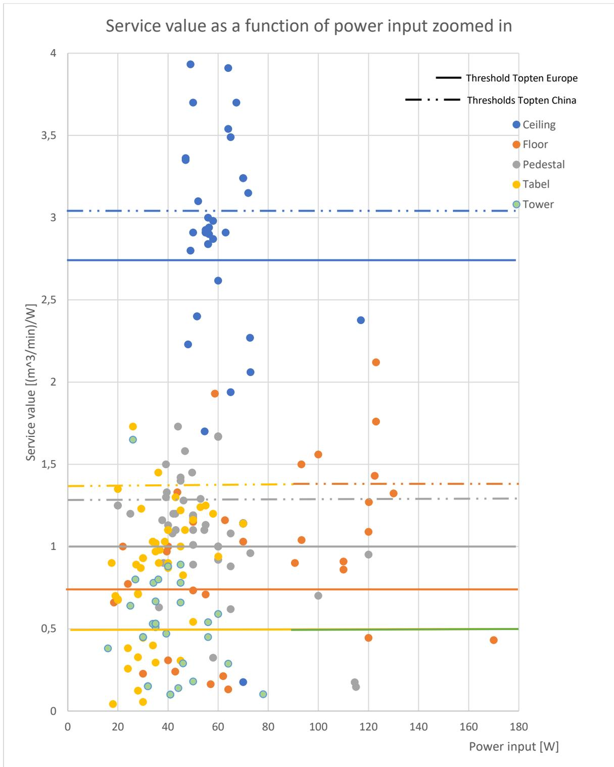
Figure 20: Data and Topten thresholds. Service value as a function of power input zoomed in on the lower service values, omitting a share of the data for ceiling fans.
