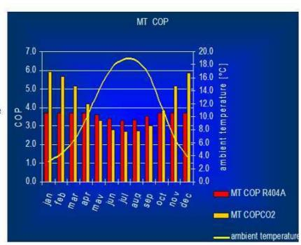
**Figure 7-81:** COP comparison of a traditional R 404A supermarket system and a CO<sub>2</sub> based system for low temperature applications
