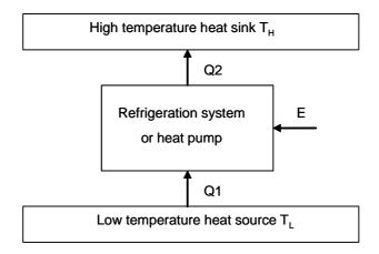
The efficiency of the refrigeration system is expressed by the COP (coefficient of performance) which is the ratio of the refrigeration effect (heat extracted) and
