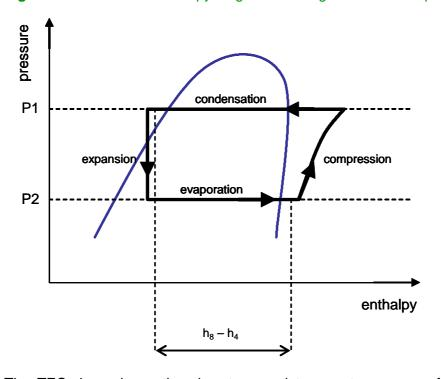
Figure 4-26: Pressure Enthalpy diagram showing measurement points
