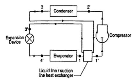
The main benefit of the use of a liquid suction heat exchanger is to avoid vapour existing into the expansion device, and to reduce the possibility of liquid transfer between the evaporator and the compressor, which could harm the latter. However, liquid-suction heat exchangers could increase the temperature and reduce the pressure of the refrigerant entering the compressor causing a decrease in the refrigerant density and compressor volumetric efficiency.
