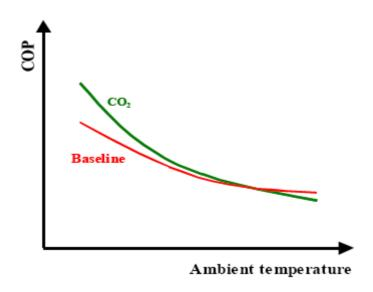
Another drawback ok  $CO_2$  is high pressures required in the refrigeration system for a good operation, due to transcritical operation of the process. This has consequences on the use of raw materials (more material is used) and therefore on the final cost of the appliance.
