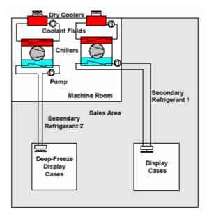
Other secondary loops, containing coolant fluid, are used in the system to transport heat rejected from condensers, to dry coolers often located on the roof of the supermarket. This allows not to warm over the machine room, and therefore to less use air conditioning.
