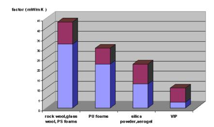
Figure 6-6: Thermal conductivity of various insulating materials<sup>12</sup>
