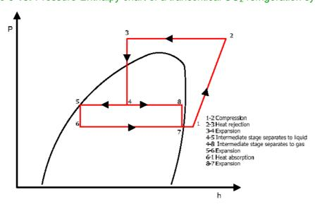
Figure 6-18: Pressure-Enthalpy chart of a transcritical CO<sub>2</sub> refrigeration system
