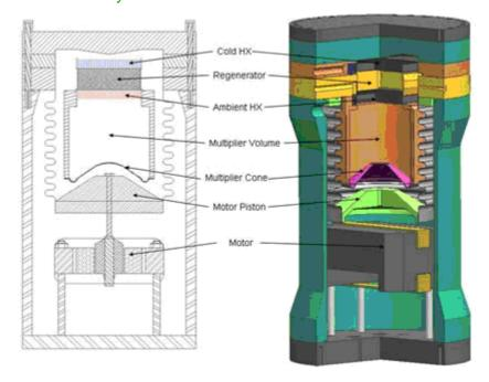
Figure 6-25: Cut-away view of the thermo-acoustic chiller<sup>42</sup>
