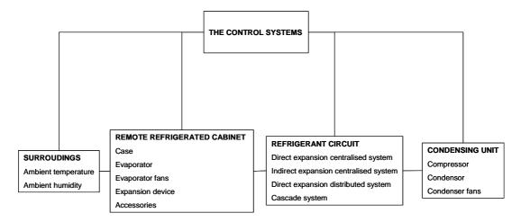
The functional system of remote refrigerated display cabinet includes:
