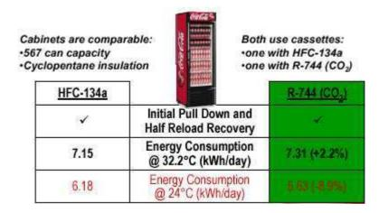
**Figure 6-22:** Comparison of two refrigeration equipments using R134a and  ${\rm CO_2}^{34}$
