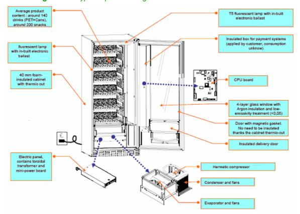
Figure 4-9: Typical spiral vending machine<sup>11</sup>
