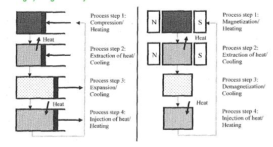
The Camfridge programme from Cambridge University develops a revolutionary magnetic refrigeration technology. Magnetic refrigeration promises a number of benefits over the vapour compression technology, including a significant reduction in energy consumption, elimination of refrigerant leakage and ease of recycling.
