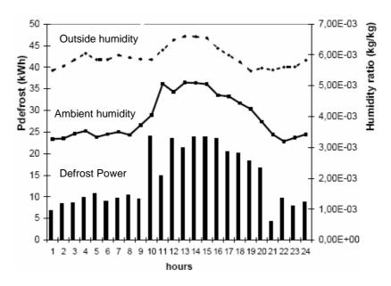
Humidity impacts the refrigeration system energy use by 10 - 20 kWh/day per % RH $^{58}$  in an average store mainly influencing the anti-sweat heaters and the electric defrost, and having a less significant impact on hot gas defrost systems.
