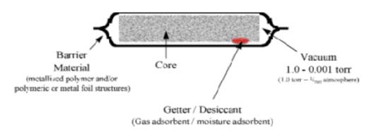
The benefit of using vacuum insulated panels is that they have thermal conductivity lower than conventional insulators such as polyurethane and polystyrene foams, thus allows achieving superior insulation performances. This implies energy savings without increasing insulation thickness.
