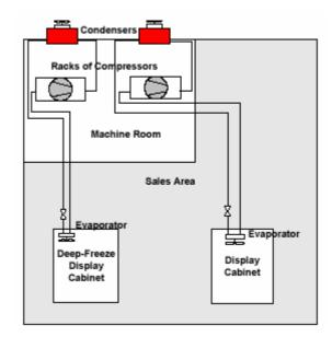
This above figure (Figure 4-40) contains one rack of compressors; it is a multiplex direct refrigeration system, the most common direct system in supermarkets. For small sets of display cases, a single-compressor condensing unit is used.
