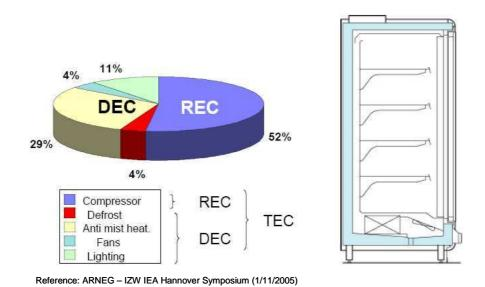
**Figure 4-29:** Electricity consumption distribution of a chilled vertical multi deck remote display cabinet<sup>27</sup>
