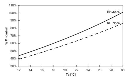
One big energy efficiency issue is the determination of the optimum set points for Ta and RH (optimal ambient conditions) taking into account considerations for the comfort of the shoppers. Simulation programs are currently under development.
