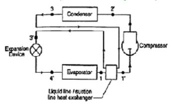
The main benefit of the use of a liquid suction heat exchanger is to avoid vapour existing into the expansion device and to reduce the possibility of liquid transfer between the evaporator and the compressor, which could harm the latter. However, liquid-suction heat exchangers could increase the temperature of the refrigerant and reduce the pressure of the refrigerant entering the compressor causing a decrease in the refrigerant density and compressor volumetric efficiency.
