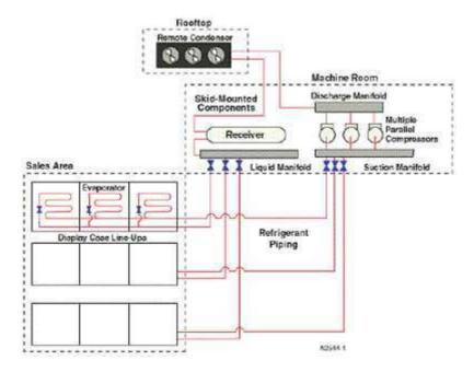
Figure 7-79: Base-line refrigeration system
