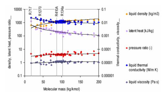
Figure 4-18: Variation of refrigerant thermodynamic properties<sup>16</sup>
