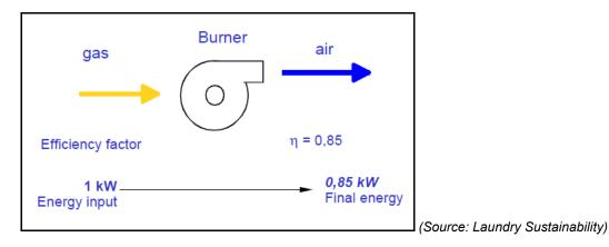
Figure 22 Energy conversion process in a direct (internal) gas heating system
