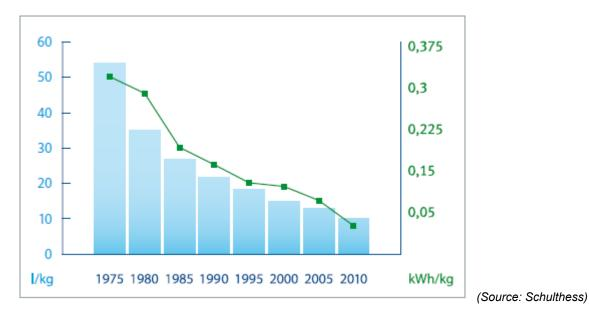
Figure 1 Development of the water and energy consumption of commercial appliances from the Swiss manufacturer Schulthess (this figure is comparable to categories WM2 and WM3)
