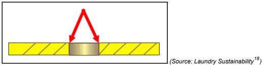
Figure 7 Cylindrical perforation of washing machines' inner drums
