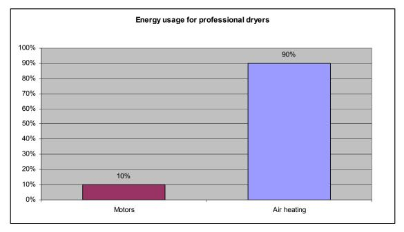
Figure 11 Energy use for a typical professional air dryer cycle<sup>27</sup>
