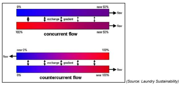
The principle of a heat exchanger is illustrated in Figure 2.
