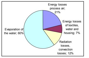
Figure 10 Energy use for a typical professional condenser dryer <sup>26</sup>
