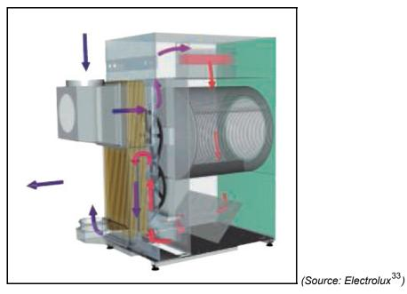
Figure 13 Air flow of the heat recovery system
