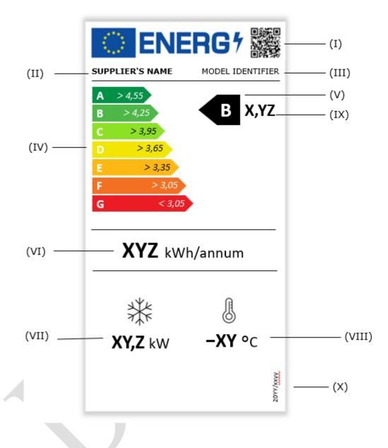
[Label above is of a MT condensing unit with cooling capacity 5-50 kW and is for illustration only – not the proposed design (to be completed once draft has been agreed).]
