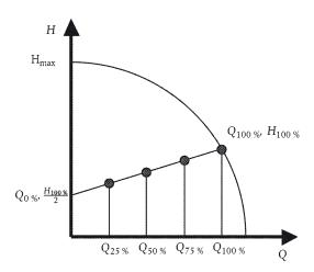
7. Select a setting of the circulator ensuring that the circulator on the selected curve reaches  $Q \cdot H = max$  point. For circulators integrated in products follow the reference control curve by adjusting the system curve and speed of the circulator.
