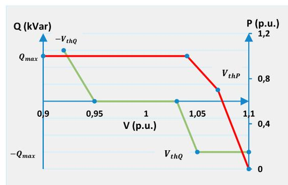
Figure 13: Active power and reactive power control of PV inverter for voltage regulation.
