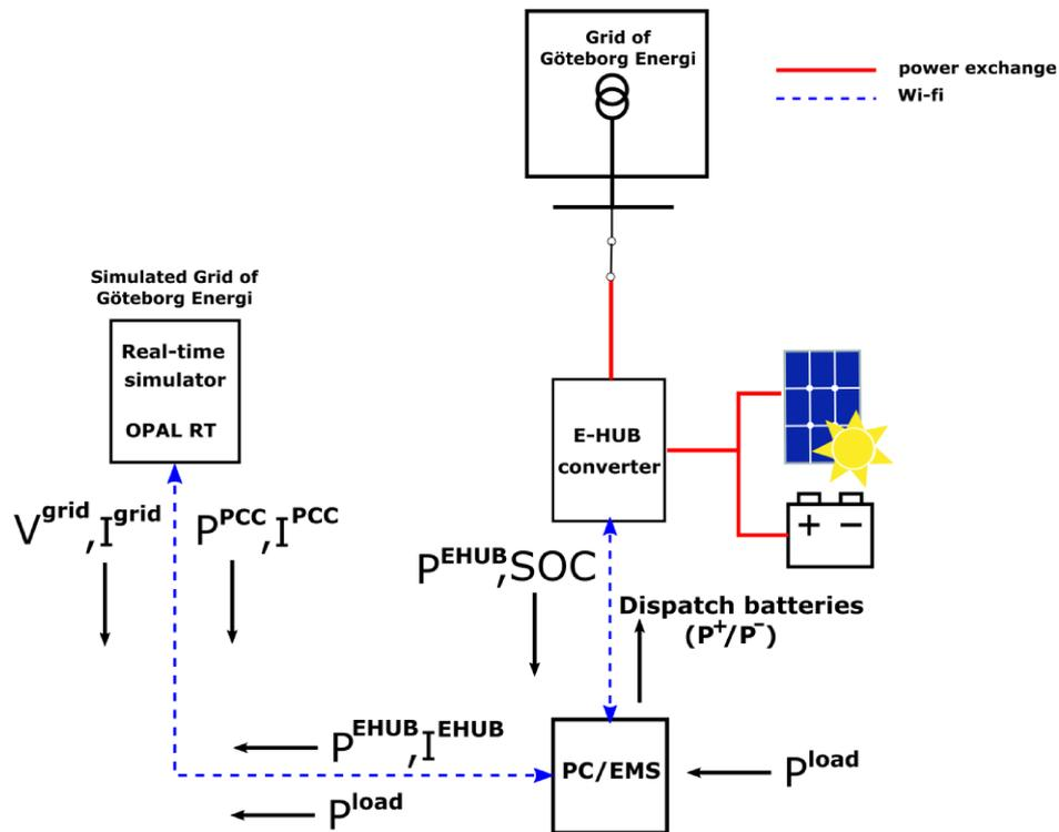
Figure 17 : Set-up with real-time simulator for the micro-grid to DMS coordination at Brf Viva test site.
