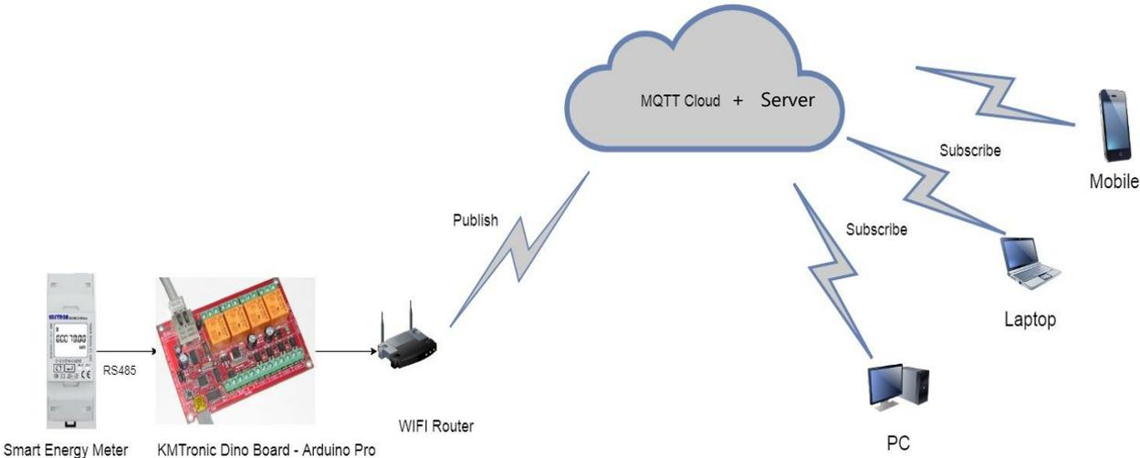
Figure 20: Example of monitoring system applied to PV
