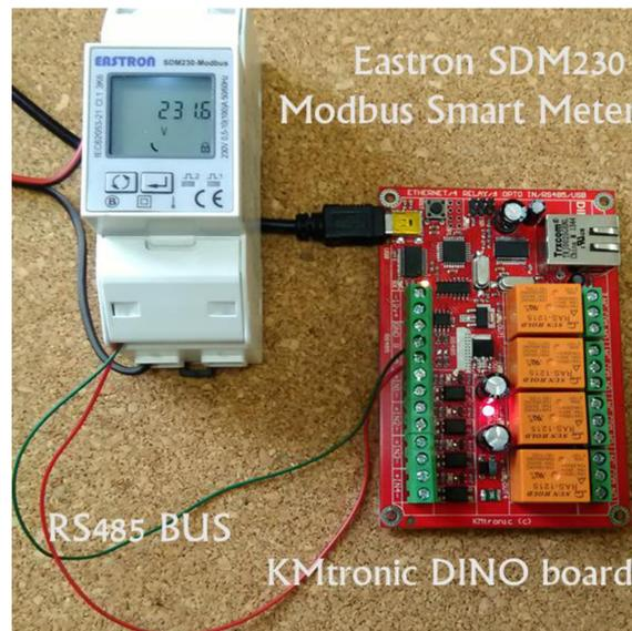
Figure 19: Proposed real-time measurement platform.
