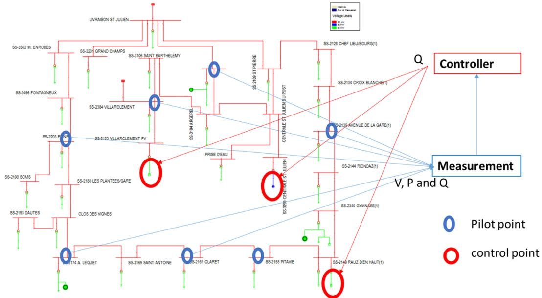
Figure 18: Pilot points and controllable plant in the single line diagram.
