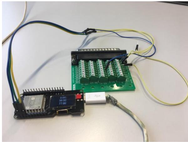
Figure 12: Voltage control prototype.
