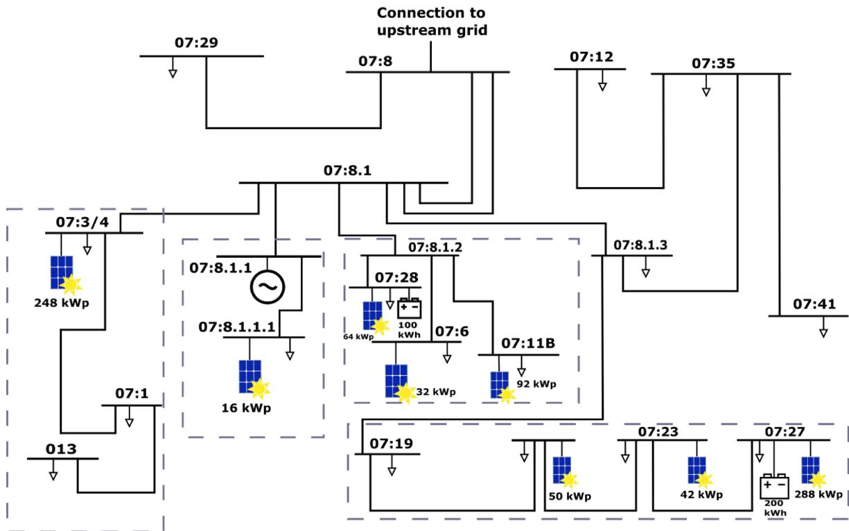
Figure 1 : The areas which are candidate for micro-grid implementation at the distribution network of Chalmers campus.
