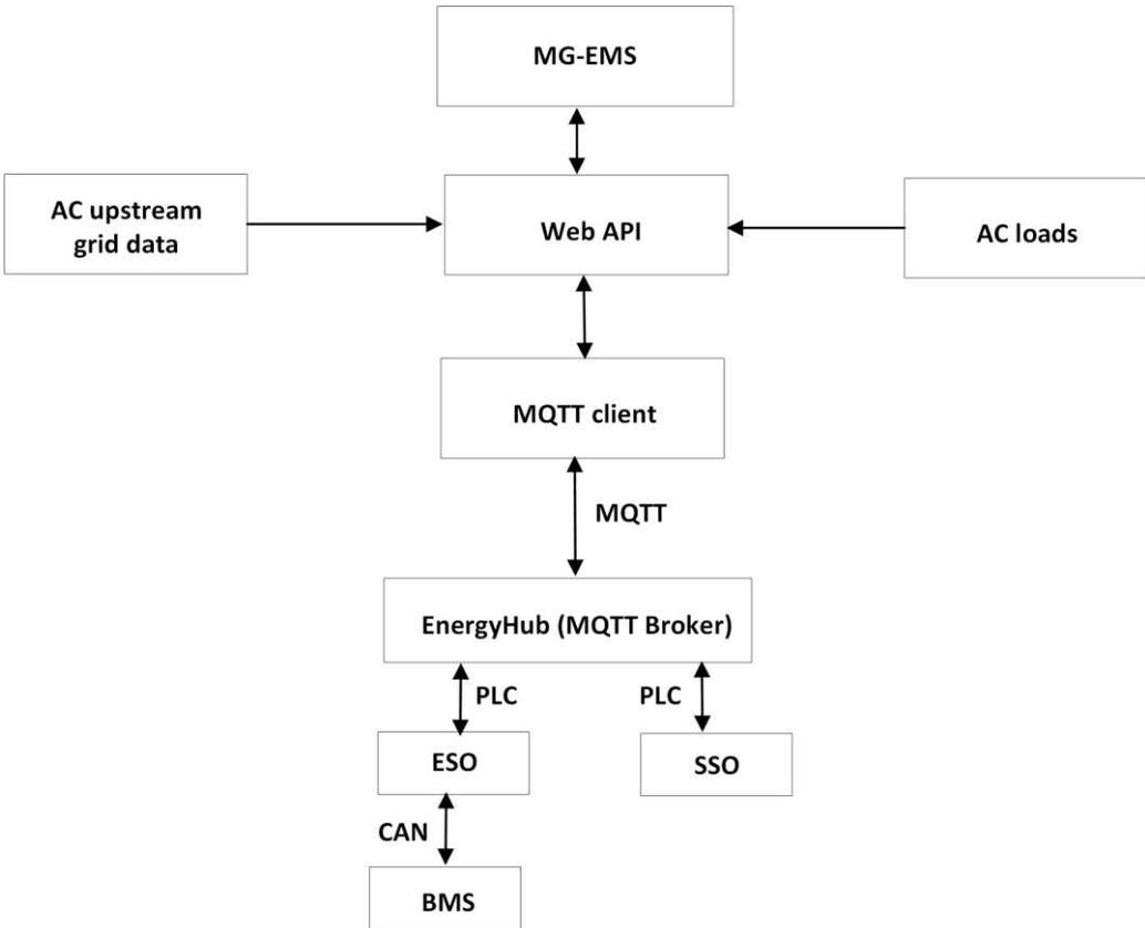
Figure 14: The communication interface set-up for the MG-EMS in Brf Viva.
