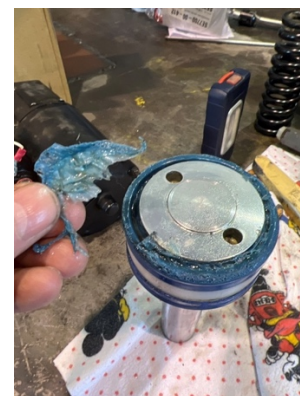
Figure 2, Broken seal on brake cylinder.
