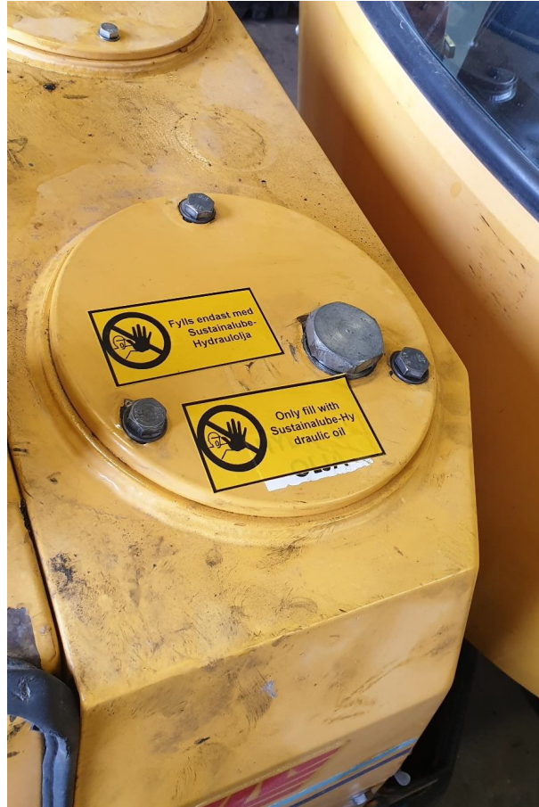
Fig 4. Hydraulic fluid tank with warning decals on, also wrong notion here with “oil” but the message should be clear: Only use Sustainalube
