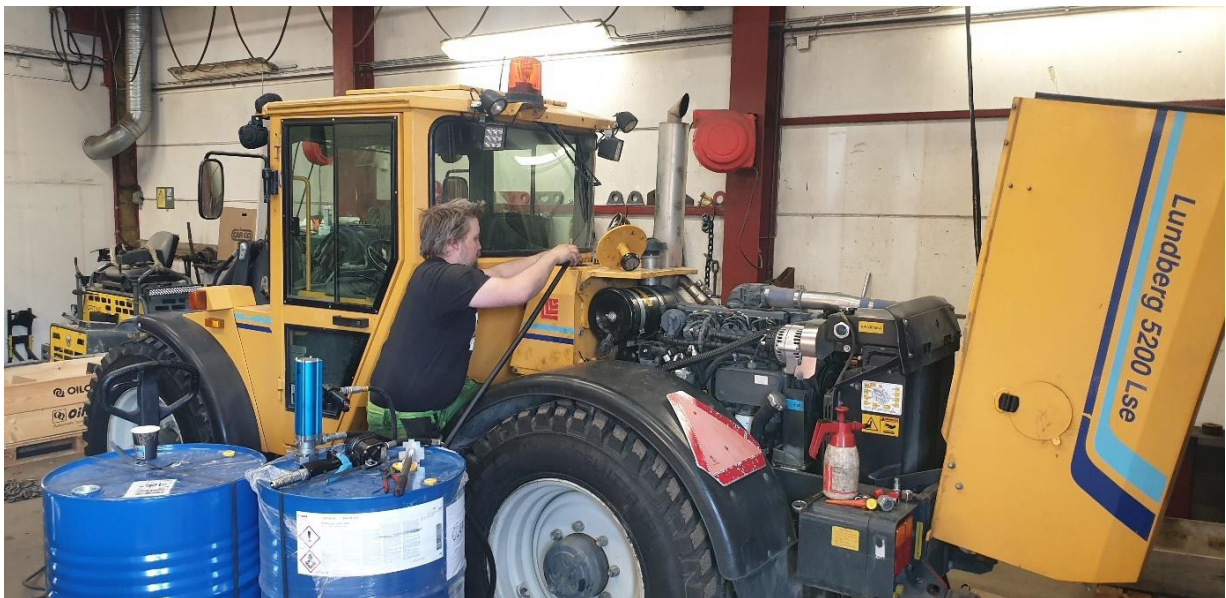
Fig 1. Leif is filling the first batch of flushing fluid in the hydraulic tank.
