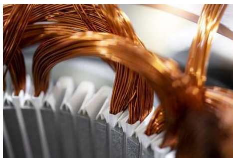
Figure 1. Components of the insulation system of electrical machine: slot liner in the slot and insulating coating on the wires.
