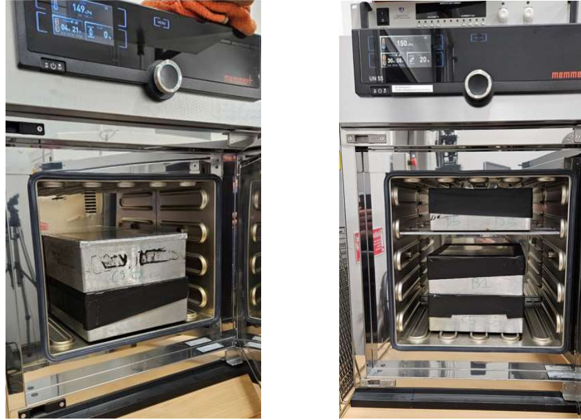
Figure 3. Containers with formettes immersed in oil inside the ovens.
