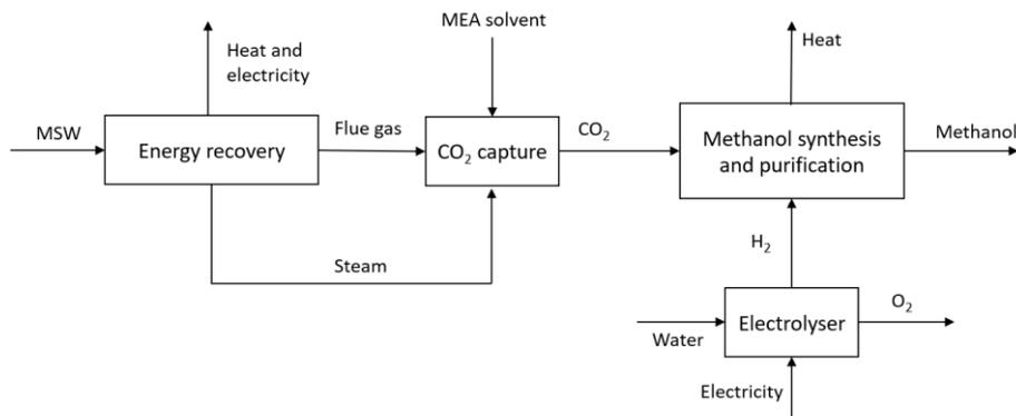
Figure 2. Schematic of methanol production by hydrogenation of the captured CO<sub>2</sub> from the waste-to-energy plant
