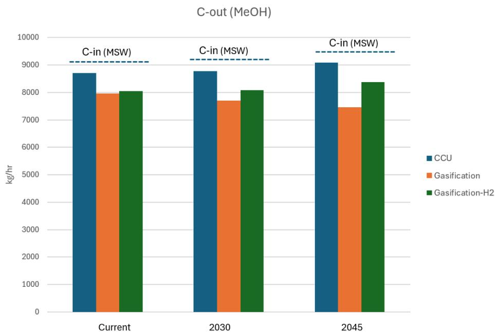
Figure 4. The amount of carbon in and out of each configuration under the current, 2030, and 2045 scenarios
