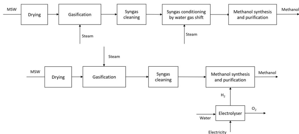
Figure 1. Schematic of methanol production by Gasification and Gasification-H<sub>2</sub> followed by methanol synthesis and purification
