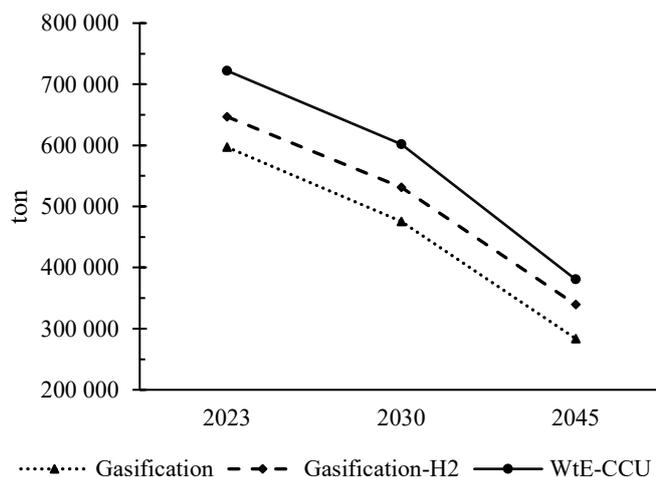
Figure 7. Total potential methanol production from municipal solid waste for the different pathway technologies
