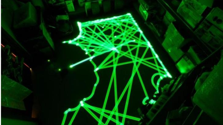
**Figure 41: Robot cleaner using a random bounce pattern to cover the surface**
