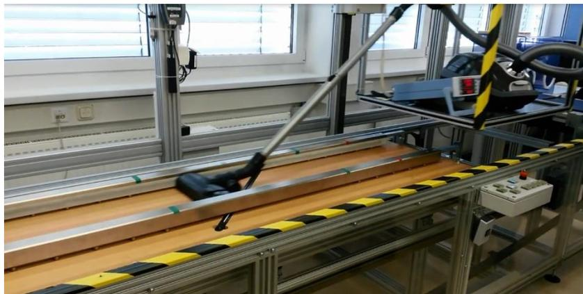
Figure 73: test rig for vacuum cleaner testing<sup>316</sup>
