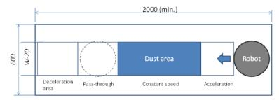
Figure 23: Floor plan of straight-line cleaning test according to section 6
