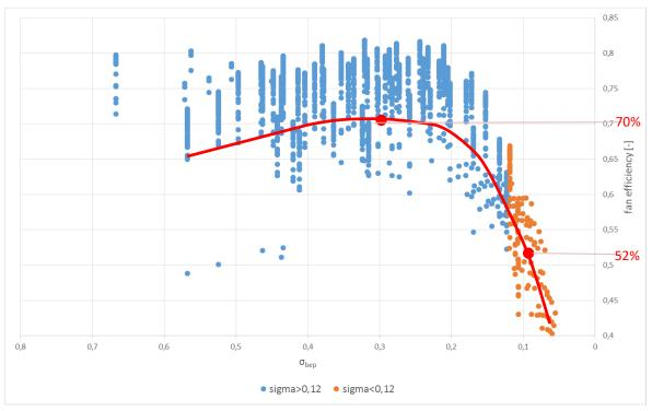
Figure 47: Fan efficiency as a function of specific speed for industrial centrifugal fans in the range up to 10 kW (source: Eurovent, EVIA. pers. comm.)
