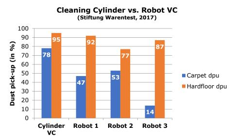
The high-end robot vacuum cleaners advertise 20 'Airwatts'<sup>39</sup> suction power, which is only 5-18% of that of an average cylinder vacuum cleaner. The relatively limited suction power is a key factor in the relatively low dust retention performance.
