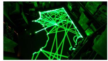
Figure 54: Robot cleaner using a random bounce pattern to cover the surface
