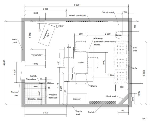
Figure 24: Floor plan for testing autonomous coverage
