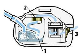
The dust stays in the bag, falls in the receptacle or stays in the water for later disposal. The air moves on to the second stage, nowadays typically a HEPA (High Efficiency Particle Air) filter, that takes out the last 0.1% of dust particles and prevents (together with appropriate seals) re-emission of dust into the room.
