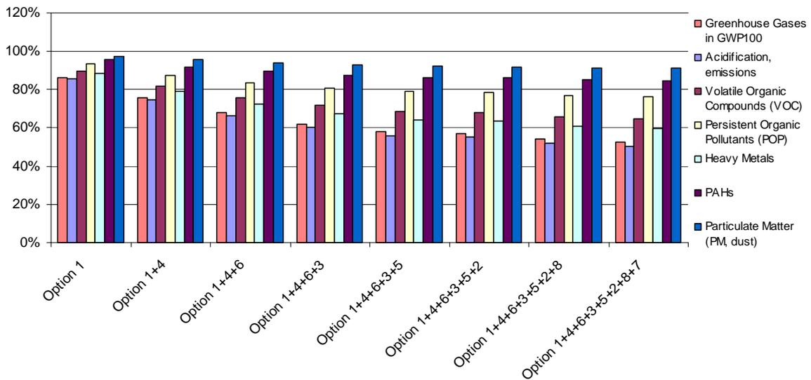
**Annexe 7-34: Comparison of the cumulative improvement options (emissions to water) base case beverage cooler in the order of LCC**
