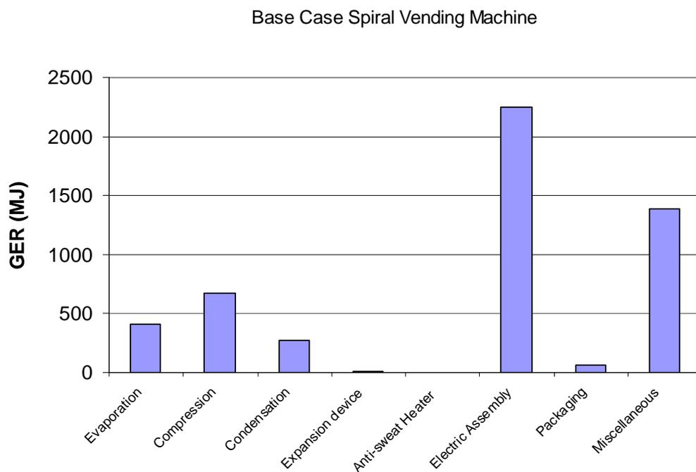
The GER during the production phase is of 40,831 MJ (36,801 MJ for the raw materials use and 4,030 MJ for the manufacturing). The housing makes up for more than 87 %, followed by the electric assembly module (5.5 %) and the miscellaneous module (3.4 %), for the whole production phase. This can be explained by the high proportion represented by the housing (about 87 %).
