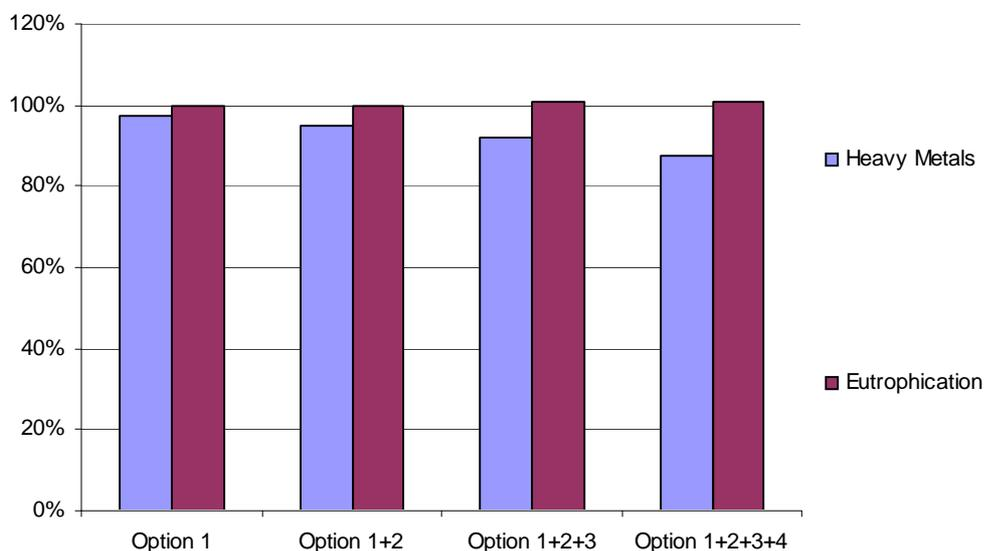
For almost all environmental indicators (resource and waste, emission to air and water) except EUP, the option 1+2+3+4 leads to the highest impact reduction in comparison with the base case ice cream freezer. It is followed by option 1+2+3 and option 1+2.
