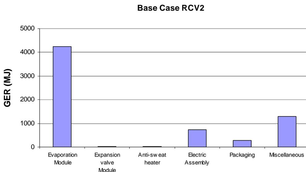
It is clearly visible that the housing contributes the bulk (> 80 %) of the total energy consumption during production phase, followed by the evaporation module. This can be explained by the high mass proportion of these two modules (housing and evaporation modules represent 85 % and 5.95 % mass of the base case RCV2 respectively).
