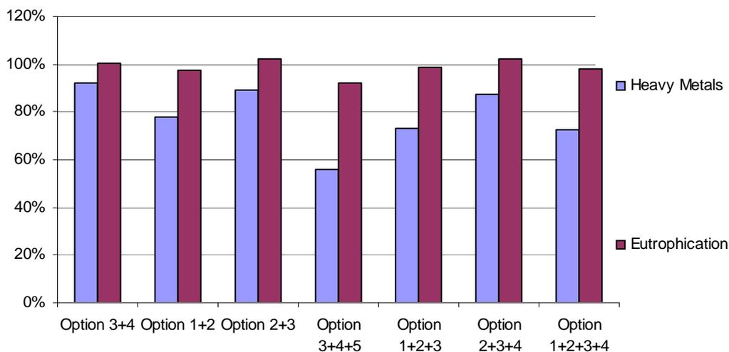
For all 15 environmental impact indicators (2 other are negligible for all base cases and for all combinations of improvement options), the best performing option (i.e. leading to the highest reductions with reference to the base case RCV2) is the option with glass door: option 3+4+5. The second best option is 1+2+3+4 (without glass door but with night curtain during 12 hours) and the third best performing option is option 1+2+3.
