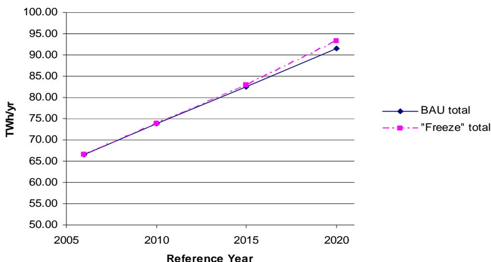
In 2020, when comparing BAU scenario to the “Freeze” scenario, the total annual TEC for the sub-scenario with the same temperature classes for remote cabinets is 14.3 % lower. The reduction is of 4.2 % when RCV2 and RHF4 operate with temperature classes 3M1 and 3L1.
