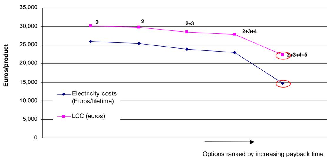
**Figure 7-34:** Energy consumption during use phase versus LCC for the base case RHF4 (with glass lid)
