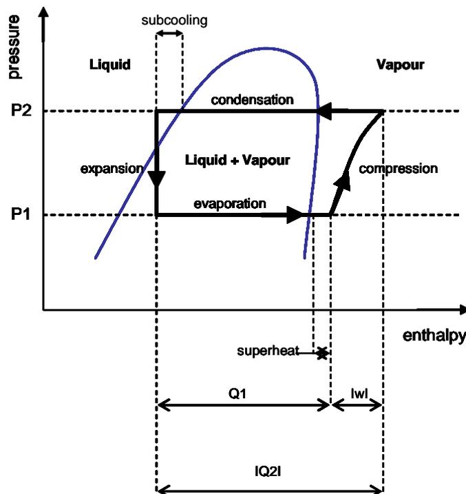
Q1: heat transferred at the evaporator (pressure P1) corresponding to the refrigeration effect
