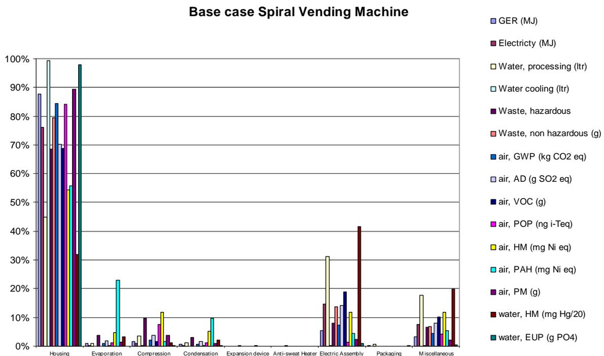
**Figure 5-49: Impacts related to the production phase for each module (excluding the housing)**
