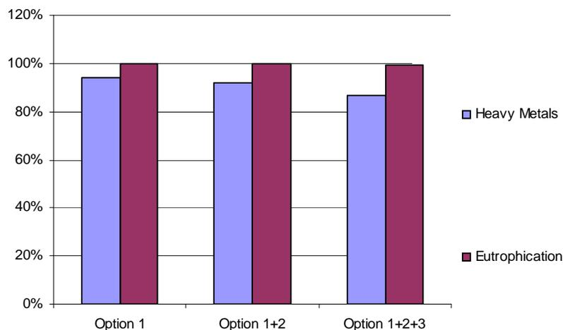
The full combination of the 3 options leads to the highest reduction for all environmental impacts. This ranking corresponds to the order of the LCC and to the order of total electricity consumption.
