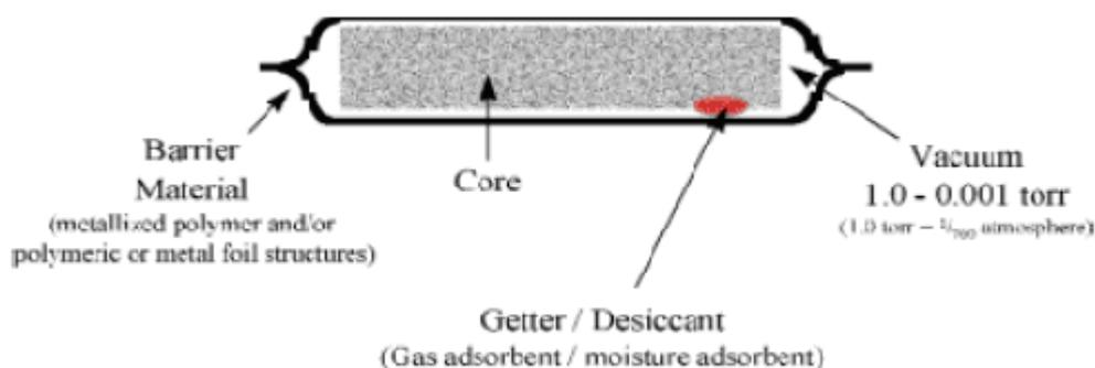
The benefit of using vacuum insulated panels is that they have thermal conductivity lower than conventional insulators such as polyurethane and polystyrene foams, thus allows achieving superior insulation performances. This implies energy savings without increasing insulation thickness.
