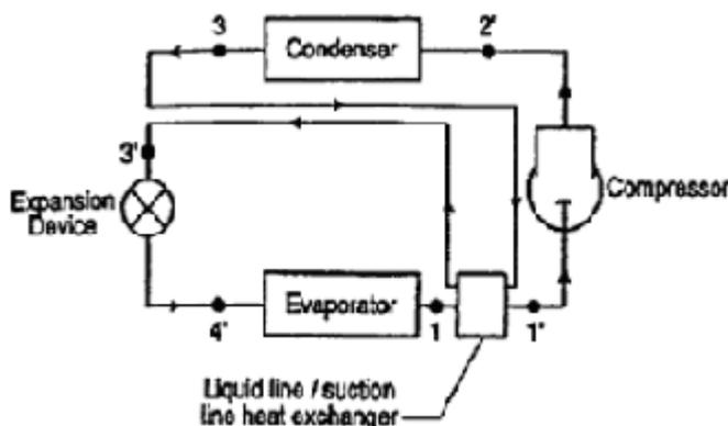
The main benefit of the use of a liquid suction heat exchanger is to avoid vapour existing into the expansion device and to reduce the possibility of liquid transfer between the evaporator and the compressor, which could harm the latter. However, liquid-suction heat exchangers could increase the temperature of the refrigerant and reduce the pressure of the refrigerant entering the compressor causing a decrease in the refrigerant density and compressor volumetric efficiency.
