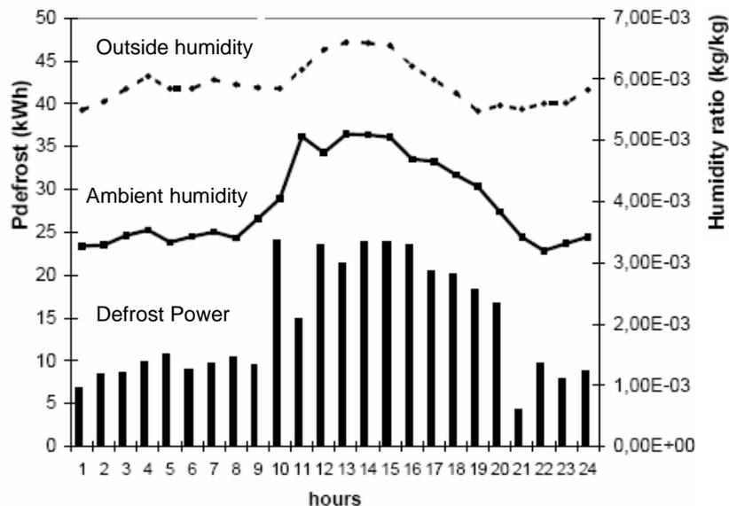
Humidity impacts the refrigeration system energy use by 10 - 20 kWh/day per % RH<sup>58</sup> in an average store mainly influencing the anti-sweat heaters and the electric defrost, and having a less significant impact on hot gas defrost systems.
