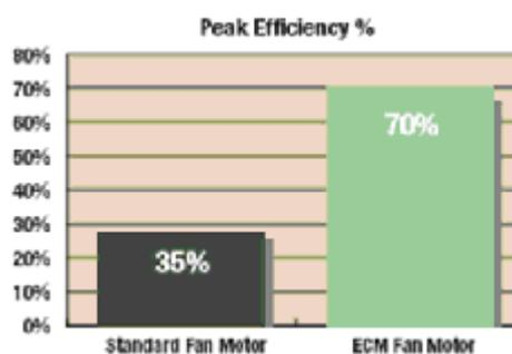
Besides, ECM fan technology provides 90,000 hours of operation on average, which is twice of that a standard fan motor.
