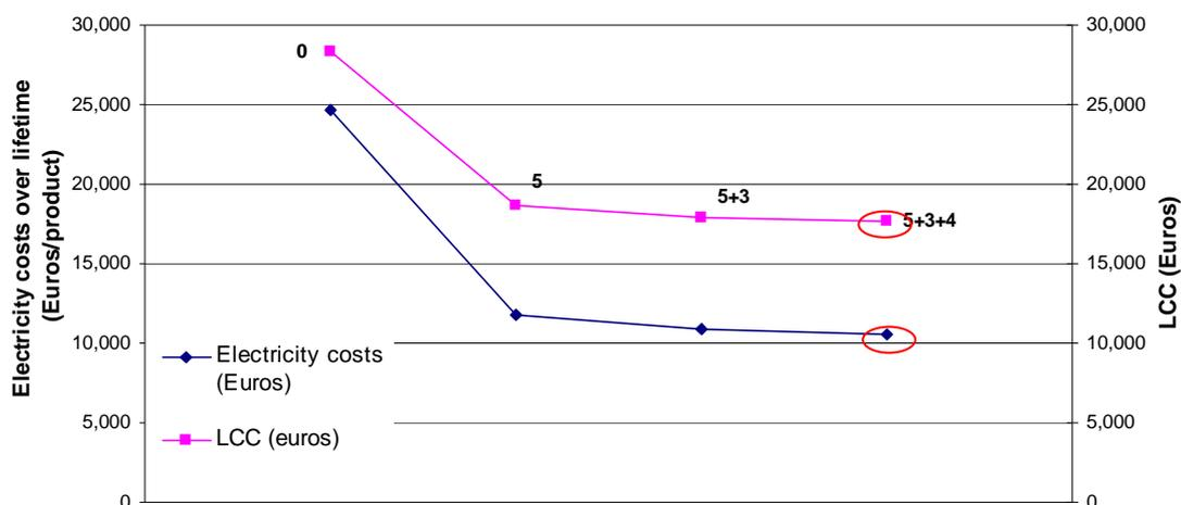
**Figure 7-29: Energy consumption during use phase versus LCC for the base case RCV2 (with glass door)**
