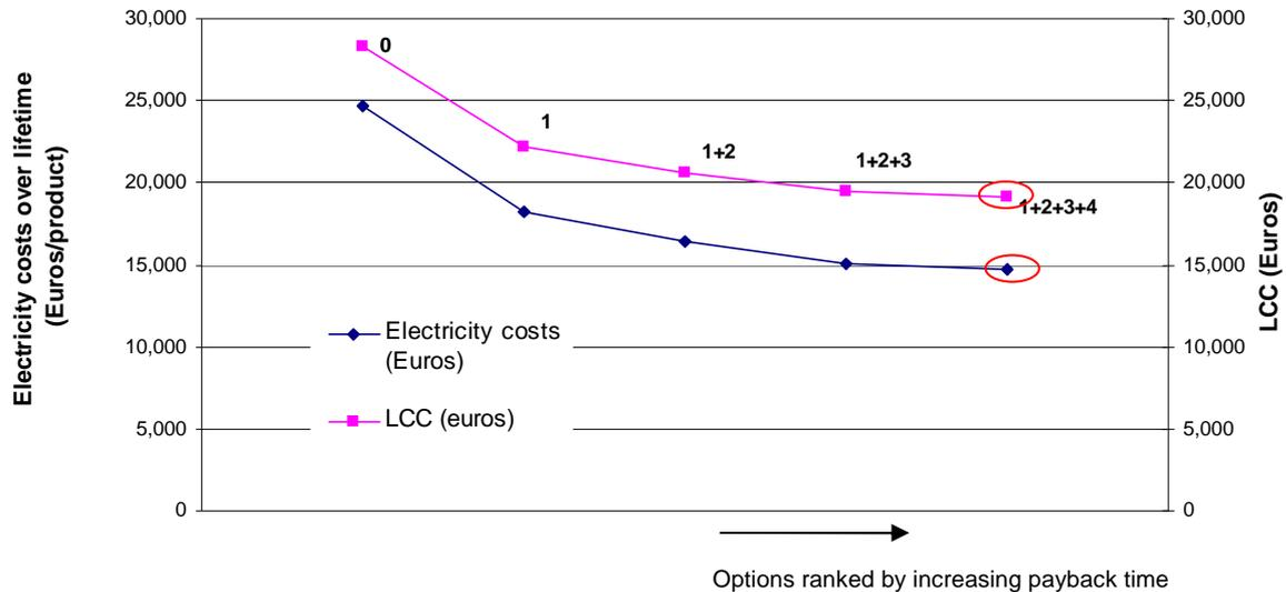
The option with BAT and presenting the LLCC is the combination option 1+2+3+4 which leads to 40 % reduction in electricity consumption during use phase and a 32 % lower LCC (see Table 7-18). Figure 7-21 and Figure 7-22 illustrate once again how closely the LCC and the electricity consumption correlate and this explains why the BAT coincides with the LLCC since most of the environmental impacts are due to the use of electricity.
