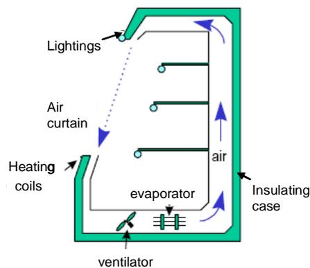
High pressure liquid and suction refrigerant piping must be connected to the case. Additional connections are electrical power supply and the drain lines for the condensate (from the defrost operation).
