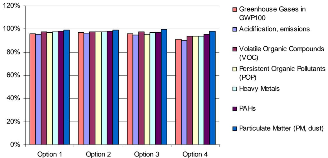
**Figure 7-12:** Comparison of the individual options (emissions to water) for the base case ice cream freezer
