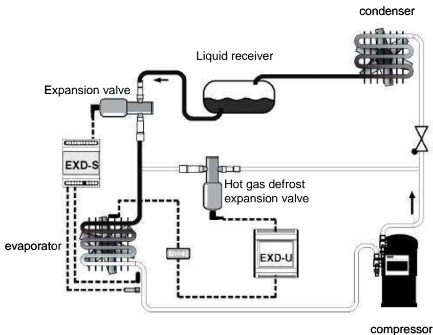
In a typical supermarket, the electric and hot or cool gas defrost is normally controlled by a preset time cycle with most display cabinets timed to defrost every 6 hours for a duration of 10 minutes<sup>16</sup>.
