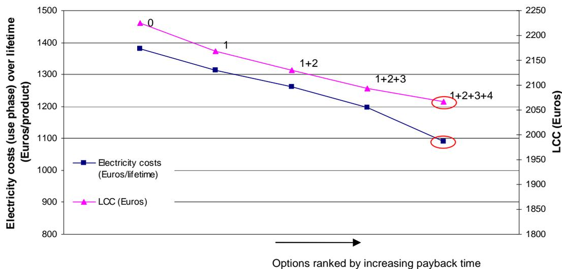
**Figure 7-62:** Energy consumption during use phase versus LCC for the base case ice cream freezer
