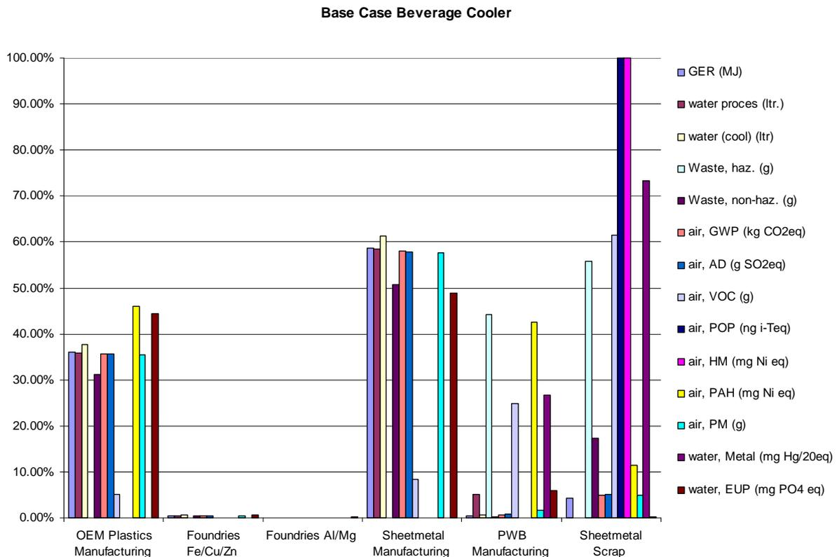
The analysis of the production phase shows that the most impacting components are the stainless steel panels used for the cabinet structure, the foam insulation and the materials used for the heat exchangers. However, as for the base case RCV2 it is critical to consider the reduction of plastic foam or non ferro metal for the heat exchangers as the reduction of the use of these materials has a direct impact of the performance of the cabinet.
