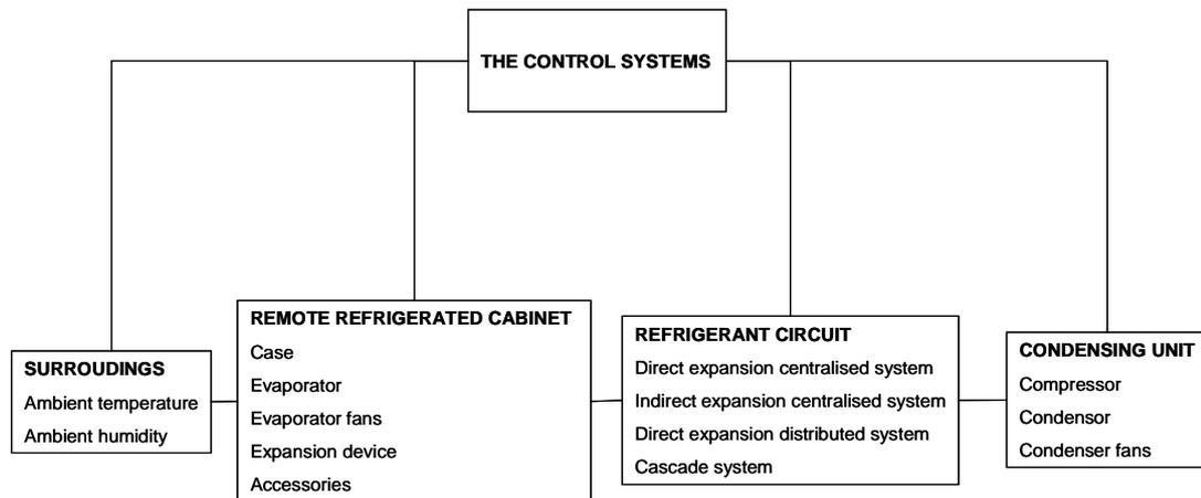
The functional system of remote refrigerated display cabinet includes:
