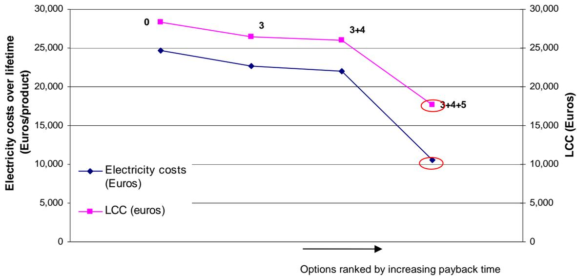
**Figure 7-20: Energy consumption during use phase versus LCC for the base case RCV2 (with glass door)**
