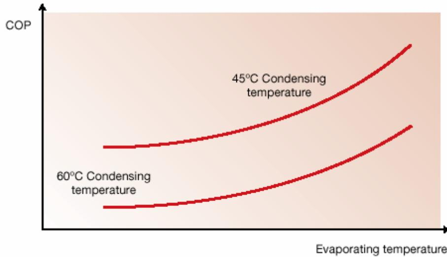
In order to increase the energy efficiency of the complete refrigeration system, the compressor control has got a relevant part. The compressor is chosen to supply power at the limiting conditions of the refrigerated display cabinet (maximum temperature and moisture). Most of the time, it does not operate at 100 %. Thereby, the compressor with the best COP under nominal conditions is not necessarily the best under real operation conditions.
