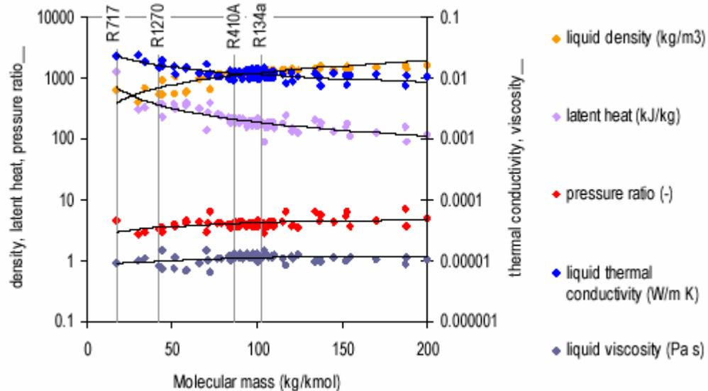
Refrigerants with a lower molecular mass, as ammonia (R 717) and propylene (R 1270) seem to have the favourable thermodynamic properties, thus higher efficiency. However environmental and safety characteristics have to be taken into account to have a global point of view on benefits and weakness of the refrigerant.
