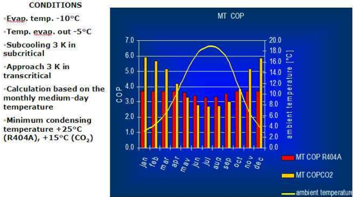
**Figure 7-81:** COP comparison of a traditional R 404A supermarket system and a CO<sub>2</sub> based system for low temperature applications
