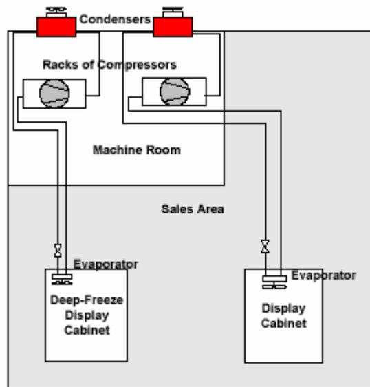
This above figure (Figure 4-40) contains one rack of compressors; it is a multiplex direct refrigeration system, the most common direct system in supermarkets. For small sets of display cases, a single-compressor condensing unit is used.
