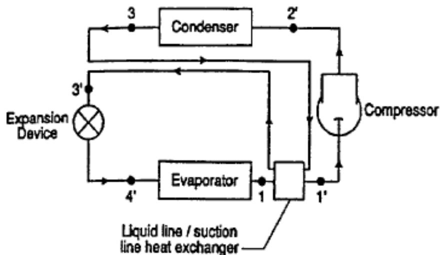
The main benefit of the use of a liquid suction heat exchanger is to avoid vapour existing into the expansion device, and to reduce the possibility of liquid transfer between the evaporator and the compressor, which could harm the latter. However, liquid-suction heat exchangers could increase the temperature and reduce the pressure of the refrigerant entering the compressor causing a decrease in the refrigerant density and compressor volumetric efficiency.
