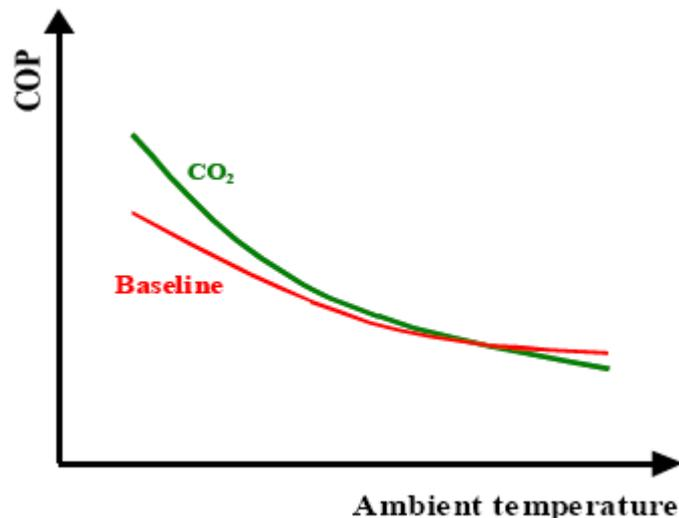
Another drawback of CO<sub>2</sub> is high pressures required in the refrigeration system for a good operation, due to transcritical operation of the process. This has consequences on the use of raw materials (more material is used) and therefore on the final cost of the appliance.
