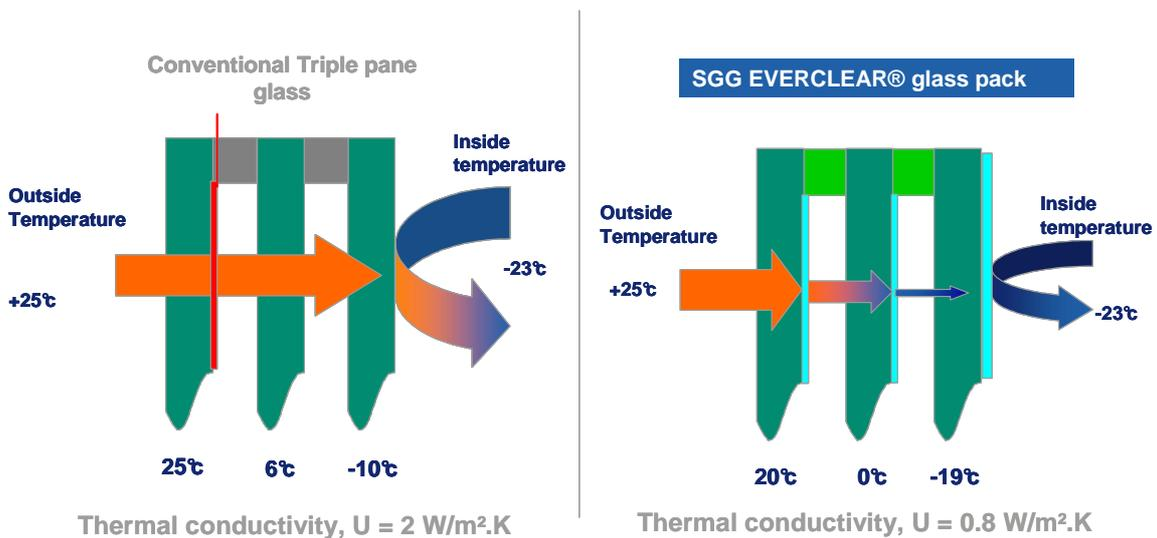
Besides of the electricity savings, the high light transmission of the SGG Everclear® glass pack allows a better visibility of products, and does not require any maintenance.
