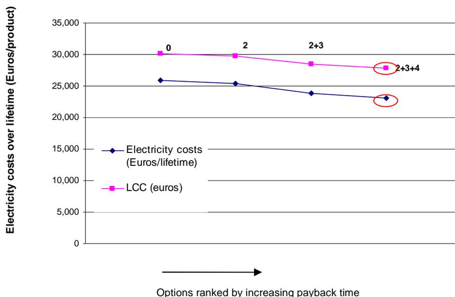
**Figure 7-38:** Energy consumption during use phase versus LCC for the base case RHF4 (without night curtain)
