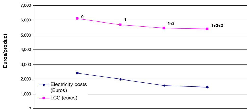
**Figure 7-77: Energy consumption during use phase versus LCC for the base case spiral vending machine**
