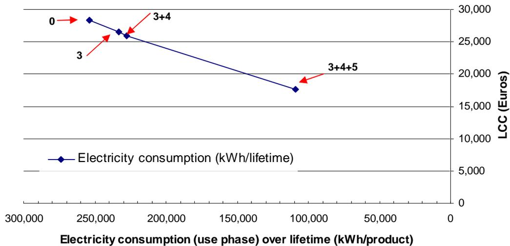
When considering the addition of a glass door, the option 3+4+5 is the option with BAT and LLCC. It leads to over 57 % reduction in electricity consumption during use phase and a 37.5 % lower LCC (see Table 7-17).
