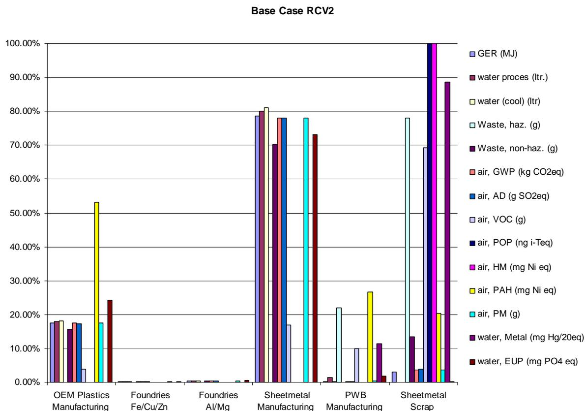
In the production phase (production and manufacturing) for the base case RCV2, major impacts are due to the material and manufacture of the housing and of the evaporator. However, modification of the design of these components would imply reduction of the performance of the appliance during the use phase and therefore cannot really be considered as an area of improvement. Focus should be made on the use phase which represents the most impacting phase (over 95 % of the total life cycle GER).
