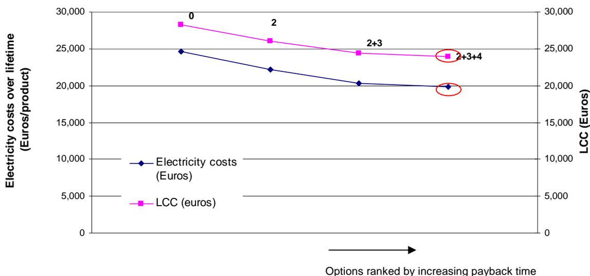
**Figure 7-24:** Energy consumption during use phase versus LCC for the base case RCV2 (without night curtain)
