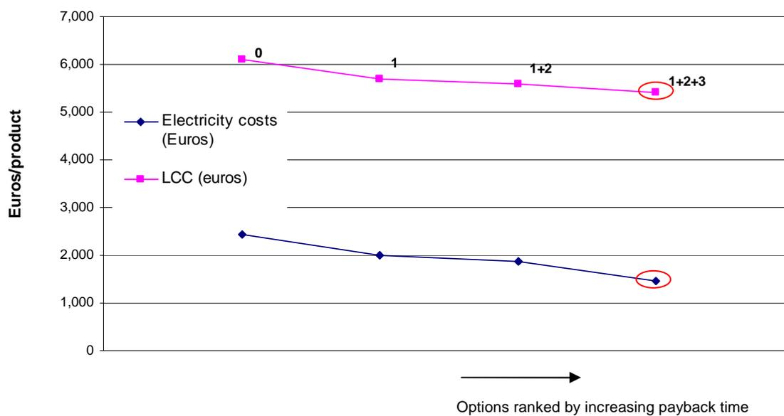
**Figure 7-72: Energy consumption during use phase versus LCC for the base case spiral vending machine**
