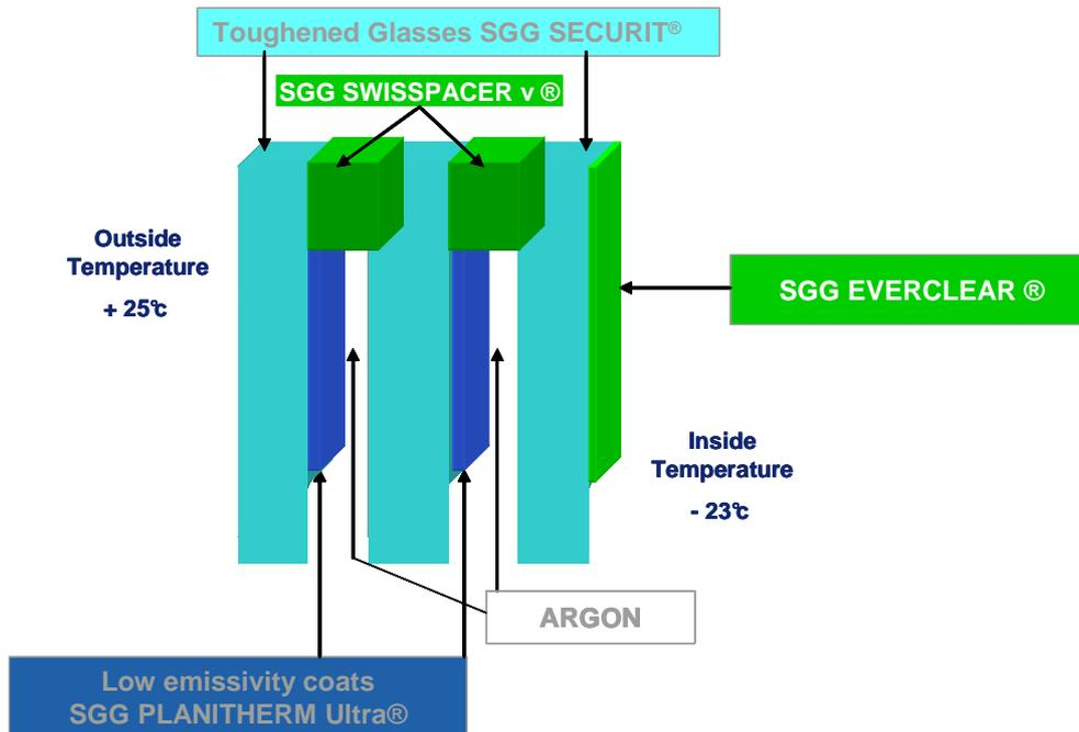
As shown in Figure 6-10, the lower thermal conductivity with the SGG Everclear® implies a lower temperature for products inside the cabinet and a better homogeneity.
