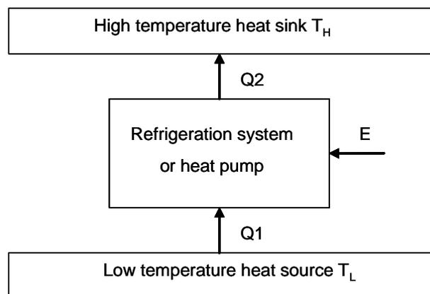
The efficiency of the refrigeration system is expressed by the COP (coefficient of performance) which is the ratio of the refrigeration effect (heat extracted) and the energy input required:  $COP = \frac{Q_1}{E}$
