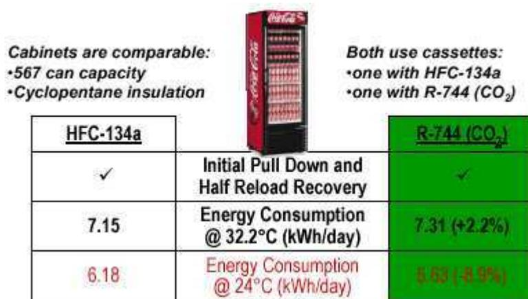
**Figure 6-22:** Comparison of two refrigeration equipments using R134a and CO<sub>2</sub><sup>34</sup>
