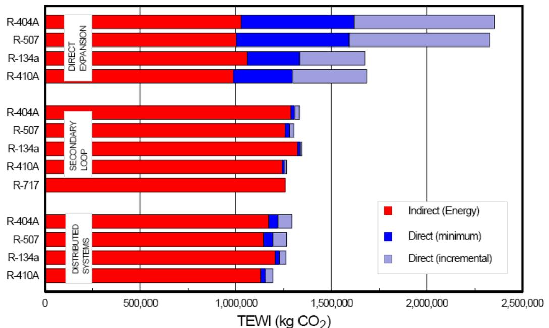
However, refrigeration experts agree that it is very difficult to compare the quality in terms of environmental impacts and energy efficiency of different refrigeration systems because no objective tool of comparison exists. In Sweden indirect systems have been used for long time and experiences show that it can be the opposite – an indirect system can actually be more energy efficient than a DX system.
