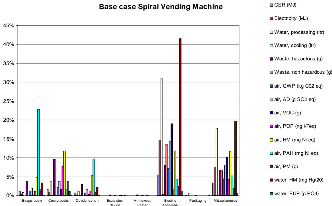
The raw materials use contributes to 90 % of the GER of the production phase. The most contributing modules are developed below.
