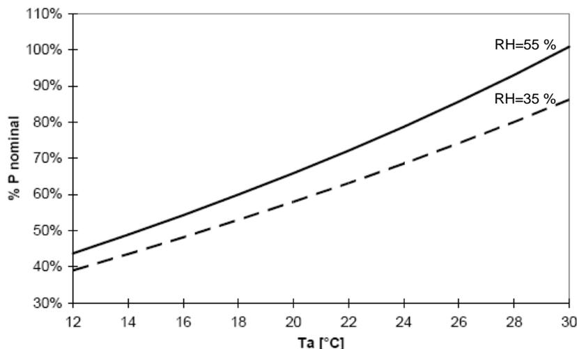
One big energy efficiency issue is the determination of the optimum set points for Ta and RH (optimal ambient conditions) taking into account considerations for the comfort of the shoppers. Simulation programs are currently under development.
