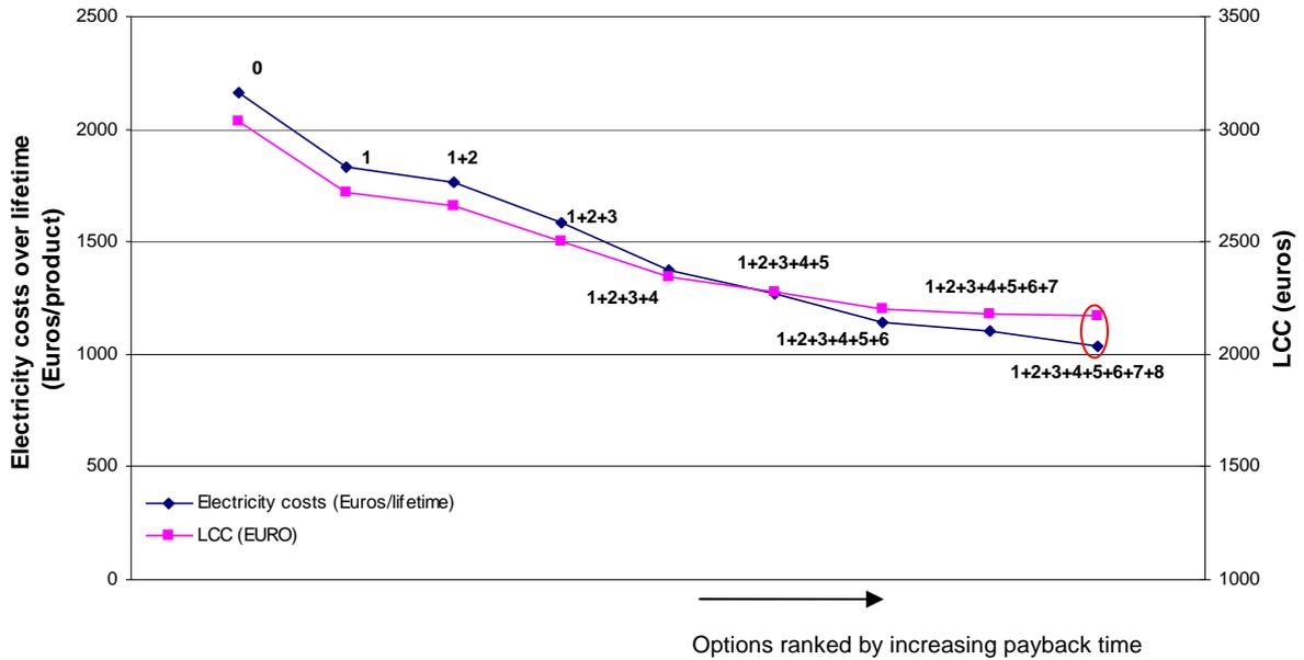
**Figure 7-52: Energy consumption during use phase versus LCC for the base case beverage cooler**
