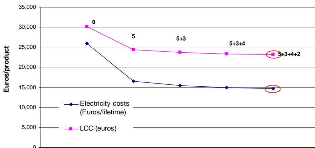
**Figure 7-43: Energy consumption during use phase versus LCC for the base case RHF4 (with glass lid)**
