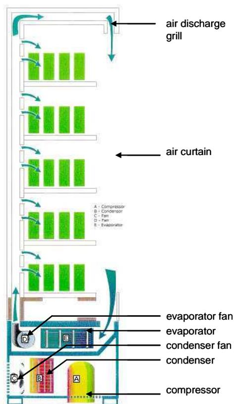
Beverage coolers (Figure 4-6) are fronted glass cabinets for displaying and selling goods, primarily canned and bottled beverages but also ice creams. The case is typically insulated with a 40 mm thick panel of blown polyurethane foam.
