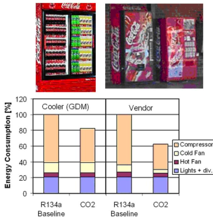
Although energy reduction by using CO<sub>2</sub> instead of R134a in cold vending machines seems to be relevant for a certain range of temperatures, few are available on the EU-27 market. Likewise, for ice cream freezers only a small number of appliances using carbon dioxide as refrigerant are put on the market. More generally, CO<sub>2</sub> based refrigeration for ice cream freezer is still a technical challenge, specifically for single stage compressors.
