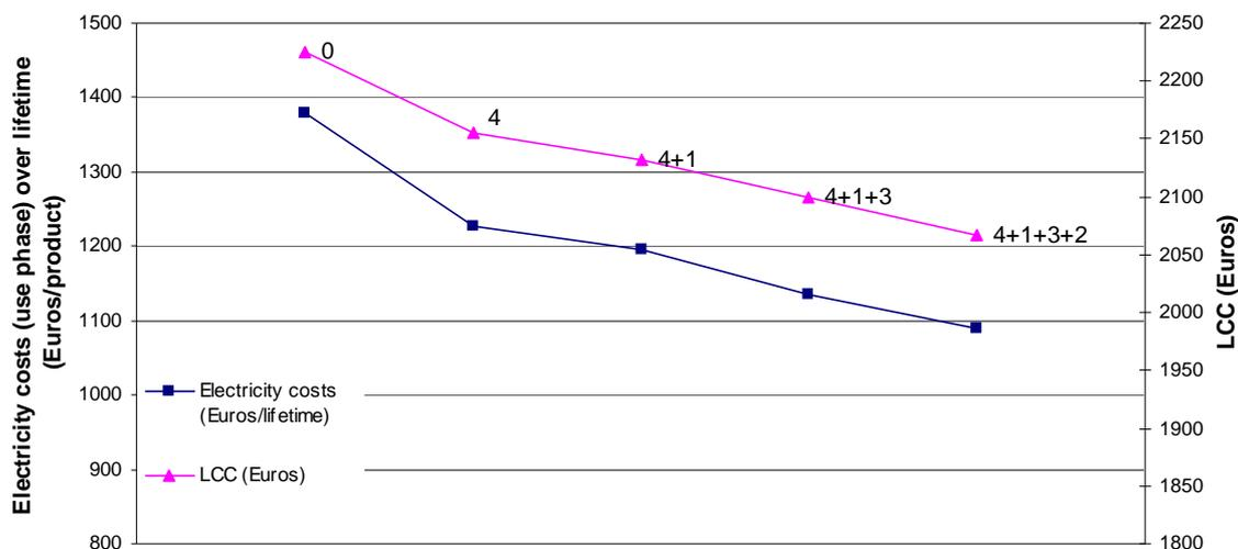
**Figure 7-67:** Electricity consumption during use phase versus LCC for the base case ice cream freezer
