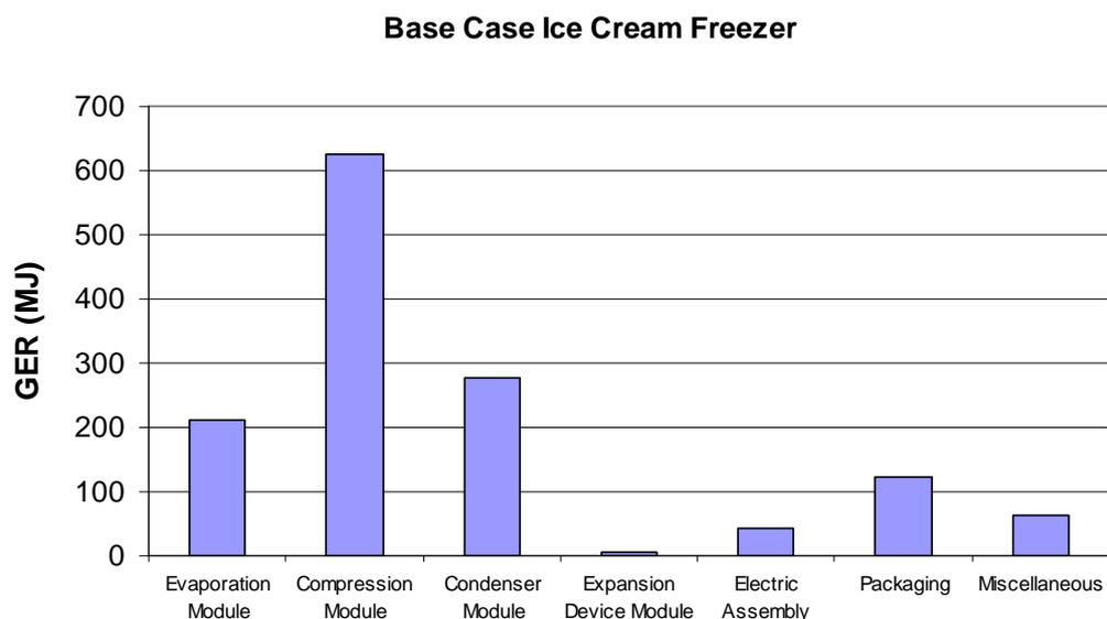
The GER during production phase is of 10,710 MJ. The housing represents over 87 % of this figure, followed by the compression module (~ 6 %), the condenser module (2.6 %) and the evaporation module (~ 2 %). As for the other cabinets
