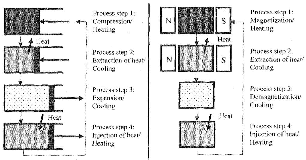
The Cambridge programme from Cambridge University develops a revolutionary magnetic refrigeration technology. Magnetic refrigeration promises a number of benefits over the vapour compression technology, including a significant reduction in energy consumption, elimination of refrigerant leakage and ease of recycling.
