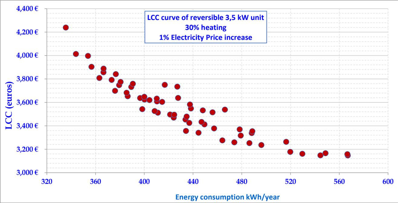
Figure 37 BC 1: 30% heating/ 1% electricity price increase
