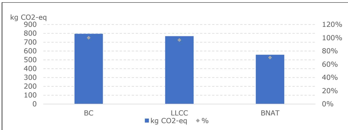
Figure 31: Emission of CO<sub>2</sub> (kg CO<sub>2</sub>-eq) of the base case, LLCC and BNAT – for BC 3 (single duct 2.6 kW – R290)
