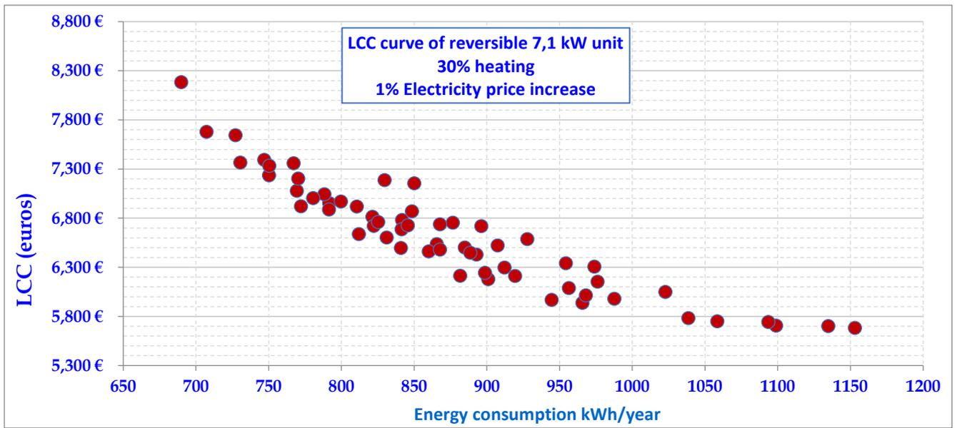
Figure 41 BC 2 : 30% heating/ 1% electricity price increase
