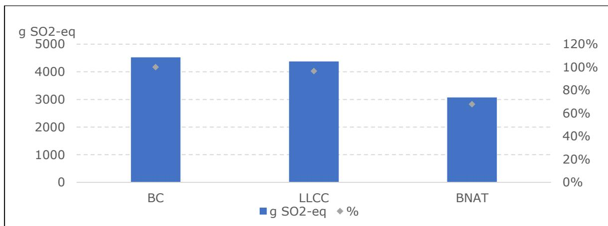
Figure 35: Emission of acidifying agents (g SO<sub>2</sub>-eq) of the base case, LLCC and BNAT – for BC 3 (single duct 2.6 kW – R1234yf)
