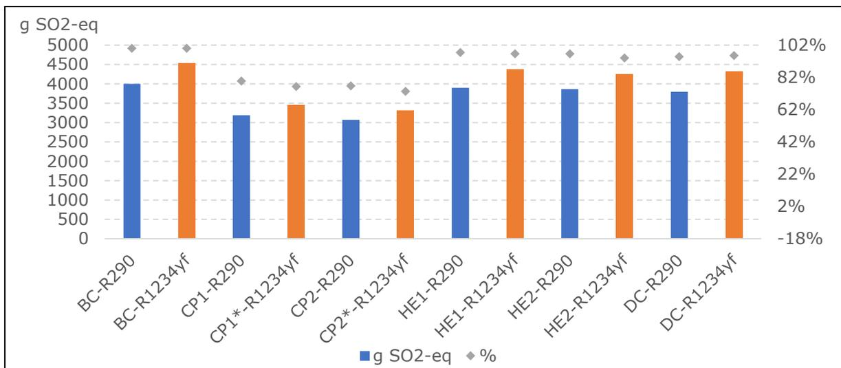
Figure 10: Emission of acidifying agents (g SO<sub>2</sub>-eq) of the base case and the different improvement options – for BC 3 (single duct 2.6 kW- R290 and R1234yf)
