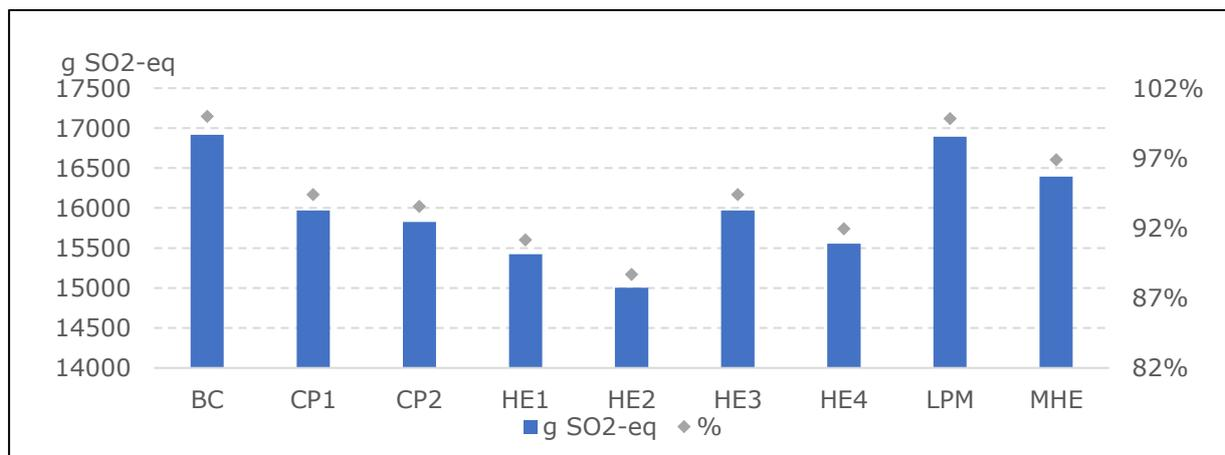
Figure 4: Emission of acidifying agents (g SO<sub>2</sub>-eq) of the base case and the different improvement options – for BC 1 (split 3.5 kW)
