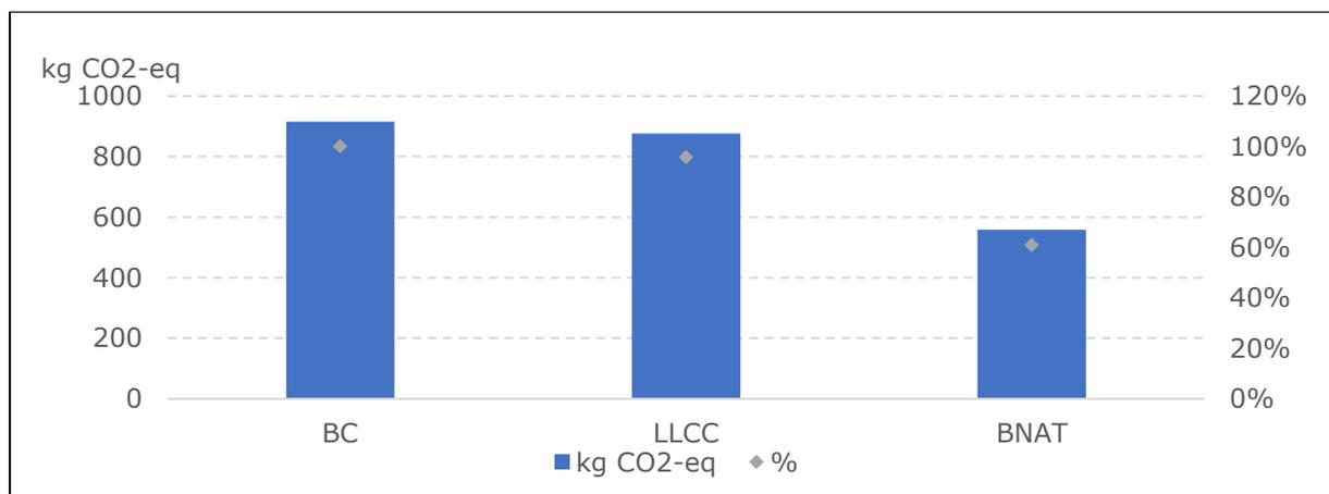
Figure 34: Emission of CO<sub>2</sub> (kg CO<sub>2</sub>-eq) of the base case, LLCC and BNAT – for BC 3 (single duct 2.6 kW – R1234yf)
