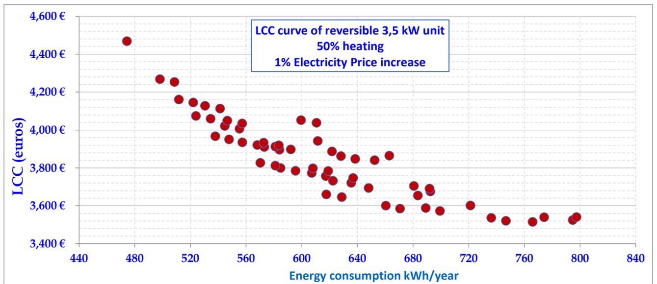
Figure 39 BC 1 : 50% heating/ 1% electricity price increase
