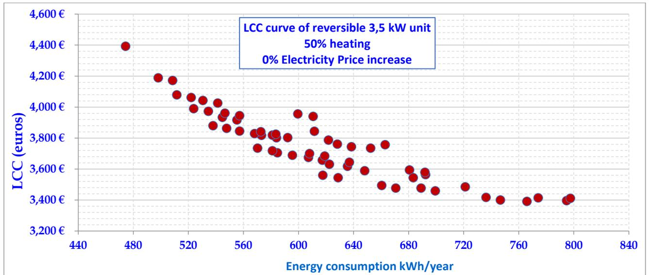
Figure 38 BC 1 : 50% heating/ 0% electricity price increase
