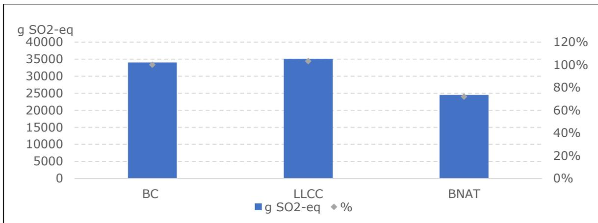
Figure 25: Emission of acidifying agents (g SO<sub>2</sub>-eq) of the base case, LLCC and BNAT – for BC 2 (split 7.1 kW)
