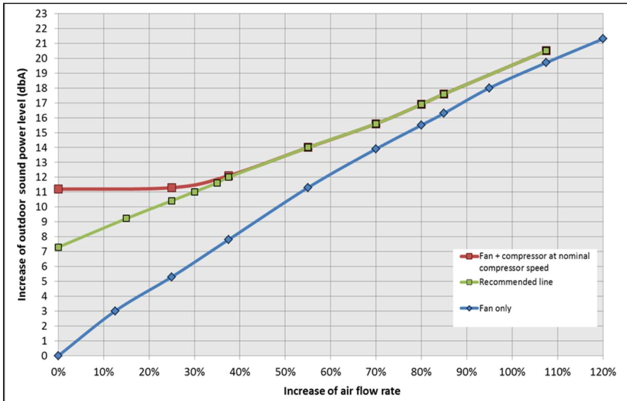
Figure 11: increase of sound power vs increase of airflow rate<sup>15</sup>
