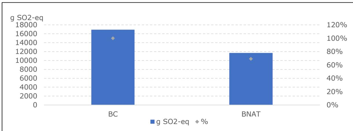
Figure 20: Emission of acidifying agents (g SO<sub>2</sub>-eq) of the base case, LLCC and BNAT – for BC 1 (split 3.5 kW)
