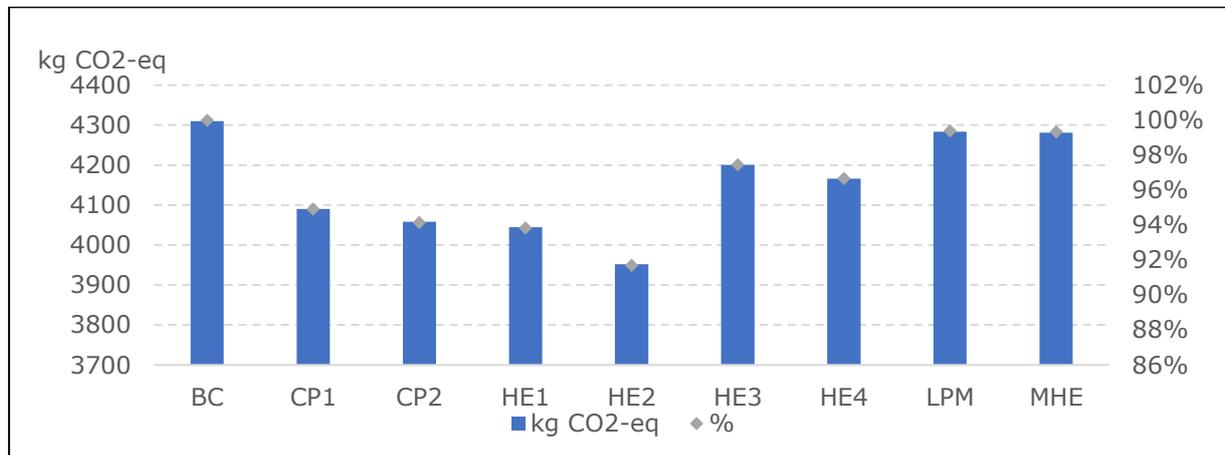
Figure 3: Emission of CO<sub>2</sub> (kg CO<sub>2</sub>-eq) of the base case and the different improvement options – for BC 1 (split 3.5 kW)
