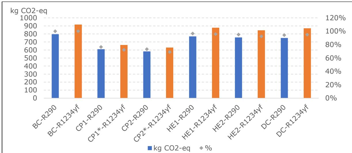
Figure 9: Emission of CO<sub>2</sub> (kg CO<sub>2</sub>-eq) of the base case and the different improvement options – for BC 3 (single duct 2.6 kW- R290 and R1234yf)
