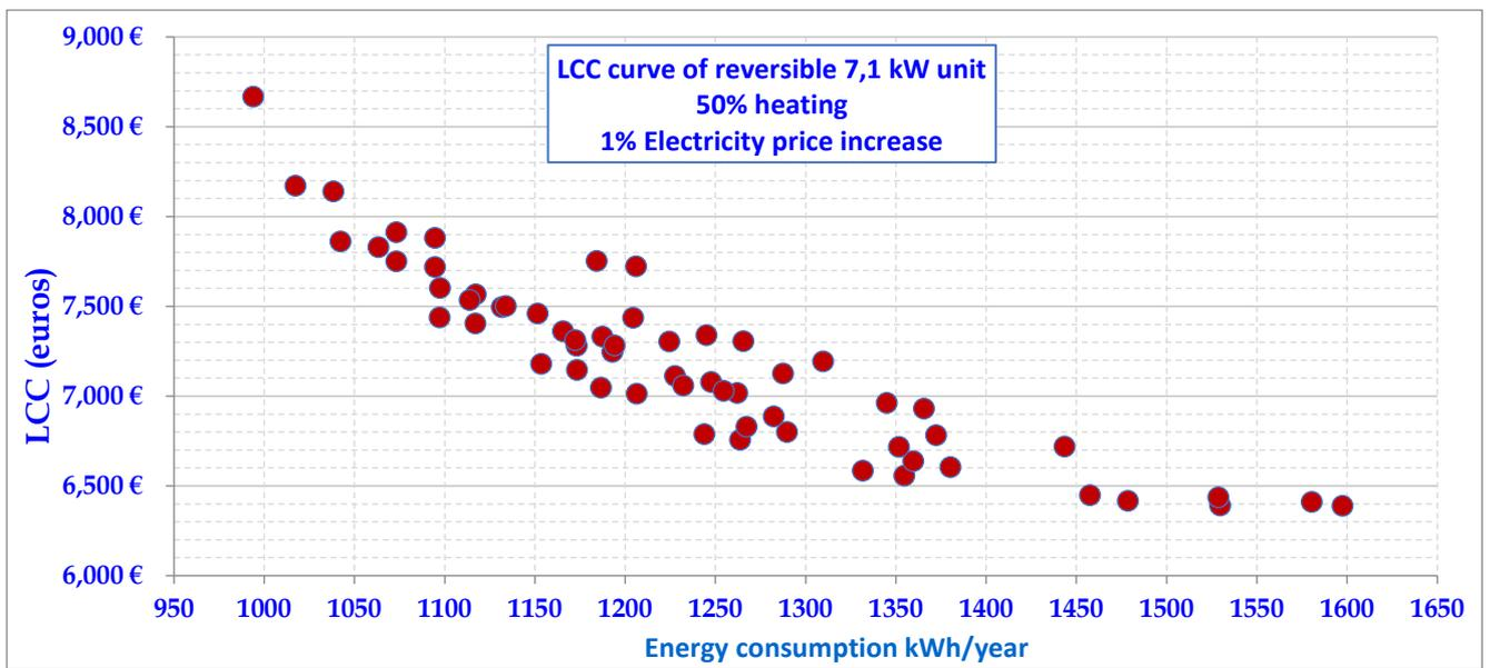
Figure 43 BC 2 : 50% heating/ 1% electricity price increase
