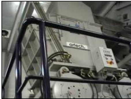
Figure 123: Granulator (to shred elements in small pieces)
