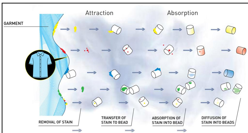
Figure 9 Polymer cleaning
