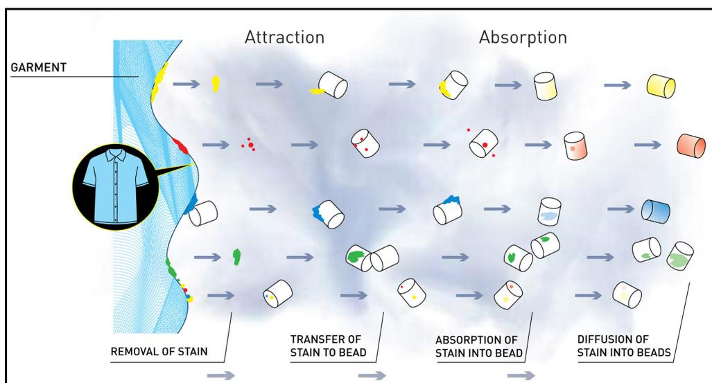
Figure 9 Polymer cleaning
