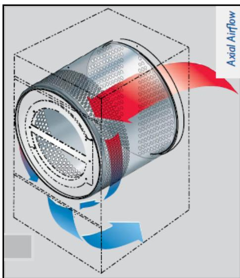
Figure 16 Axial airflow
