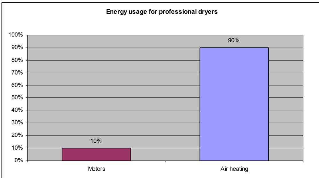
Figure 11 Energy use for a typical professional air dryer cycle<sup>27</sup>
