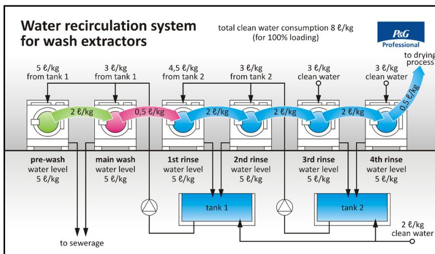
Figure 5 Various washer extractors in a water recirculation system <sup>10</sup>
