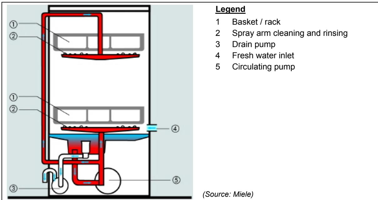
Figure 1 Construction of an undercounter water-change dishwasher (category 1)
