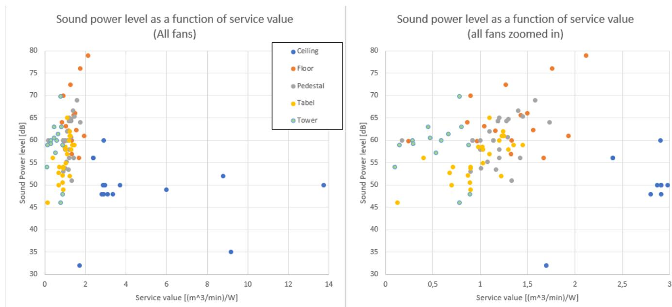
Figure 14: Sound power level as a function of the service value for the data collected in this IA study and in the review study. In the right diagram is zoomed in on the lower service values. The solid lines are the labelling classes for the sound power proposed in the working document.
