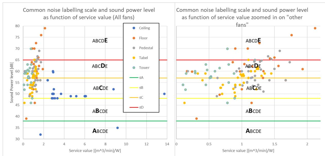
Figure 17: Revised proposal for a common sound power labelling scale for all comfort fans independent of the diameter, the graph at the right side is zoomed in on the "other fans".
