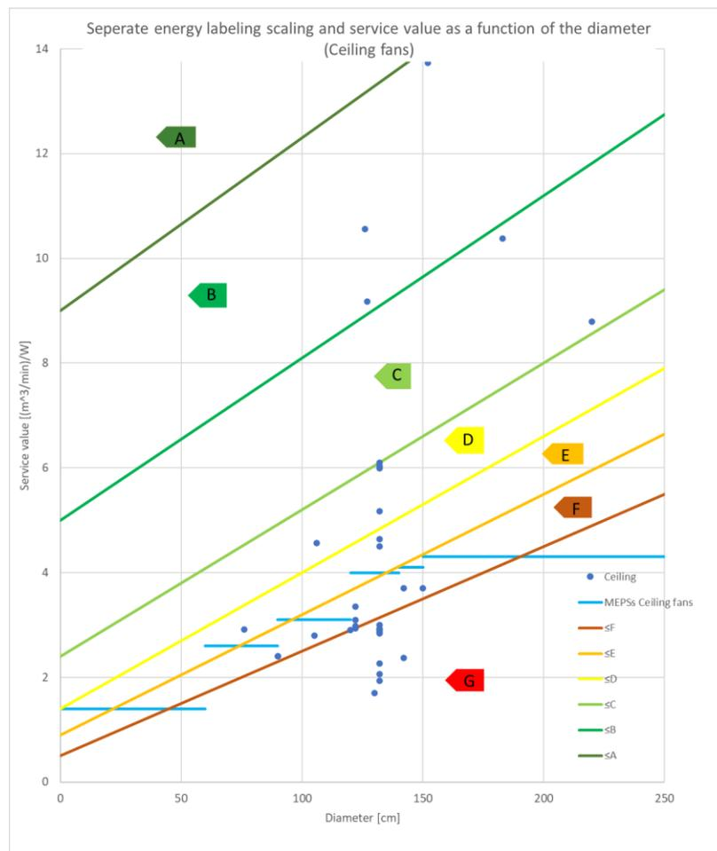
Figure 11: Suggestion for separate energy labelling scale and MEPS for ceiling fans, dependent on the diameter.
