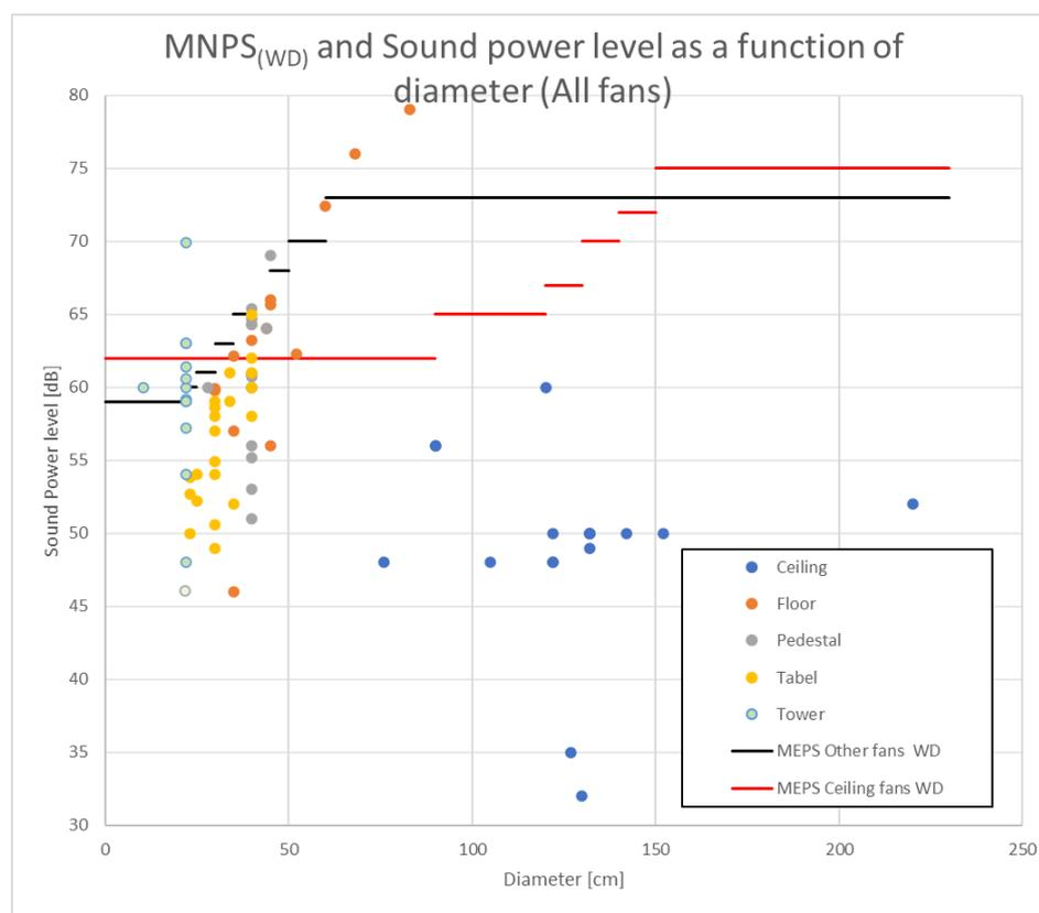
Figure 13: Sound power level as function of the diameter for the data collected in this study and in the review study. Solid lines are the MNPS proposed in the working document.
