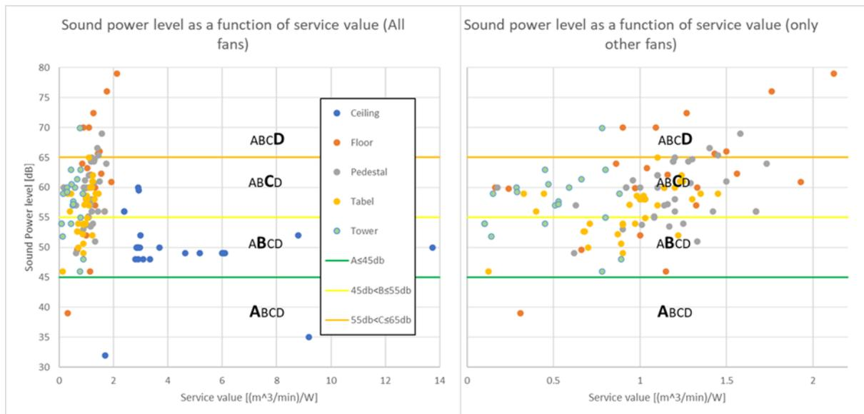
Figure 16 Sound power level as a function of the service value for the data collected for this report and in the review study. In the right diagram is zoomed in on the lower service values and only other fans are included. The solid lines are the labelling classes for the sound power propose.
