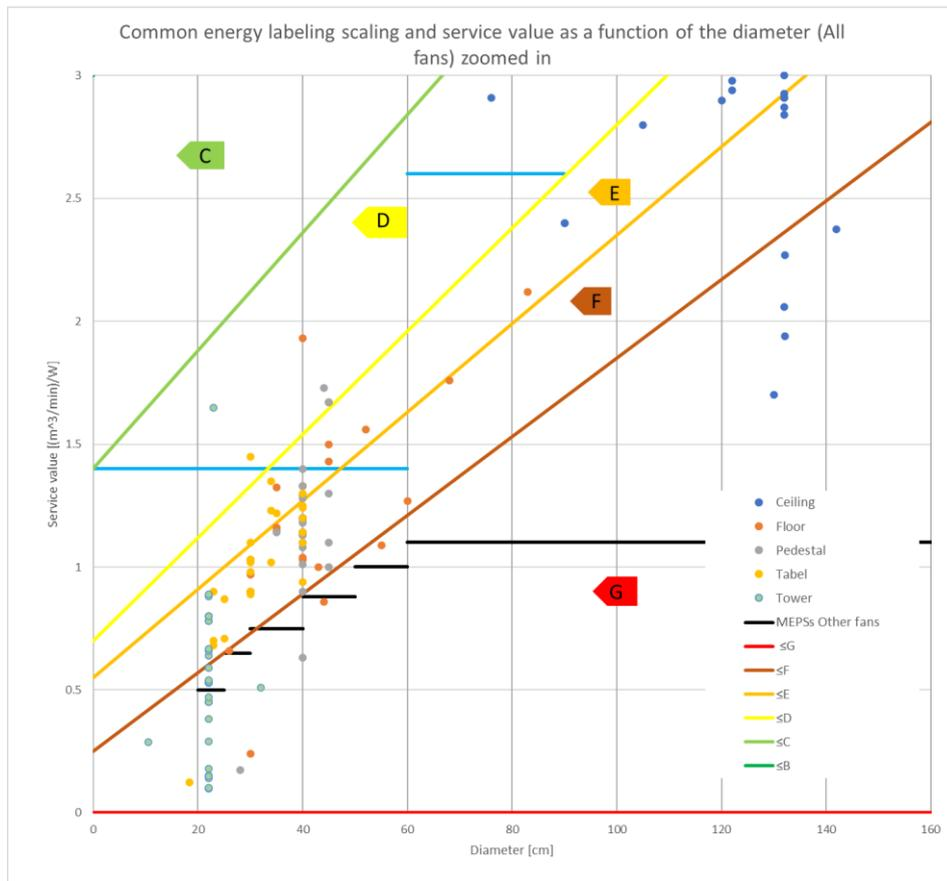
Figure 9: Suggestion for a common energy label. Thresholds for energy labelling class as a function of the diameter, uneven difference between the thresholds, same energy labelling scale for all fans, zoomed in to analyse other fans.
