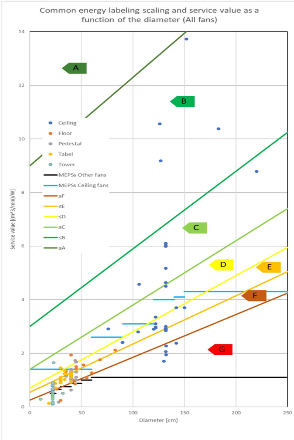
Figure 8: Suggestion for a common energy label. Thresholds for energy labelling class as a function of the diameter, uneven difference between the thresholds, same energy labelling scale for all fans
