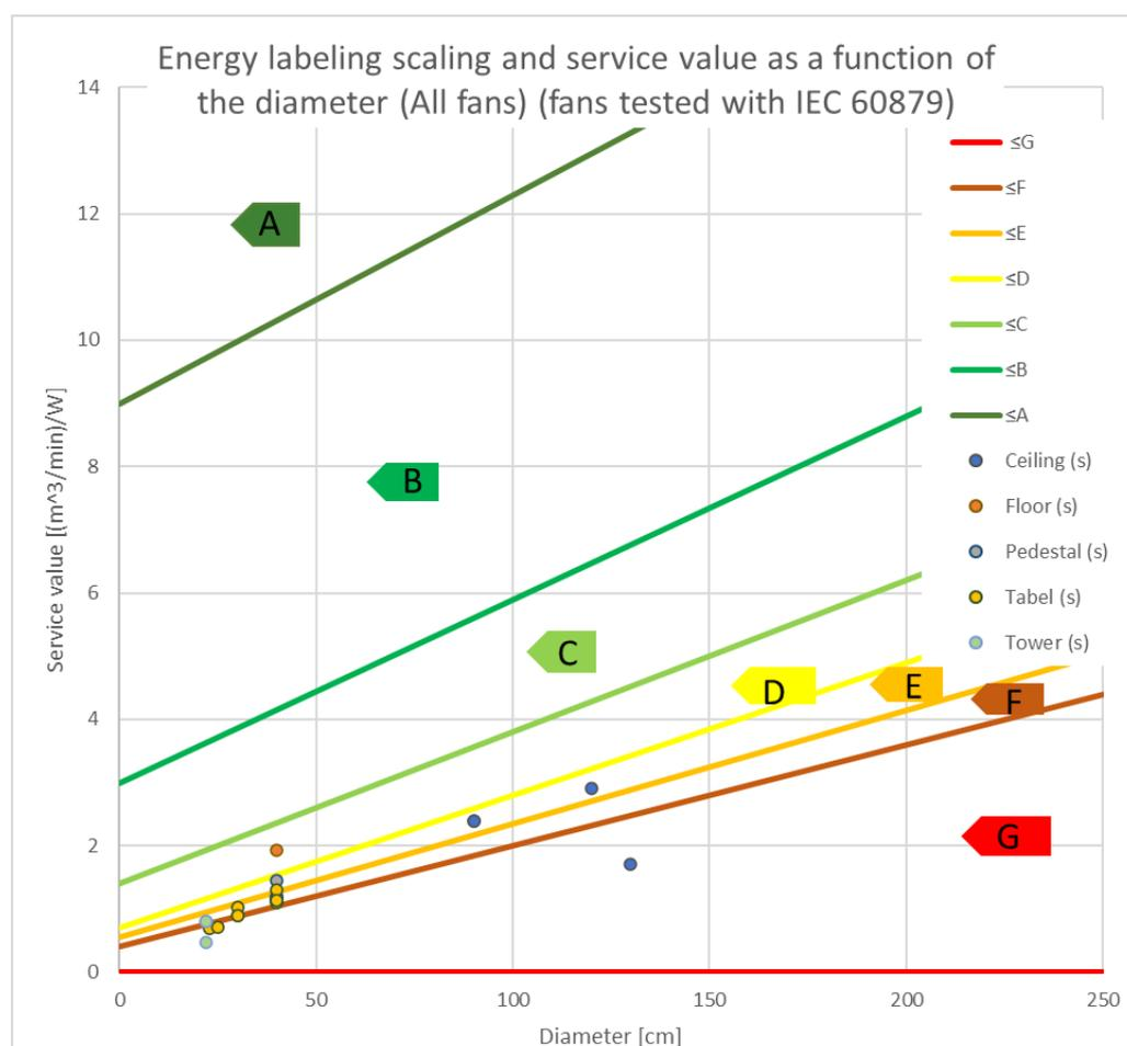
Figure 19: Distribution of comfort fans tested according to IEC 60879<sup>29</sup>
