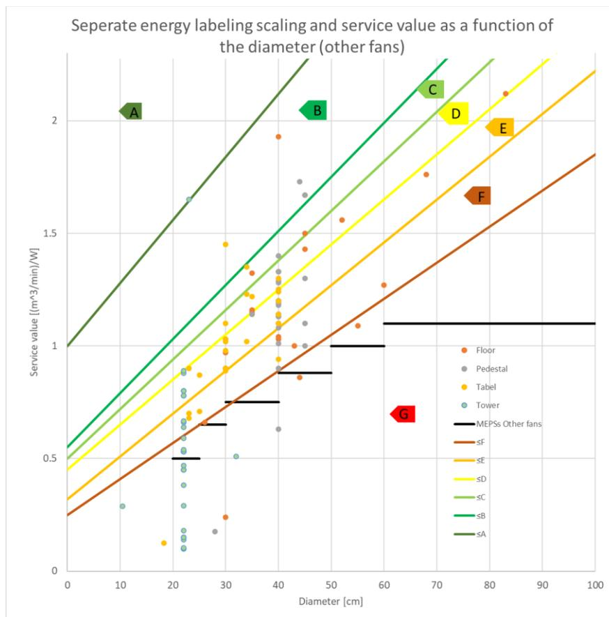
Figure 12: Suggestion for separate energy labelling scale and MEPS for “other fans”, dependent on the diameter.
