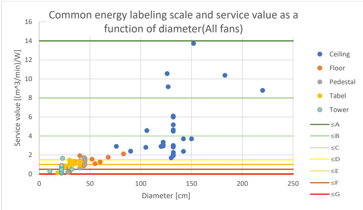
Figure 6: Suggestion for common energy label scale set independent of diameter and with uneven distribution of classes
