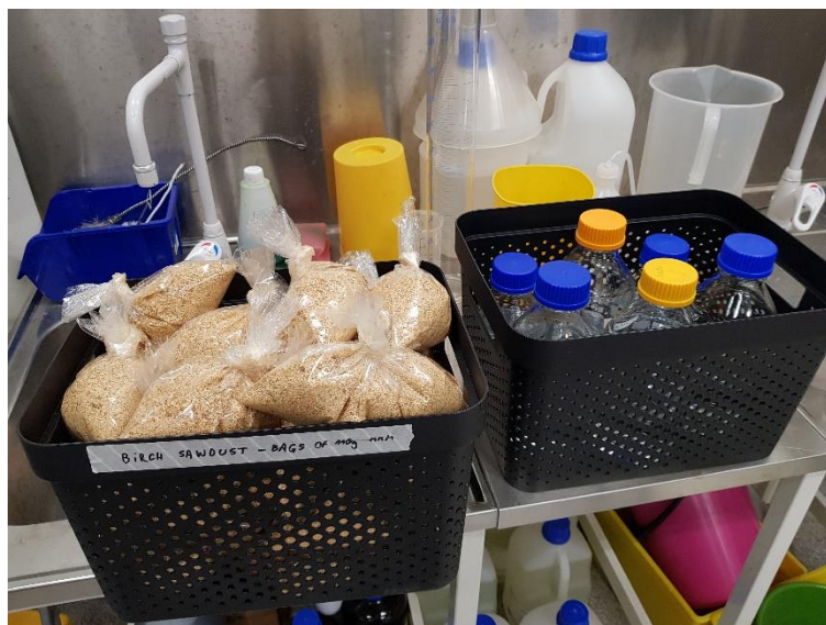
Figure 1: Birch sawdust and solvent solutions before organosolv pretreatment
