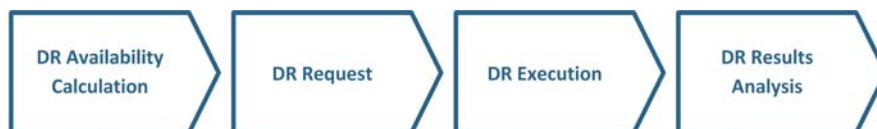
Figure 25: The centralized DR execution process.
